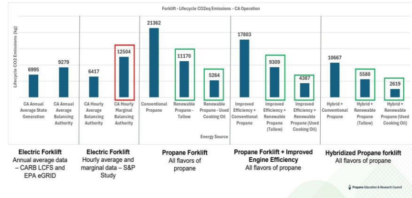
Figure 38 California 365-day forklift results: electric forklift lifecycle CO 2 e under annual-average, hourly-average, and marginal grid data, versus propane in all flavors plus improved-efficiency and hybridized variants.
