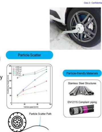
Figure 69 CFD-optimized collection nozzle: single front-wheel hub-mounted unit, antistatic materials, isokinetic sampling, 0.04 m 2 inlet, 20 mm above ground and behind the tyre, ~230 m 3 /h flow.
