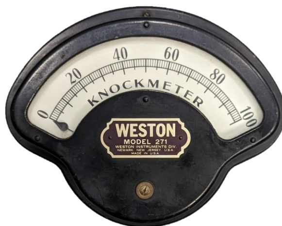
Figure 8. Standard knockmeter for the CFR Engine knock intensity characterization in RON and MON tests.
