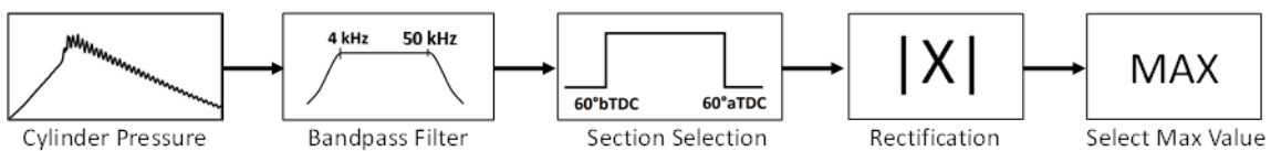
Figure 14. Calculation procedure for the maximum amplitude of pressure oscillations (MAPO)
