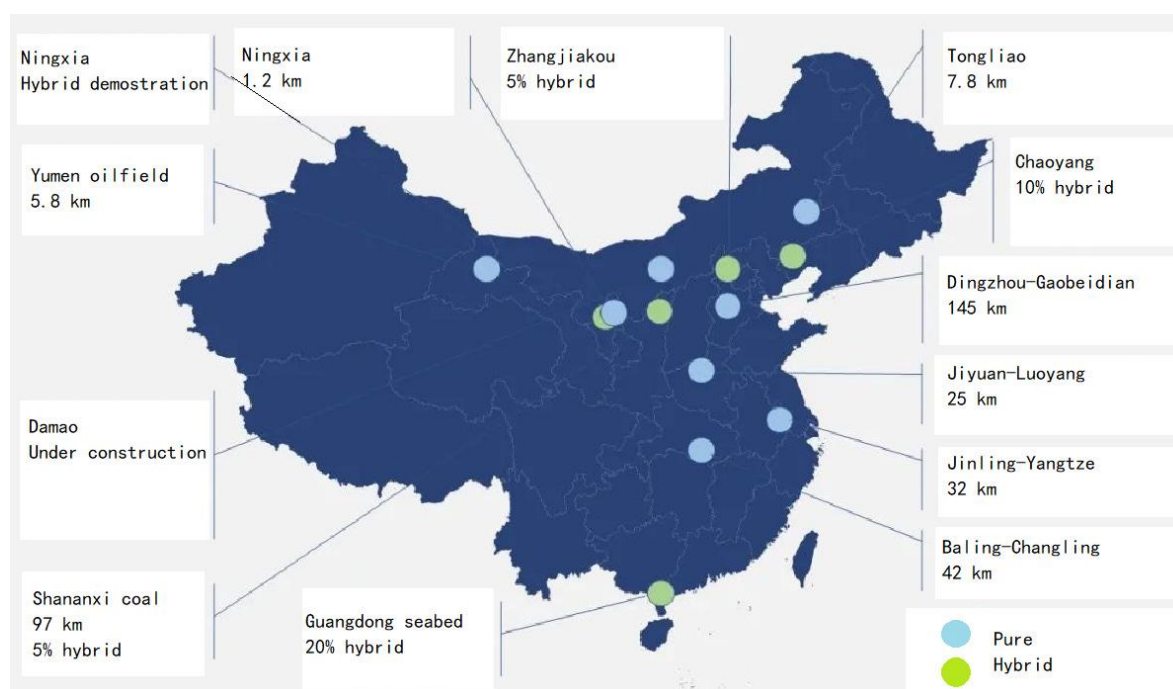
Figure 9-81. Operational Hydrogen pipeline infrastructure in China 380 .
