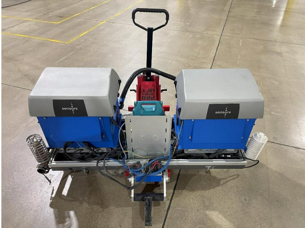
**Figure 3-6: PEMS Setup of Hydraulic Jack**
