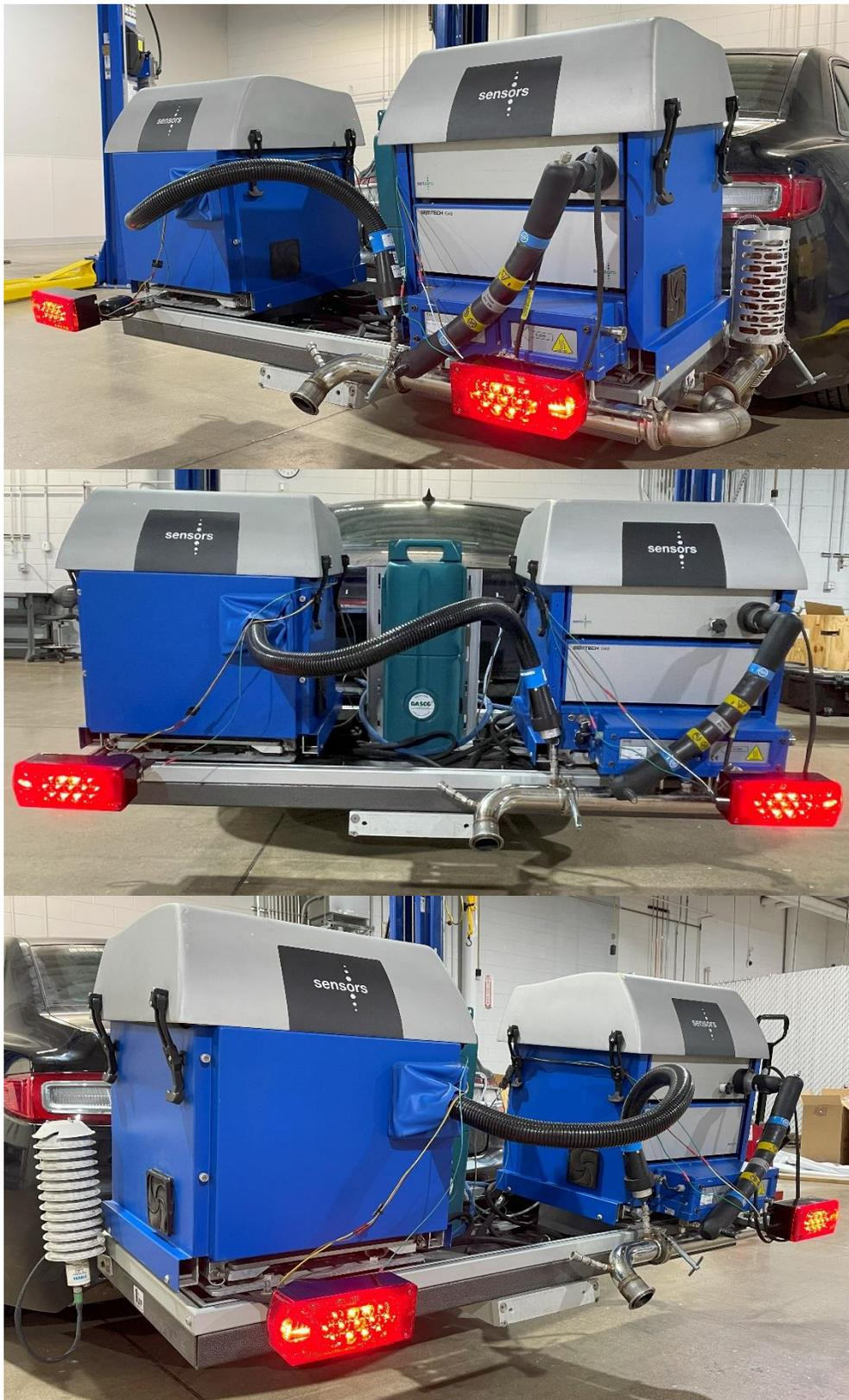
Figure 3-7: PEMS Setup Mounted on Test Vehicle
