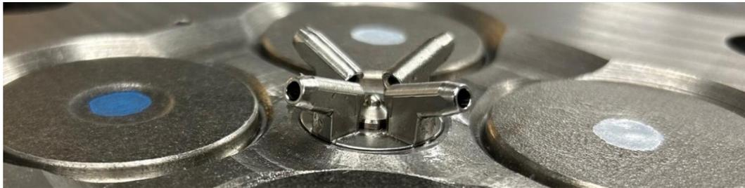
Figure 1. 4H DFI installed on a John Deere multi-cylinder diesel engine.
