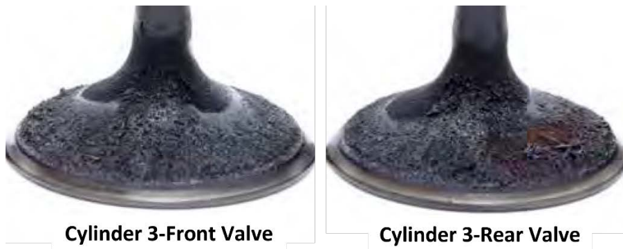
Figure 11 - Intake Valve Photos from GMIVD91-011 (Fuel B + 1 x LAC Detergent 1)
