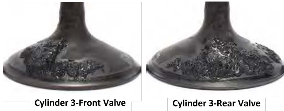
Figure 12 - Intake Valve Photos from GMLIVD91-010 (Fuel B + 2.5 x LAC Detergent 1)
