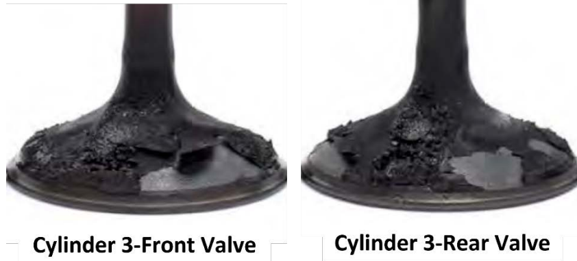
Figure 10 - Intake Valve Photos from GMIVD91-009 (Unadditized Fuel B)
