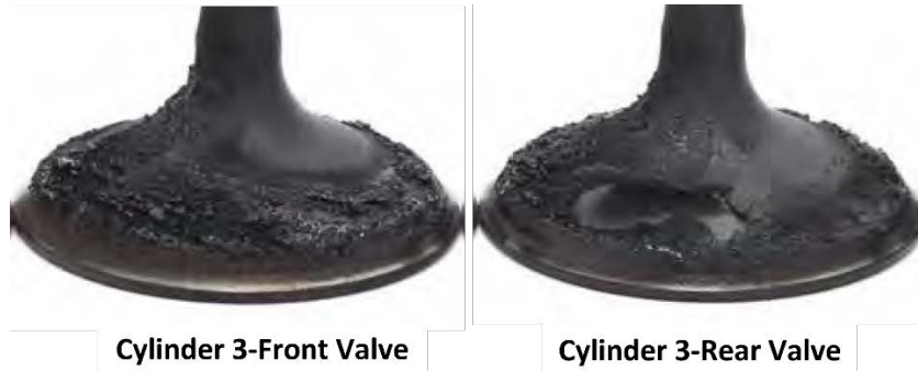
Figure 13 - Intake Valve Photos from GMLIVD91-010 (Unadditized Fuel 3 @ 50 hours)
