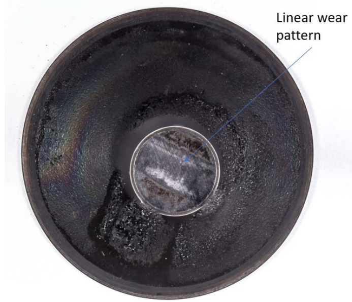
Figure 20 - Wear Pattern on Intake Valve Tip
