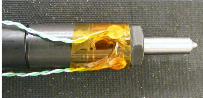
Figure 2: Photograph Showing Location of Surface Mount Thermocouple on Injector
