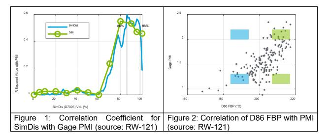
In addition, back-end distillation has come under scrutiny as a possible predictor of PMI. For example, a limit of either 425°F or 450°F (218°C or 232°C) have been discussed for SimDis T99 cutoff in recent regulatory rulemaking proposals. Therefore, there is interest in deconvoluting back-end distillation (FBP) from overall distillation, as well as from PMI, and determining if any are independently and universally correlated with vehicle tailpipe emissions.
