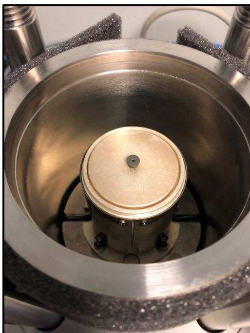
Figure C12: Inside of the HPDSC cell, with the outer silver lid installed.
