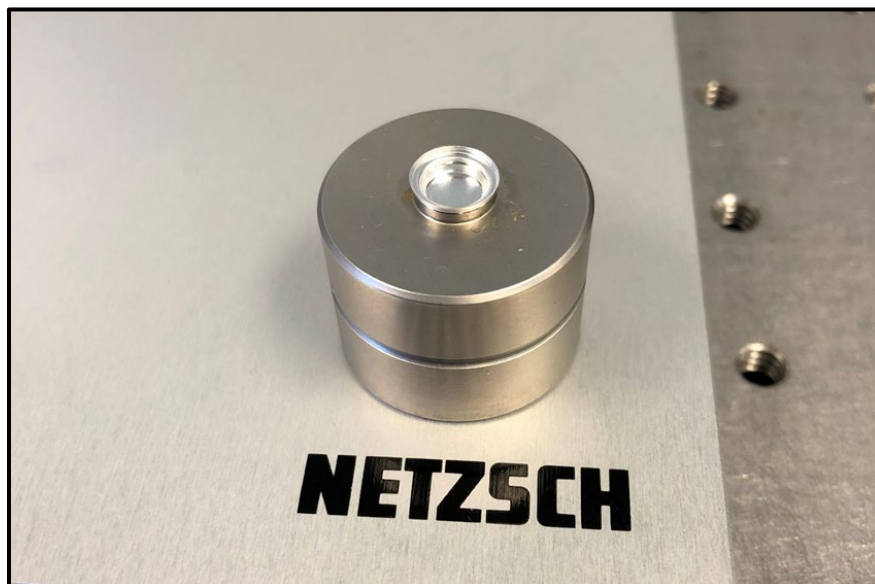
Figure C1: DSC pan resting on the crimping press lower die.
