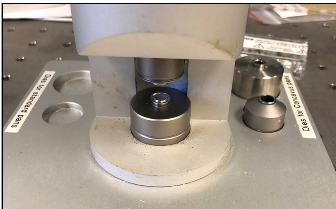
Figure C8: DSC pan/lid after crimping
