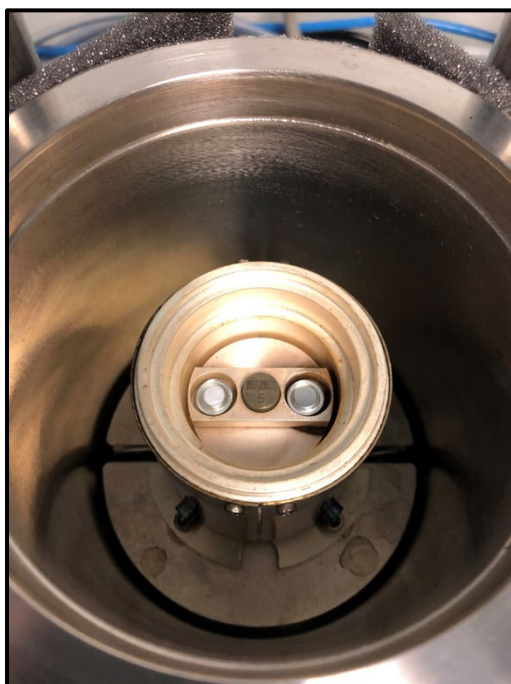
Figure C10: Inside of the HPDSC cell, with a JF sample on the sample side of the HPDSC cell.
