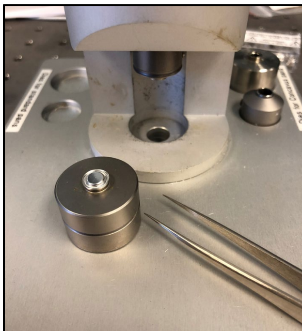
Figure C6: Laser-drilled lid placed on DSC pan.
