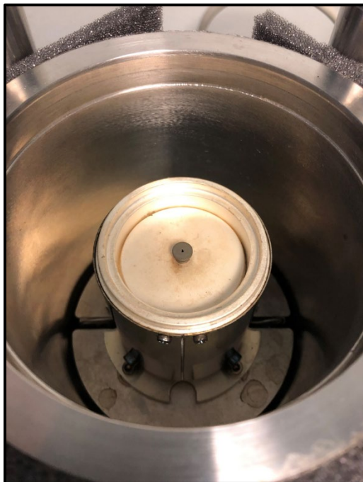
Figure C11: Inside of the HPDSC cell, with the inner silver lid installed.
