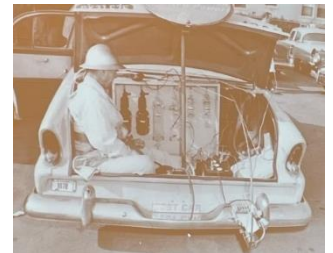
Picture of early PEMS measurement – 1955 Los Angeles Riverbed study Emission rates were given in "lbs/hour" – we have come a long way.
