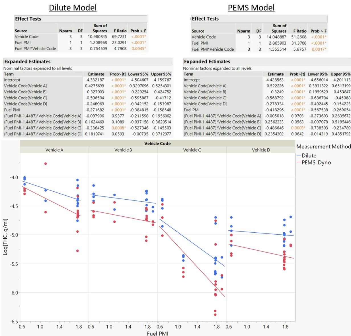
**FIGURE 78. PLOT OF LN (THC) VS. FUEL PMI BY METHOD**
