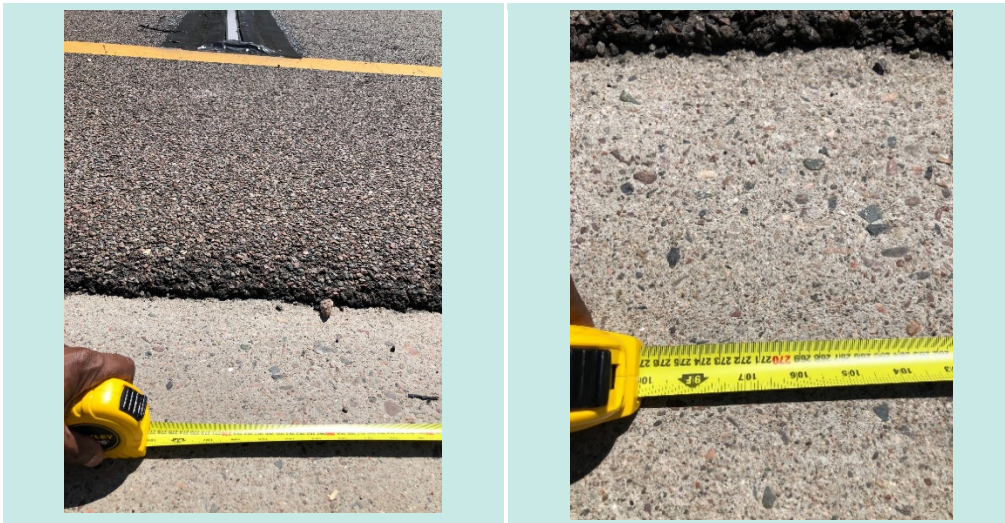
Figure 4: Initial Distance from HEAT Reflector Strip (April 12, 2021) – 9 feet
