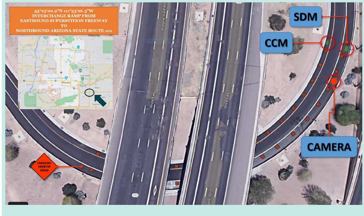
Figure 1: Unattended Model RSD5000 On-Road Deployment
