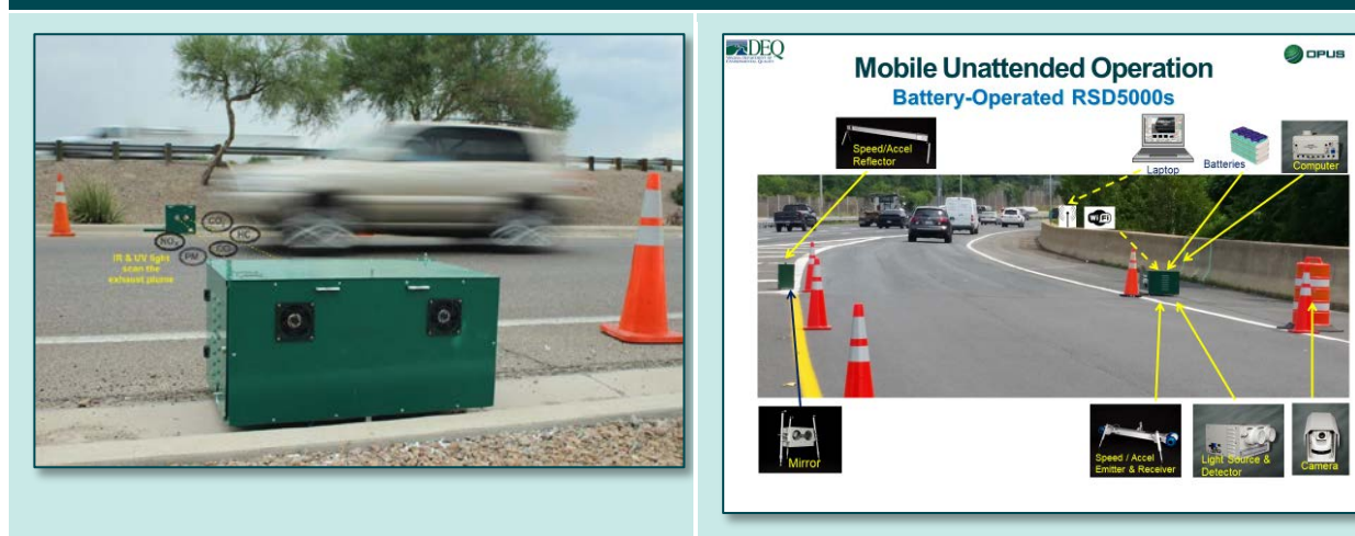
Figure 2: Unattended RSD5000 On-Road Deployment
