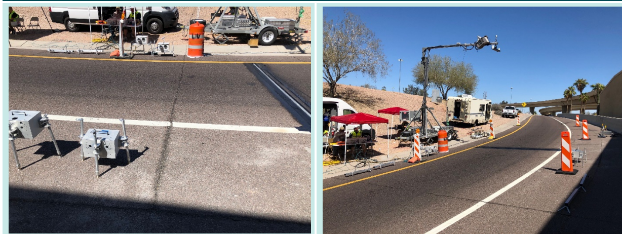
Figure 3: Two Manned RSD5000 Deployments at Different Heights
