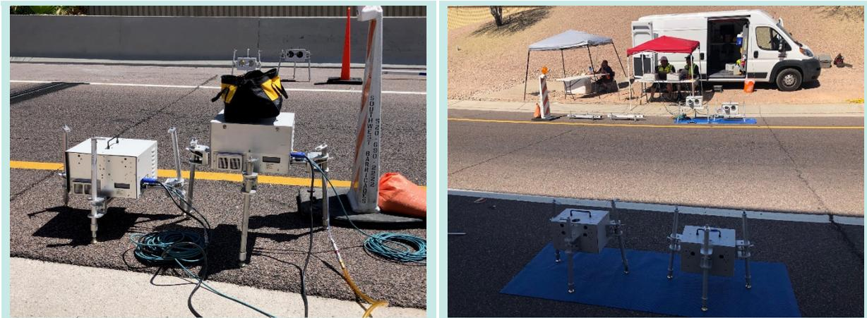
Opus moved further away (18-23ft) from the HEAT set-up starting Tuesday afternoon (April 13) and on subsequent days, but still experienced above average alignment alarms, causing recalibrations and audits. An example of a unladen truck passing over the HEAT reflector, falling back to the pavement and causing vibration was captured on video. A slow-motion and normal speed video can be found in the following DropBox folder:
