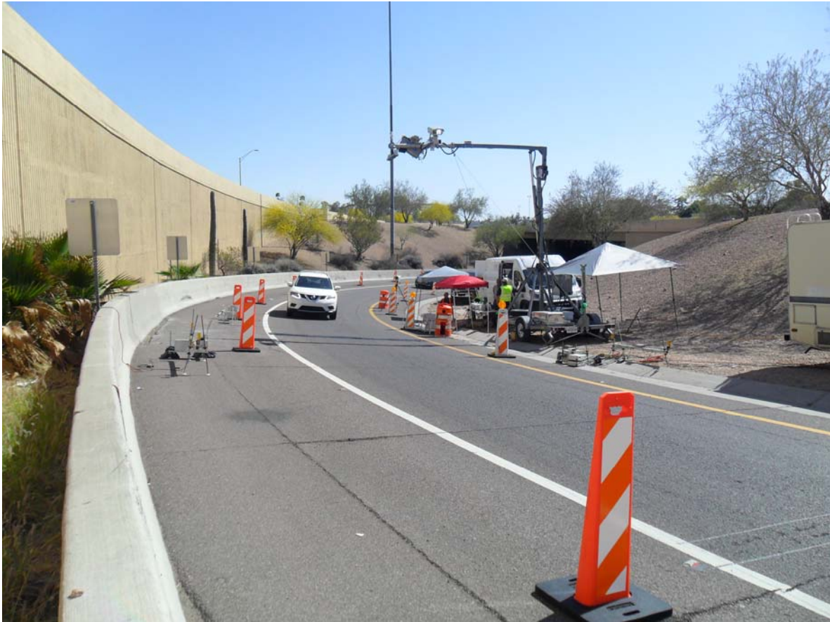
Figure 2. A photograph looking southwest at the interchange ramp from eastbound U.S. 60 to northbound SH 101 monitoring site and the remote sensing setup. The FEAT instrument is the closest to the camera in this picture followed by the HEAT and Opus instruments.
