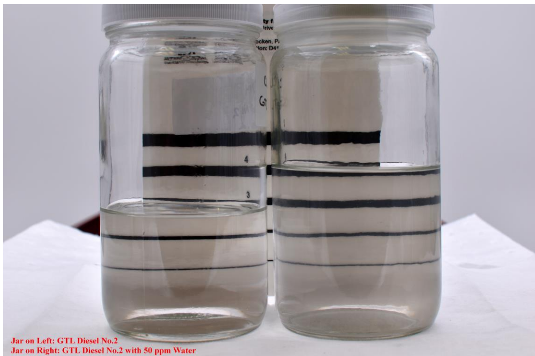
Figure 1. Representative test fuel sample with and without addition of water
