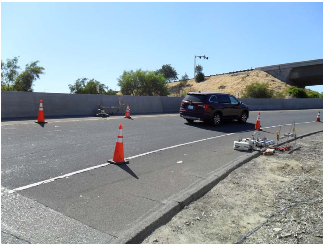
Figure 2. The Fresno monitoring site in 2021 showing the monitoring vehicle and the remote sensing detectors and speed and acceleration bars.
