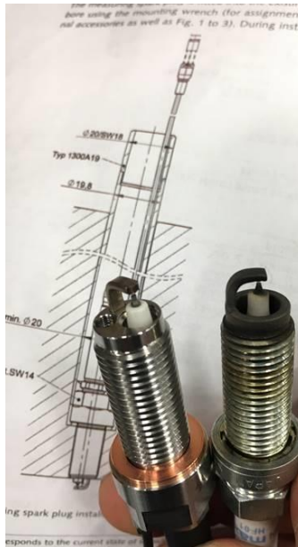
Figure 2. Spark Plug Sensor (left) Original Mazda Spark Plug (Right)
