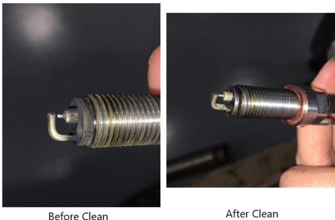
Figure 20. Spark plug inspection following C0 TR2338A Testing
