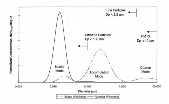
Figure 2-1. Definition of the modes and size ranges of hypothetical PM number and mass size distributions (Source: adapted from *J. Aerosol Sci.*, **29**, Kittelson, D.B., "Engine and nanoparticles: a review", 575-588, Copyright (1998), with permission from Elsevier).
