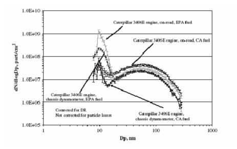
Figure 2-2. Particle number concentration distributions for diesel engines with EPA and California fuels sampled on-road and in the laboratory (Source: Reprinted from *J. Aerosol Sci.*, **37**, Kittelson, D.B., W.F. Watts and J.P. Johnson, "On-road and laboratory evaluation of combustion aerosols – Part 1: Summary of diesel engine results", 913-930, Copyright (2006), with permission from Elsevier).
