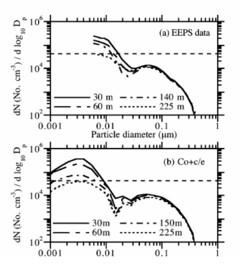
Figure 3-2. Comparison of (a) measured and (b) modeled particle number concentrations at different distances from a roadway (Source: Reprinted with permission from *Environ. Sci. Technol.*, **39**, Jacobson, M.Z., D.B. Kittelson and W.F. Watts, "Enhanced coagulation due to evaporation and its effect on nanoparticle evolution", 9486-9492. Copyright (2005) American Chemical Society).
