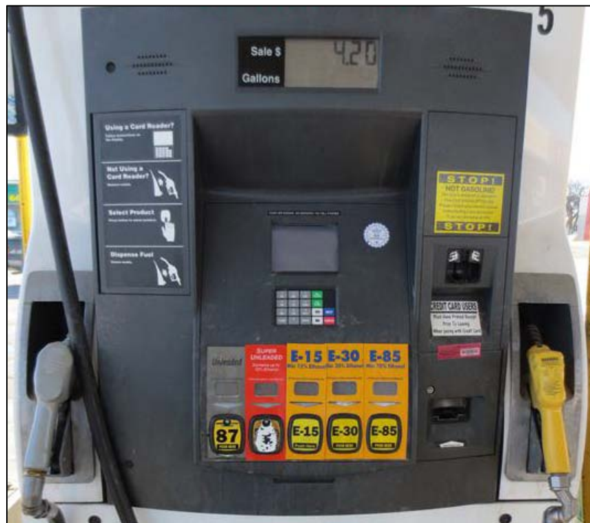
Figure 6. Station #17 offered E15 from same nozzle as higher ethanol blends
