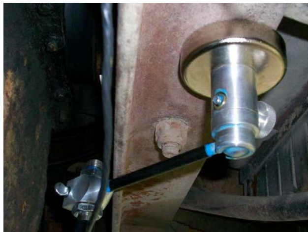
Figure 3.9-1 Optical Sensor on a Bracket With a Magnetic Base
