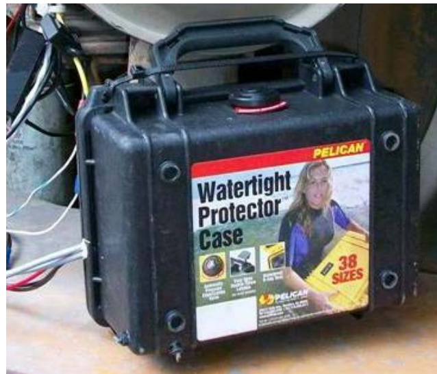
Figure 7.4-1 Pelican Case Housing a Corsa Datalogger
