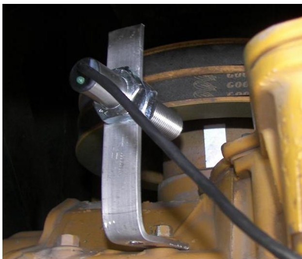
Figure 3.9-2 Optical Sensor on an Aluminum Bracket
