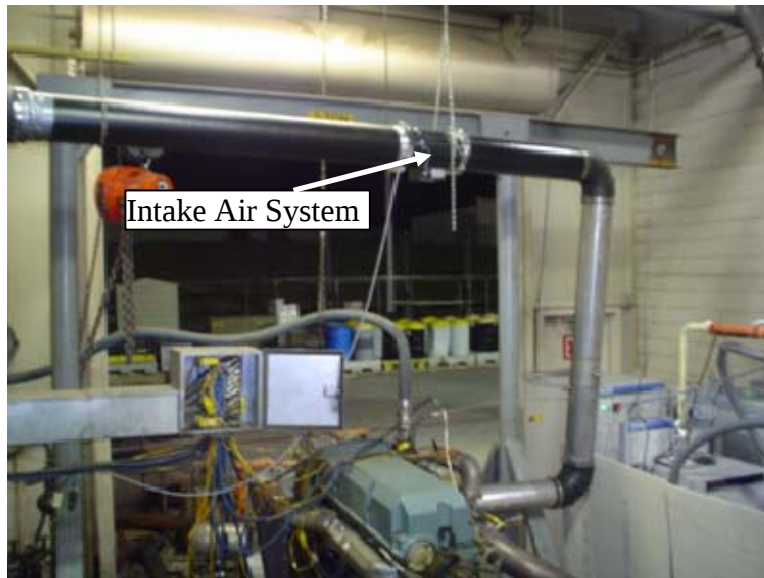
FIGURE 4. INTAKE AIR FLOW MEASUREMENT SYSTEM MOUNTED ON ENGINE INTAKE
