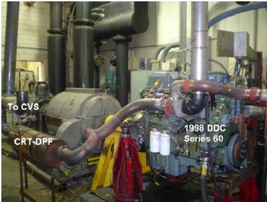
FIGURE 1. ENGINE AND EXHAUST CONFIGURATION WITHOUT A BYPASS
