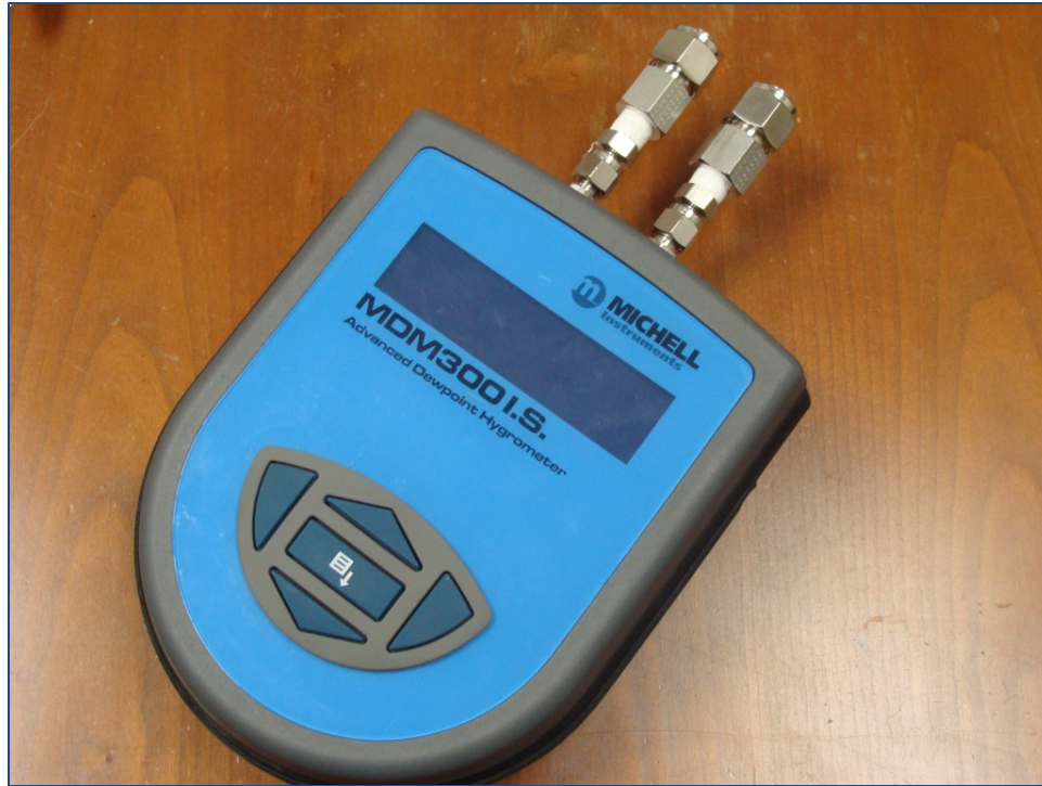
Figure 3.1. Michell MDM300-IS Portable Hygrometer Used in This Research
