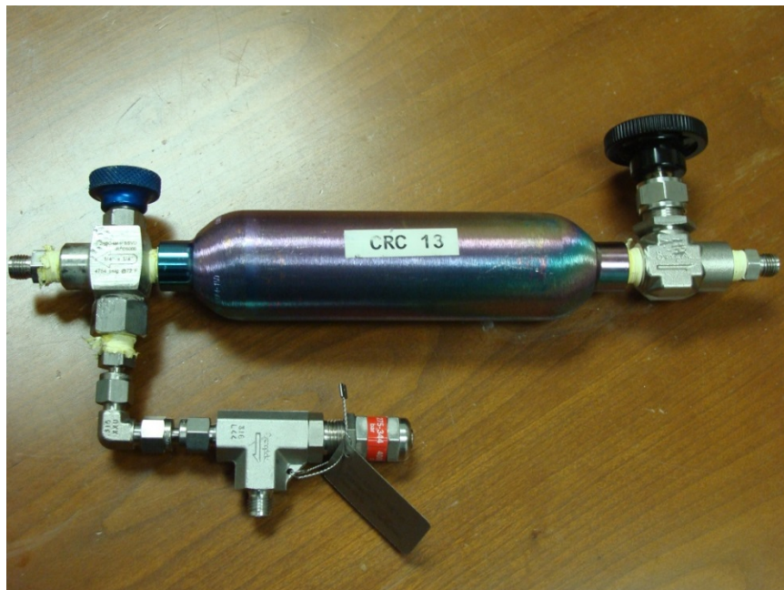
Figure 3.6. Final Configuration of Sample Cylinders Used for CNG Collection
