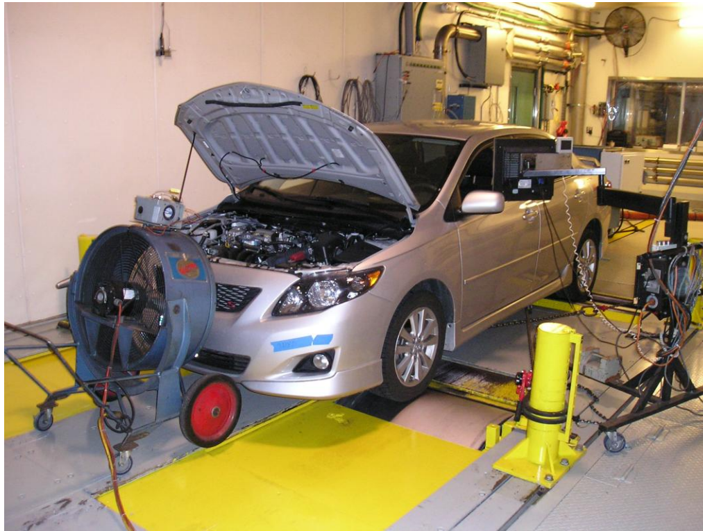
Figure 4. Corolla Tested on 48" Burke Porter Dynamometer, at SGS Emissions Laboratory
