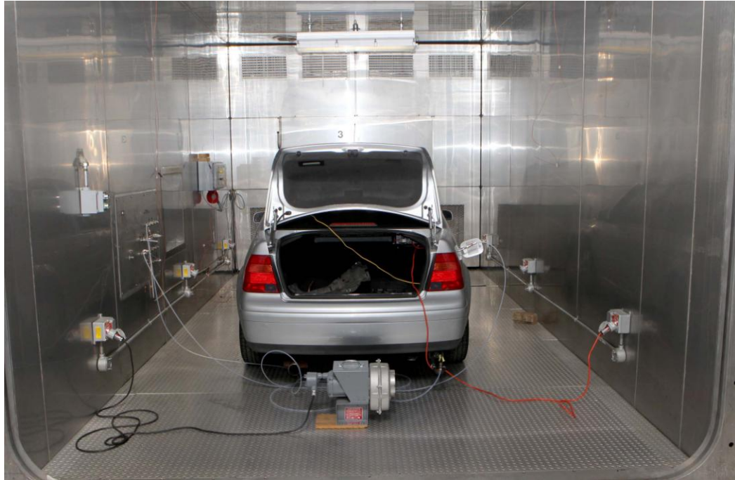
Figure 5. Jetta Loaded in the Chrysler CPG SHED
