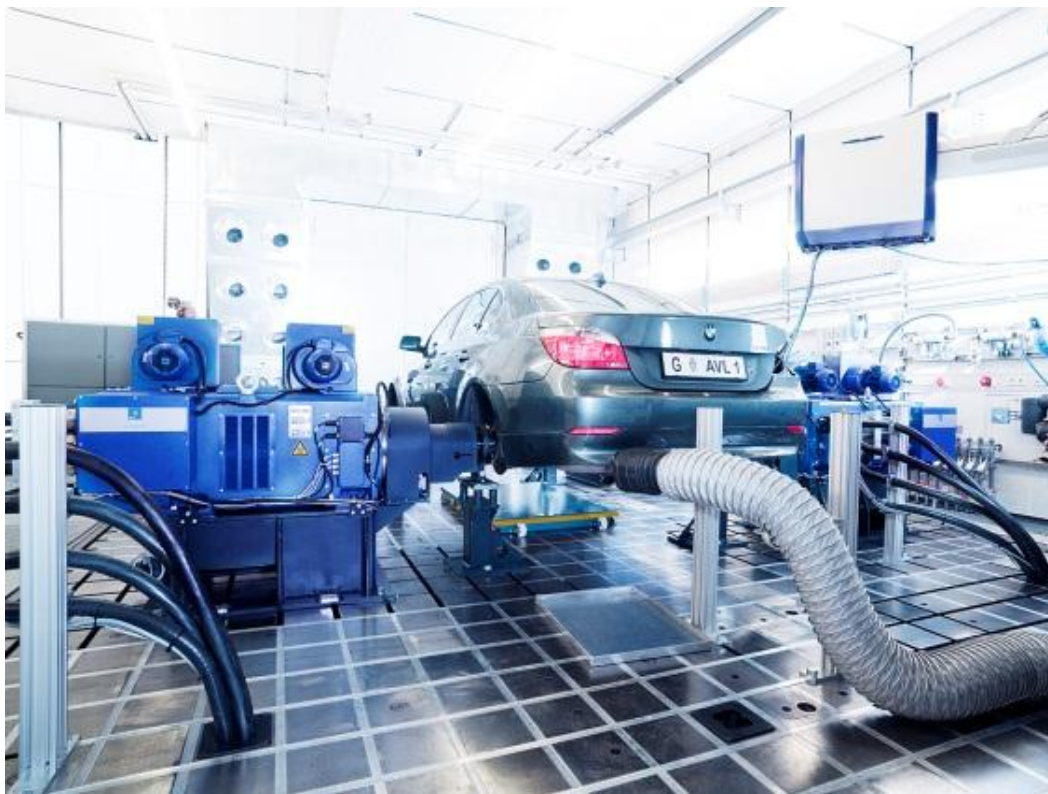
Figure 15 Typical installation on to powertrain testbed for vehicle testing
