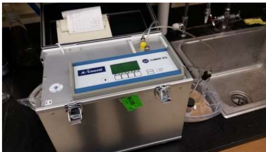
Figure 12. Photo of Seta Analytics SA1000 automatic particle counter (APC).
