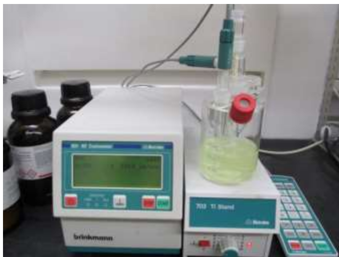
Figure 7. Metrohm Model 831 Karl Fischer Coulometer in DRI laboratory
