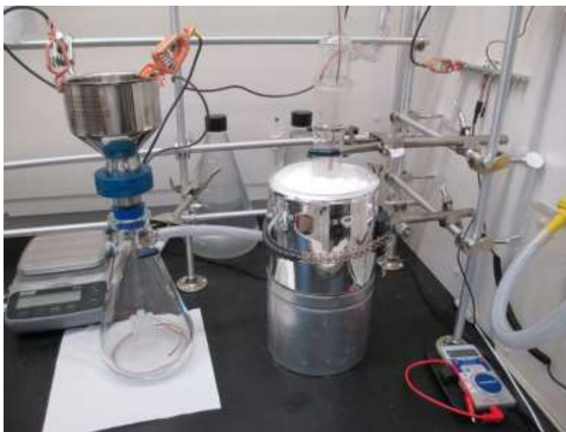
Figure 9. Fuel filtration apparatus installed in laboratory hood
