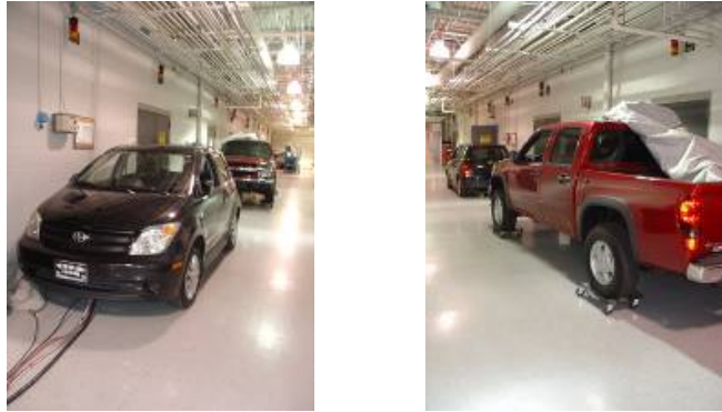
Figure D.5.1.2: Umbilical Cord Vehicle to Engine Setup
