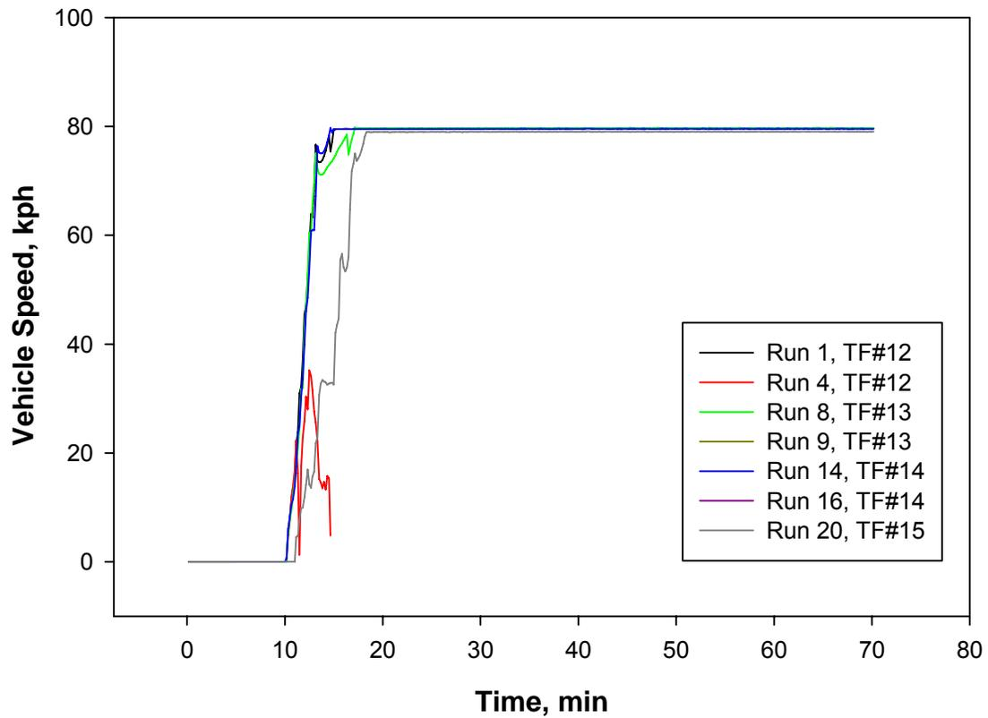
Figure 22. Vehicle speed traces for fuels tested in Truck D2.
