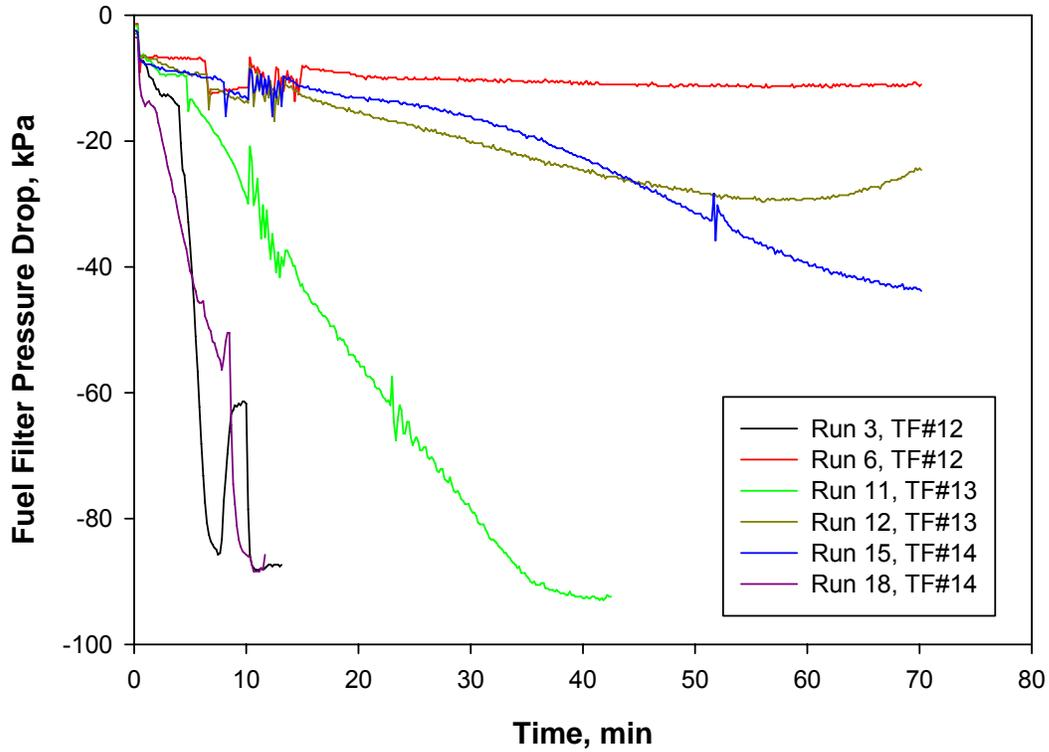
Figure 9. Primary fuel filter pressure drop for tests run on Truck A2.
