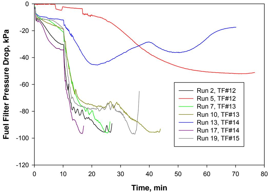
Figure 10. Primary fuel filter pressure drop for tests run on Truck C2.
