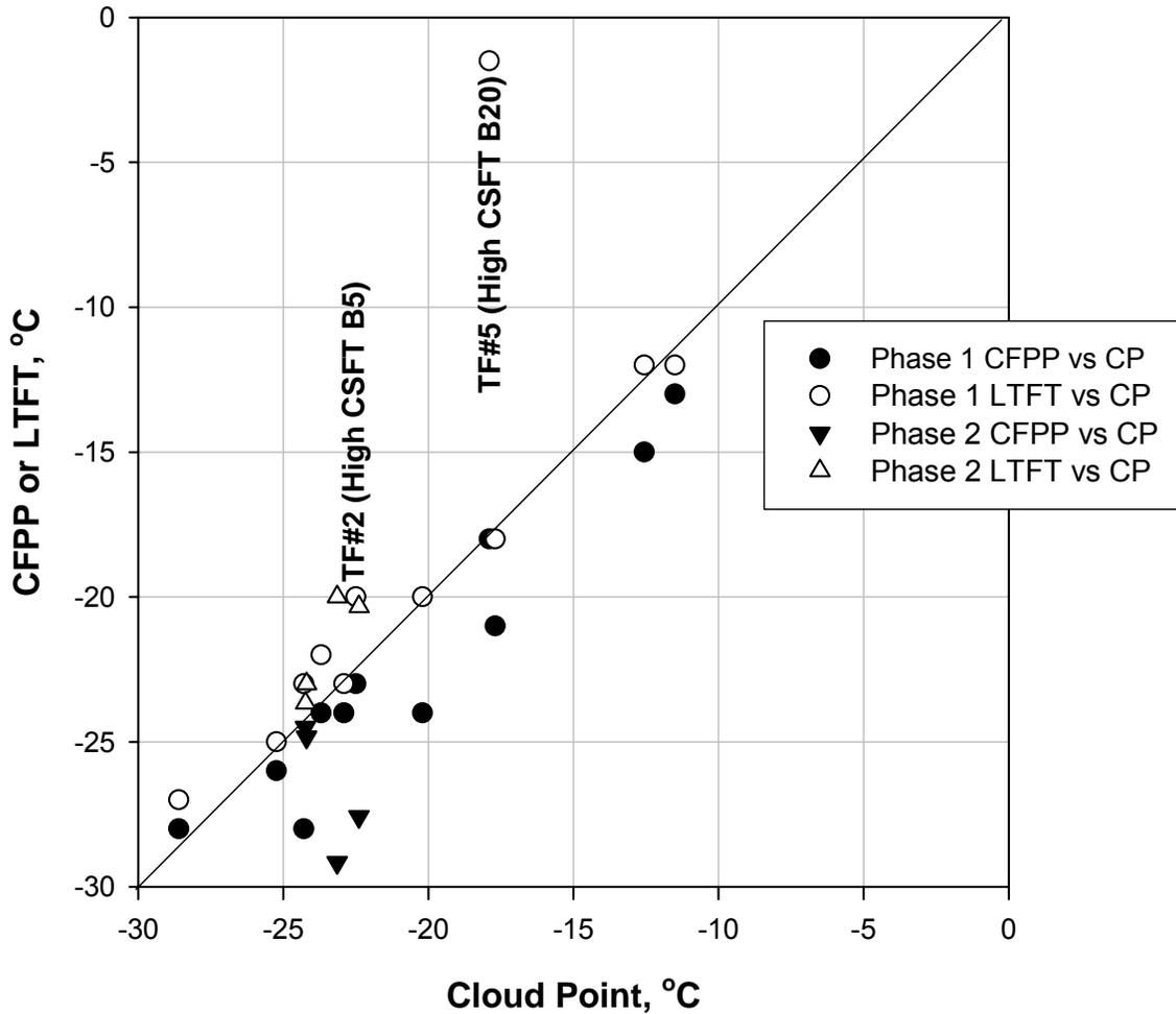
Figure 5. Comparison of CP with CFPP and LTFT for B5 and B20 blends.
