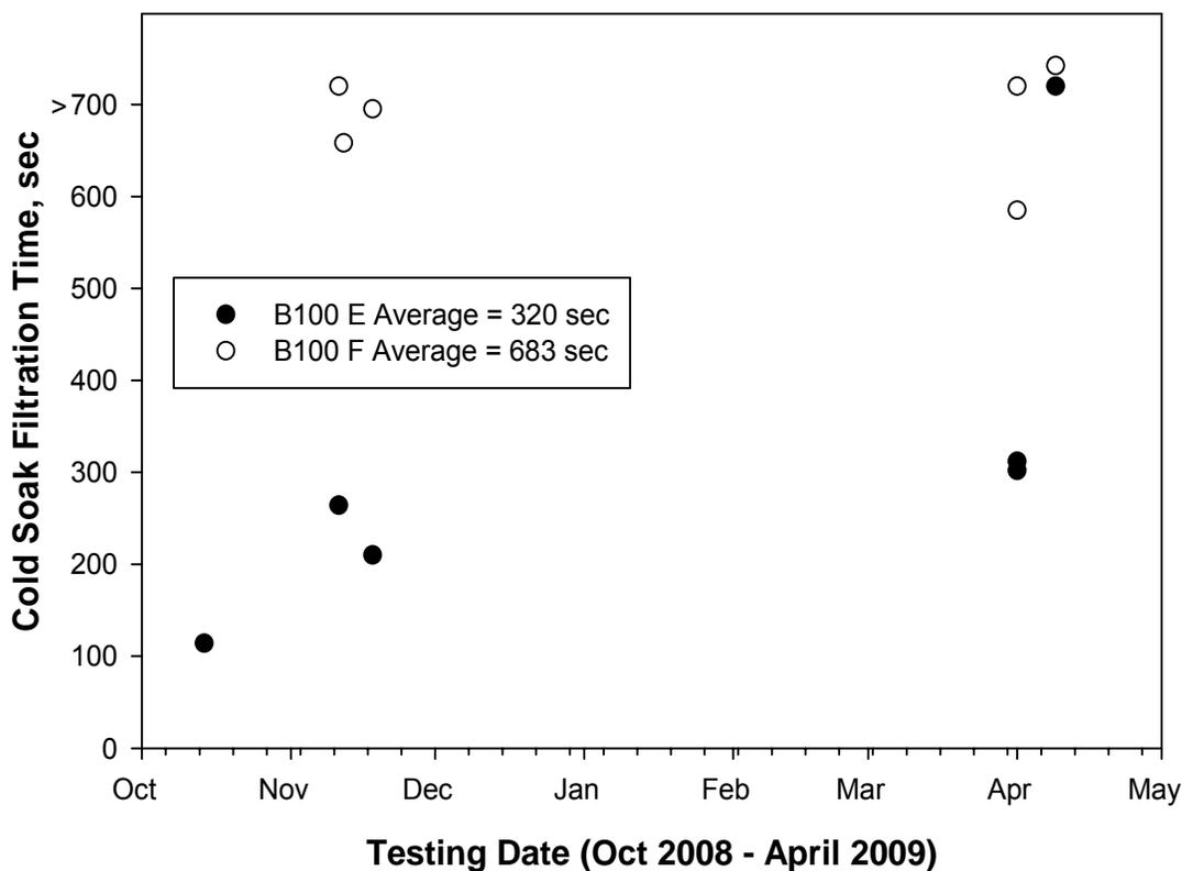
Figure 4. Cold soak filtration time results for B100 samples.
