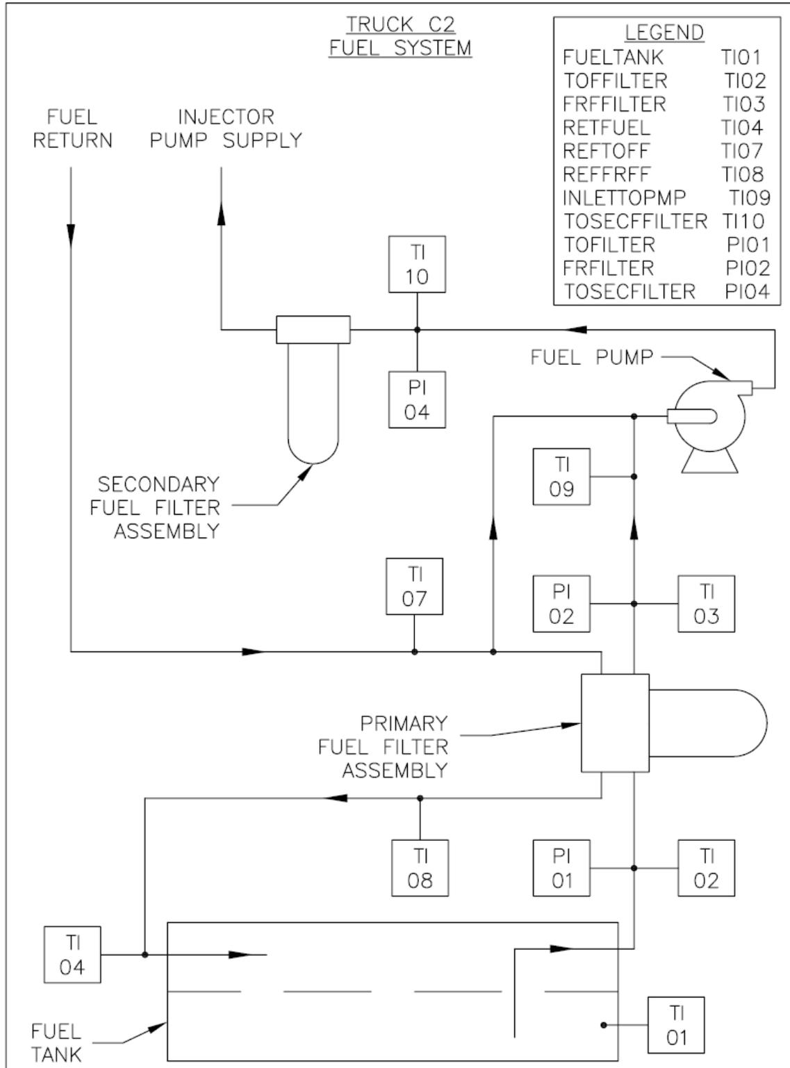
**Figure 2. Vehicle fuel system diagram for Truck C2.**
