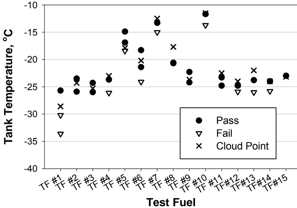
Figure 8. Operability test results for Trucks D and D2.
