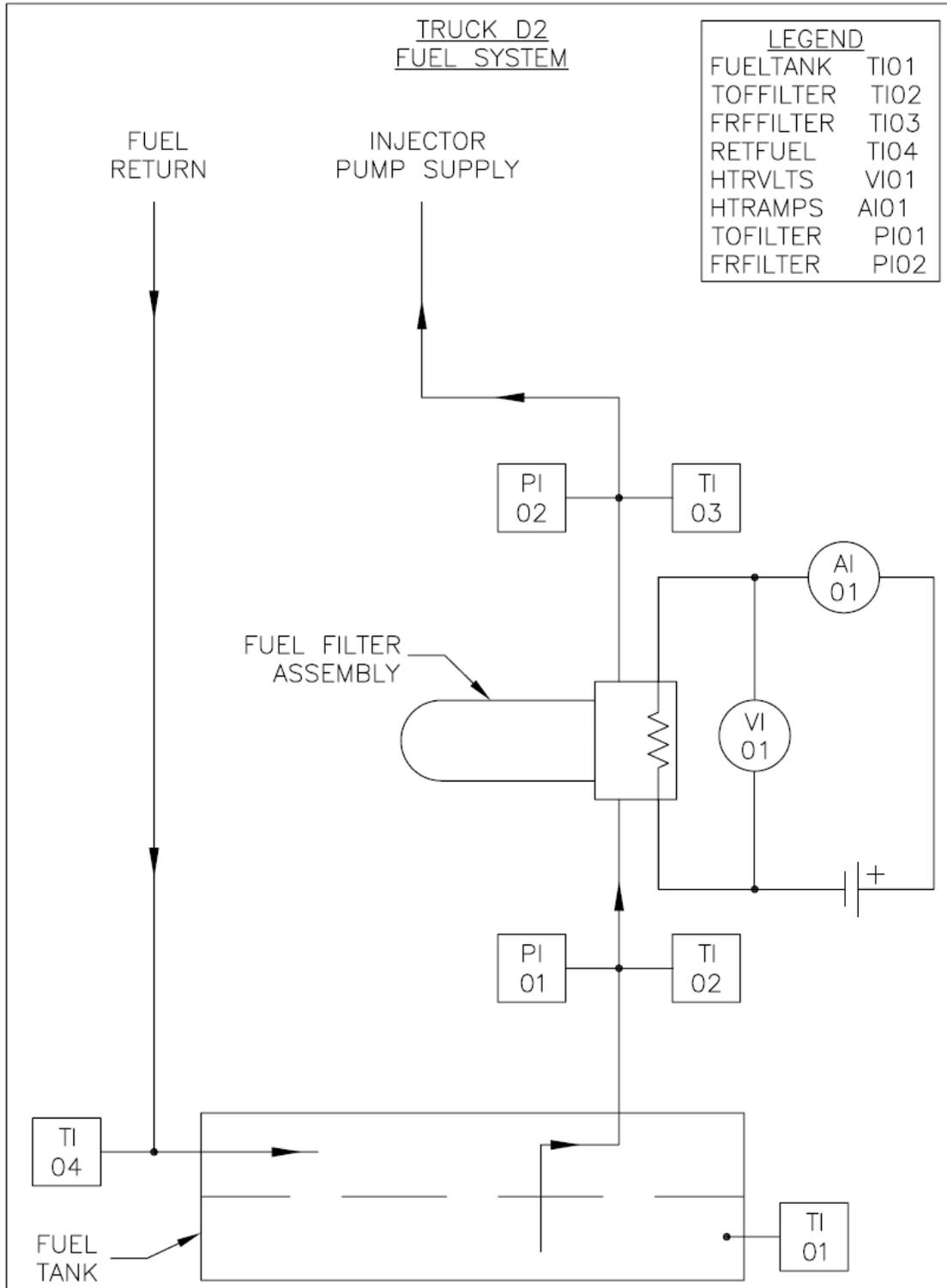
**Figure 3. Vehicle fuel system diagram for Truck D2.**
