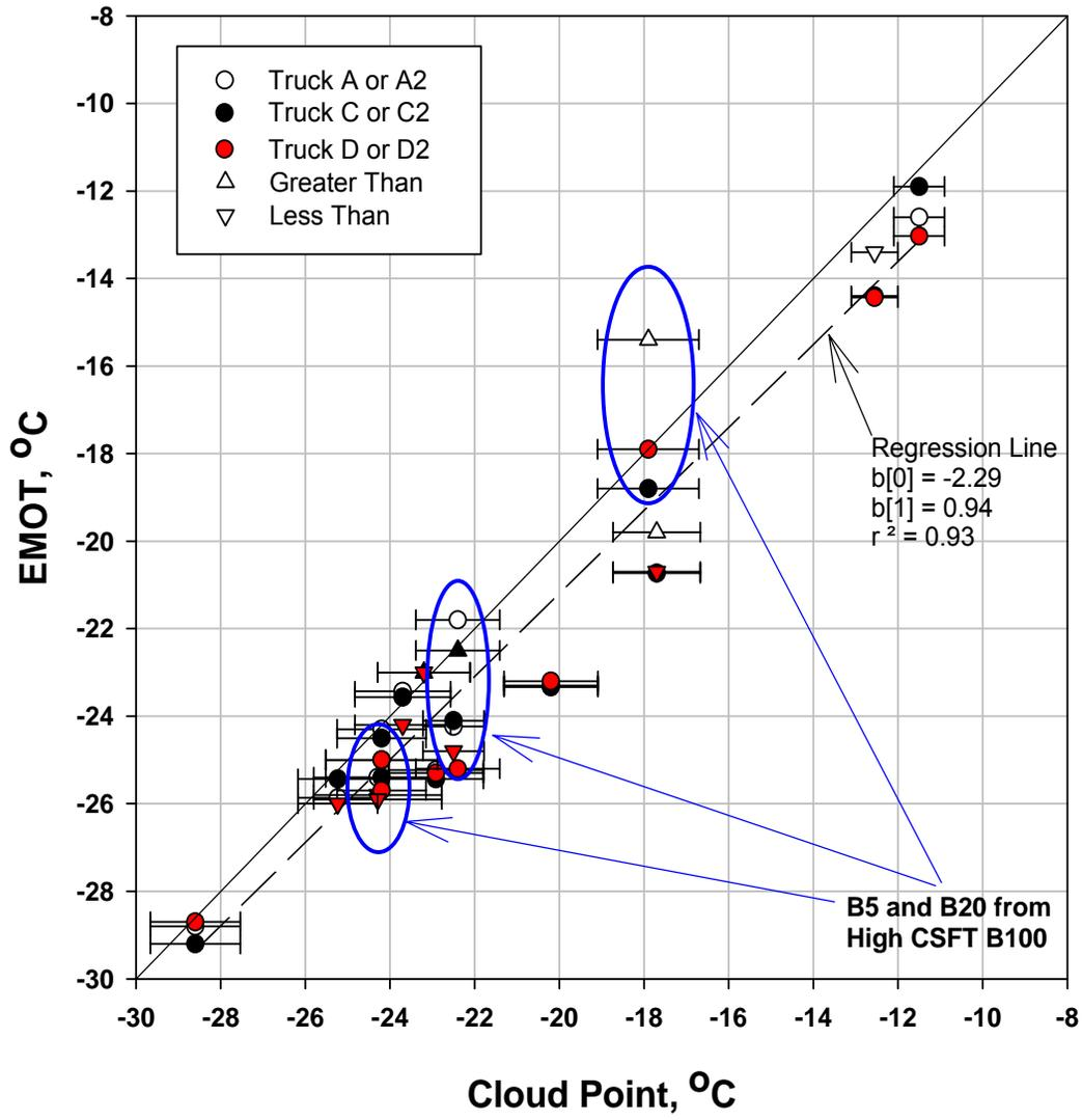
Figure 16. EMOT as a function of CP for all fuels tested (95% confidence interval shown for CP).
