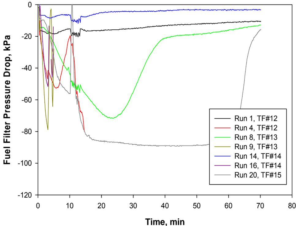
Figure 11. Primary fuel filter pressure drop for tests run in Truck D2.
