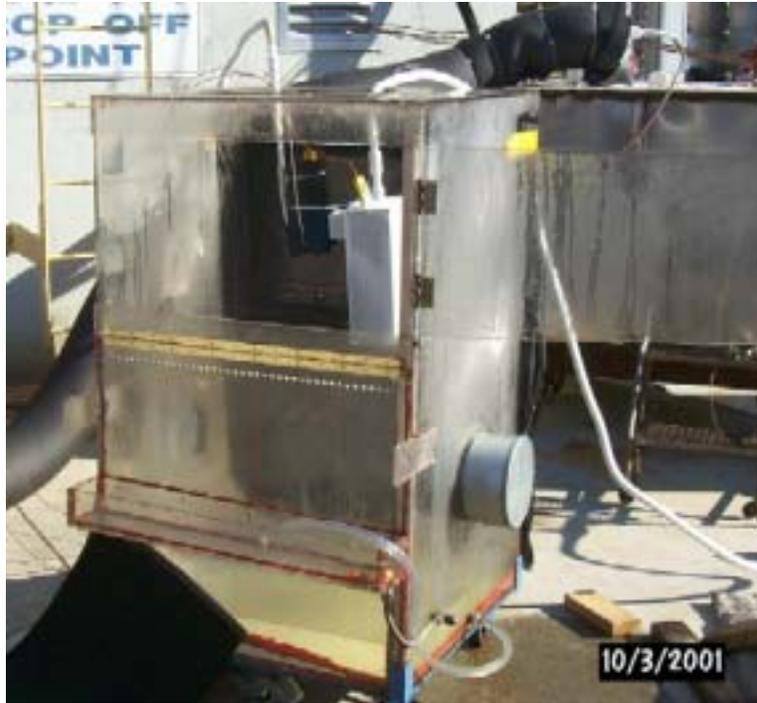
**Figure 19. Spray Chamber** *Door open, fuel nozzle spray box mounted and being cooled down.*
