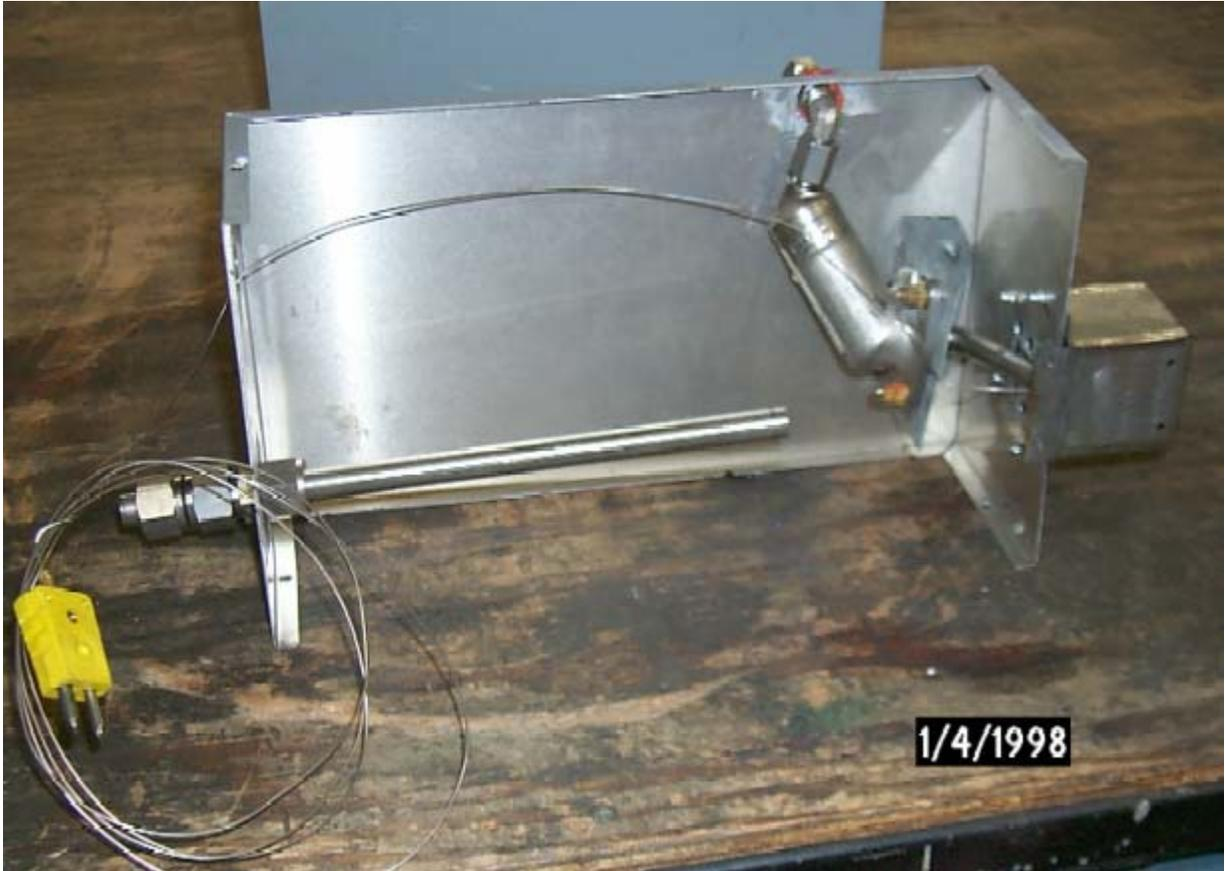
**Figure 21. CFM56 Fuel Nozzle** *Note small housing to account for offset of fuel nozzle tip.*
