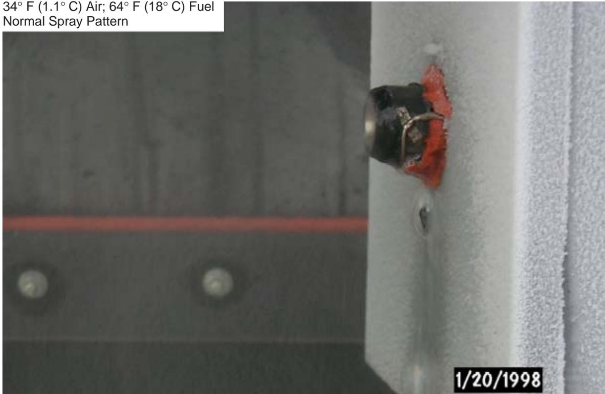
Figure 22. CF6 Fuel Nozzle at Starting Flow
