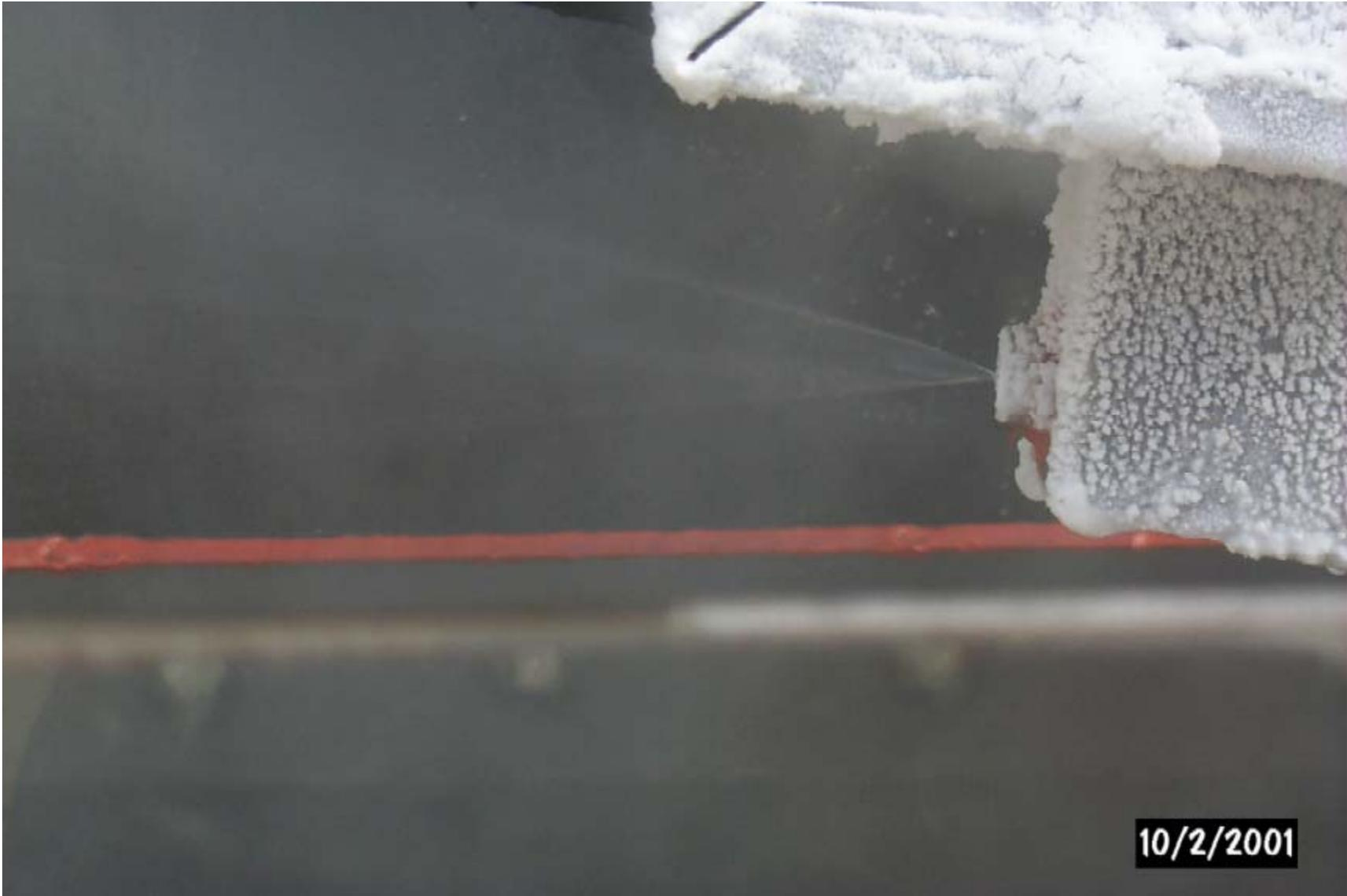
**Figure 26. CFM56 Nozzle, Neat Fuel** *Spray narrows, becomes streaky, sheets near apex.*
