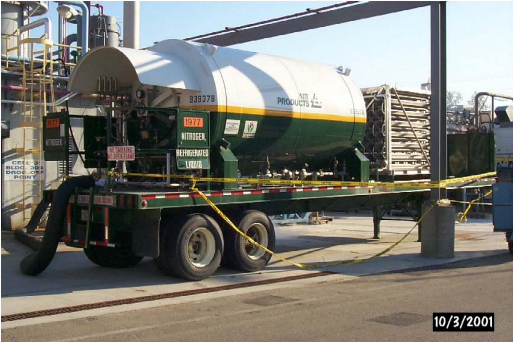
Figure 17. Cryogenic Nitrogen Storage Trailer
