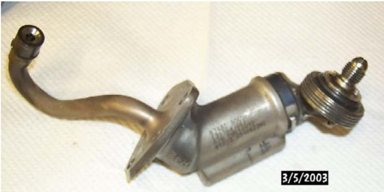
**Figure 30. Test Sector Combustor and Fuel Nozzle** *Combustor is an annular sector of a combustor; fuel nozzle is a standard commercial part.*
