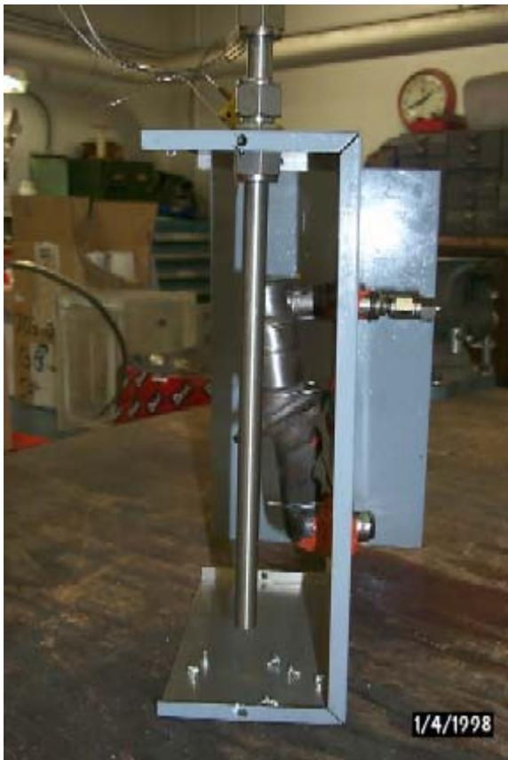
**Figure 20. CF6 Fuel Nozzle in Enclosure** *Air feed tube in foreground. Nozzle fuel inlet is upper horizontal line.*
