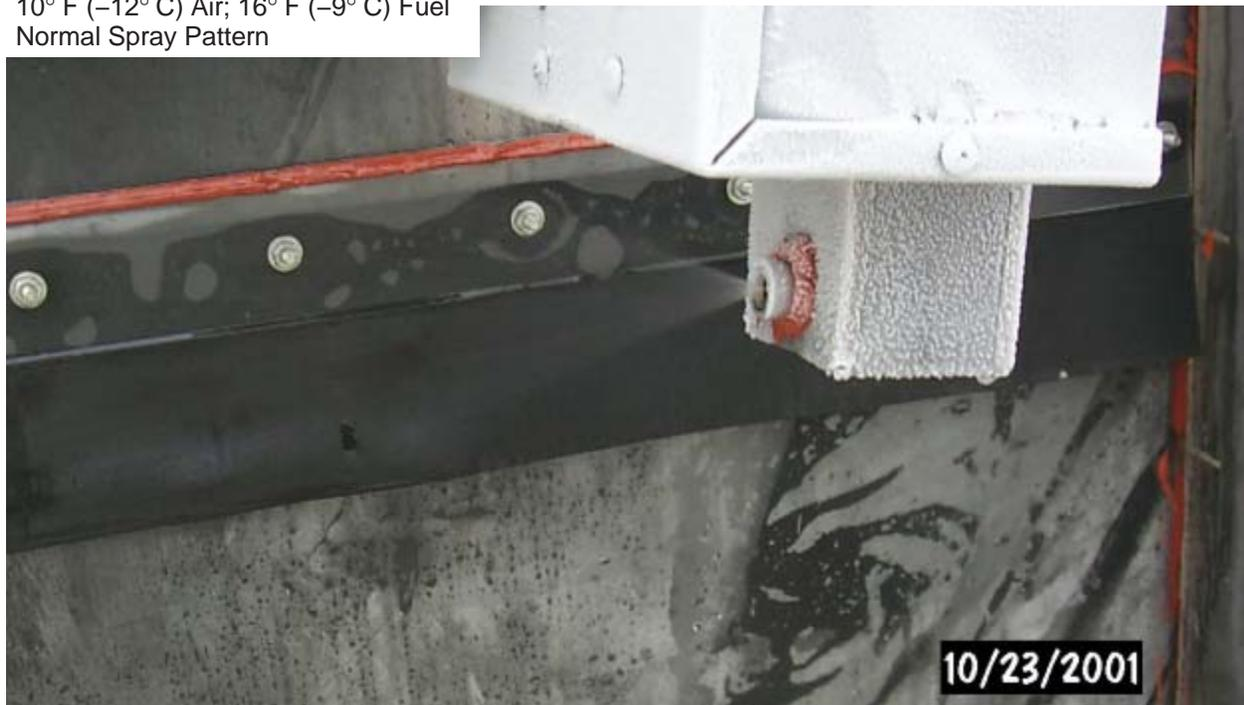
Figure 23. CFM56 Nozzle, Starting Flow
