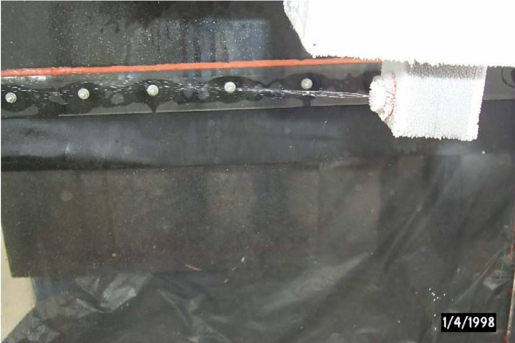
**Figure 28. CFM56 Nozzle, 32-ppm PDR** *Spray cone collapsed to a Stream. Spray reestablished at over 3X starting flow.*
