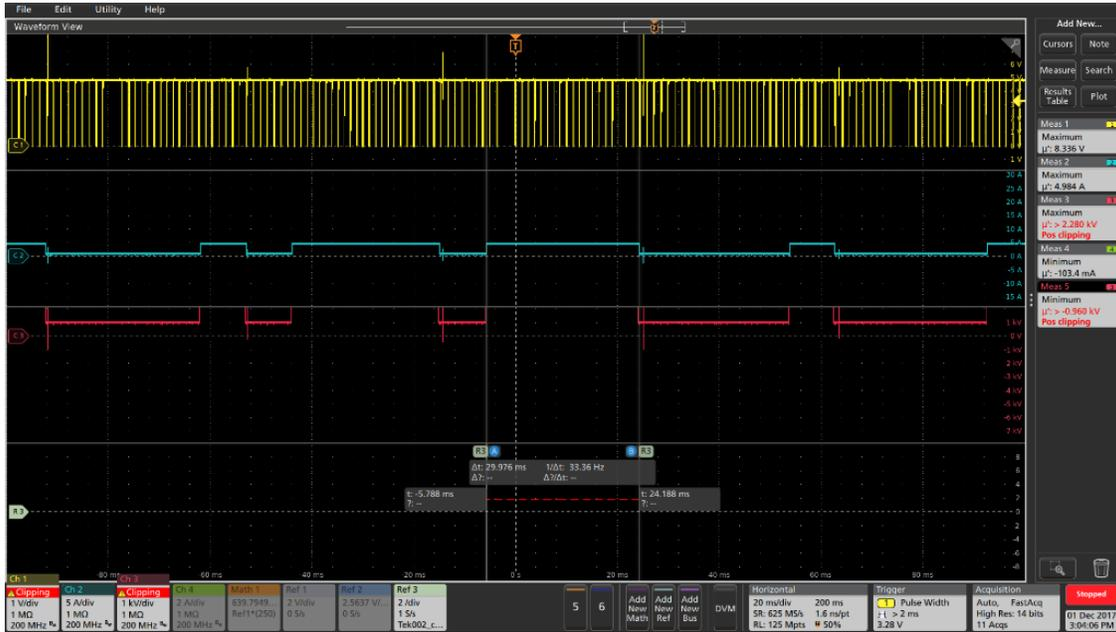
**Figure 4. Crank (Yellow), Intake Cam (Blue) and Exhaust Cam (Red) Signals as Measured using an Oscilloscope**
