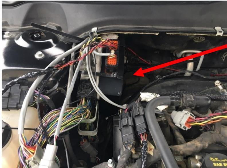
**Figure 9. Direct Injector Driver Mounted near the Vehicle ECM under the Hood**
