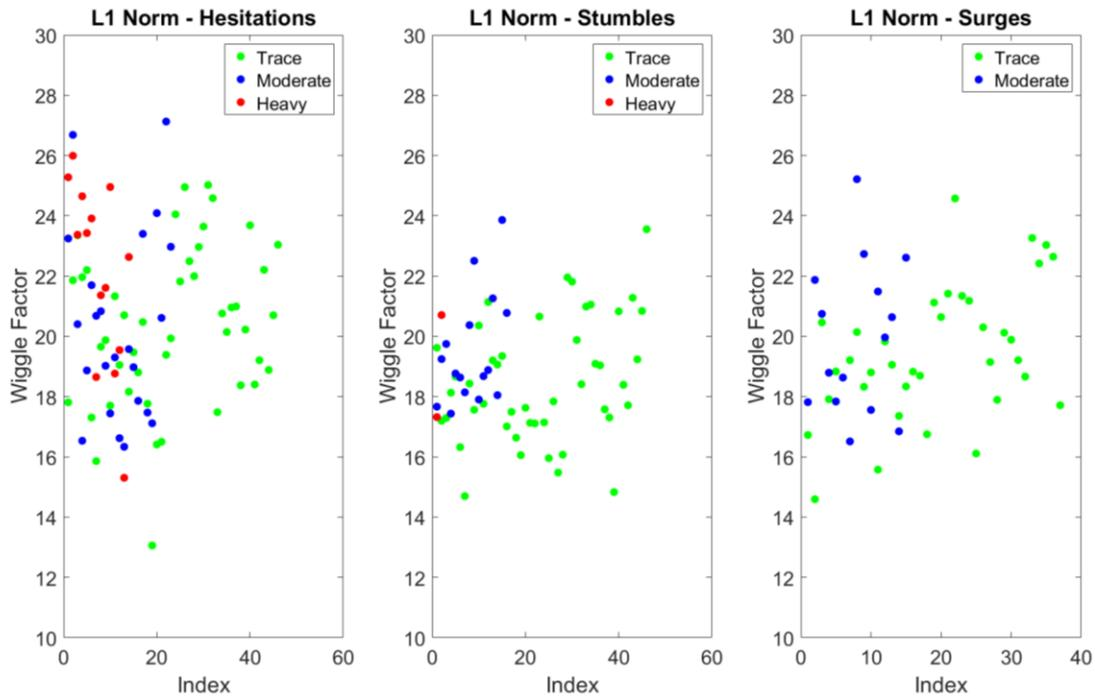
**Figure 43. L1-Norm Value of Pedal Input at Various Reported Severities**
