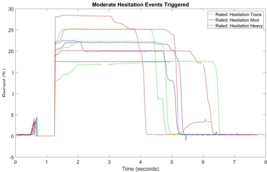
**Figure 42. Raw Pedal Trace for Hesitation Events at Various Reported Severities**
