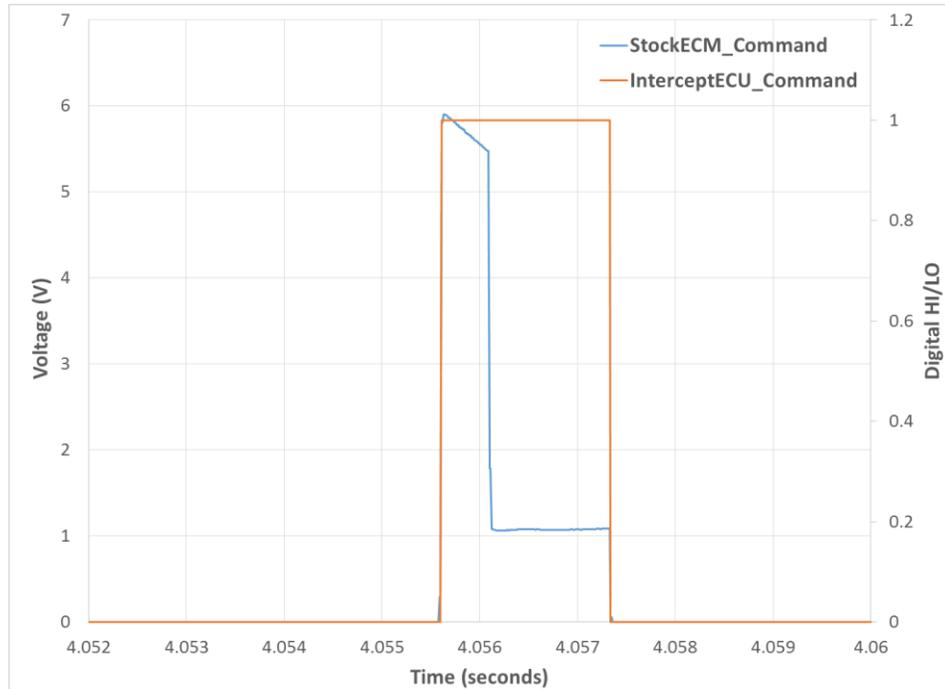
**Figure 7. Injector Operation in Pass-through Mode, Left Axis Corresponds to Scaled Voltage Measured across Dummy Injector and Right Axis is the TTL Output from Intercept ECM to the Direct Injection Driver**
