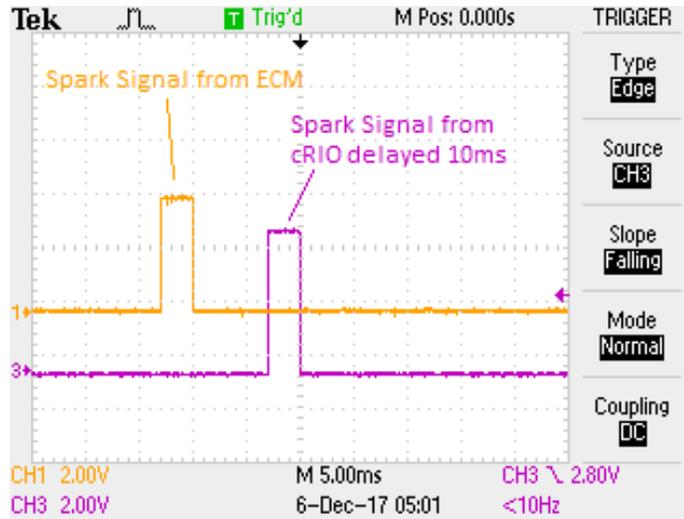
**Figure 5. Spark Signal Intercept and Custom Command from SwRI Intercept Controller**
