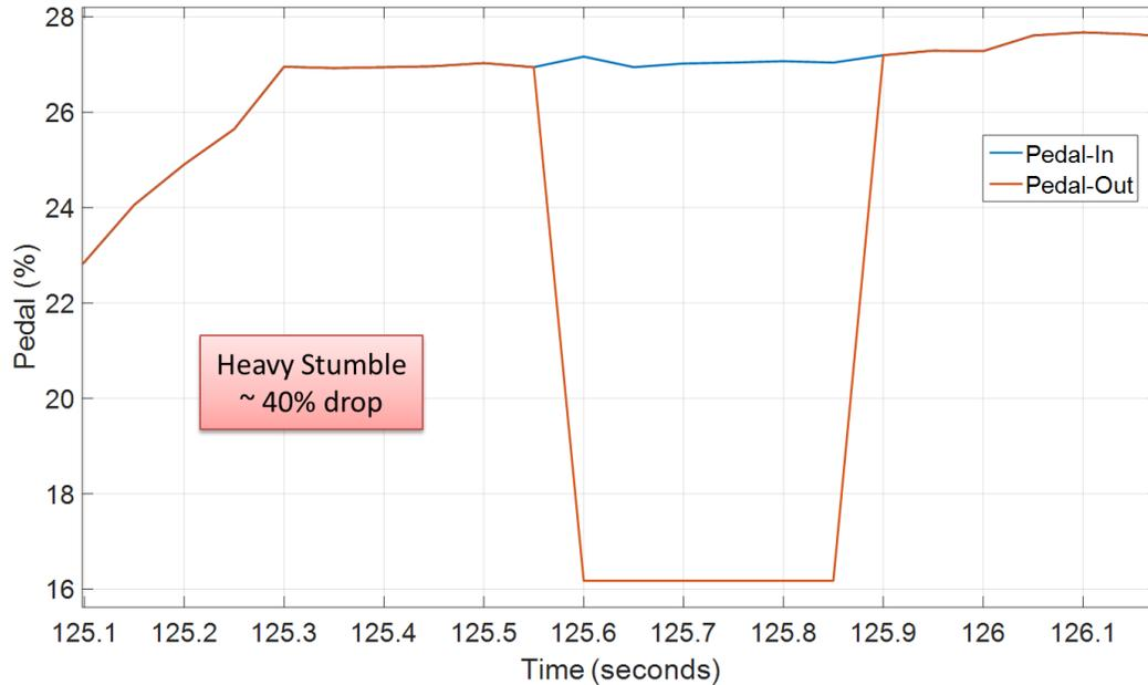
**Figure 17. Pedal Manipulation during a Stumble Event**
