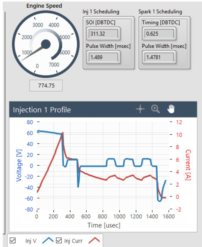
**Figure 6. Synchronization Logic and Fuel Injection/Spark Timing Detection**
