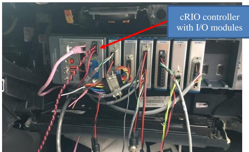
**Figure 8: SwRI Intercept Controller Mounted in the Vehicle Glove Box**
