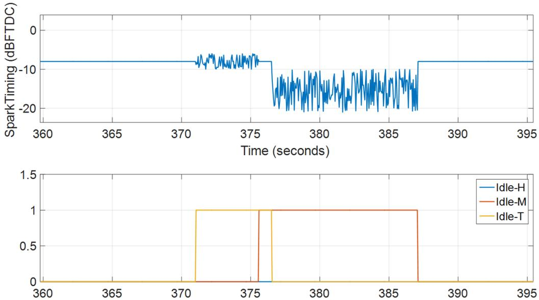
**Figure 15. Data Sample – Idle Quality Event (Top: Spark Timing Command to ECM; Bottom: Button Push Corresponding to Idle-Trace or Moderate Event Trigger)**
