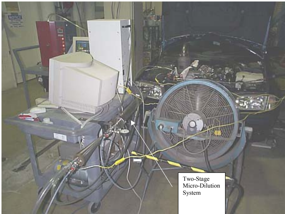
FIGURE 3. PARTICLE SIZE MEASUREMENT SETUP UPSTREAM OF DIESEL OXIDATION CATALYST
