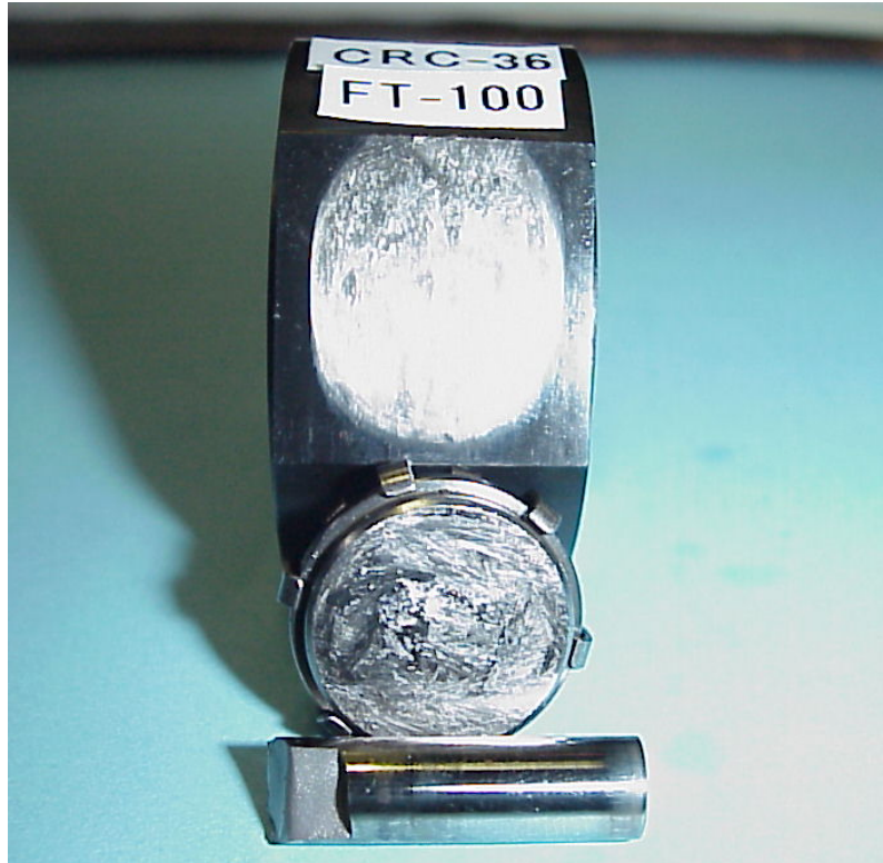
Figure 1-20. FT100 (Test 3) High-Pressure Common Rail Pump Cam Follower and Plunger Follower Wear Scars for Seized and Broken Plunger.
