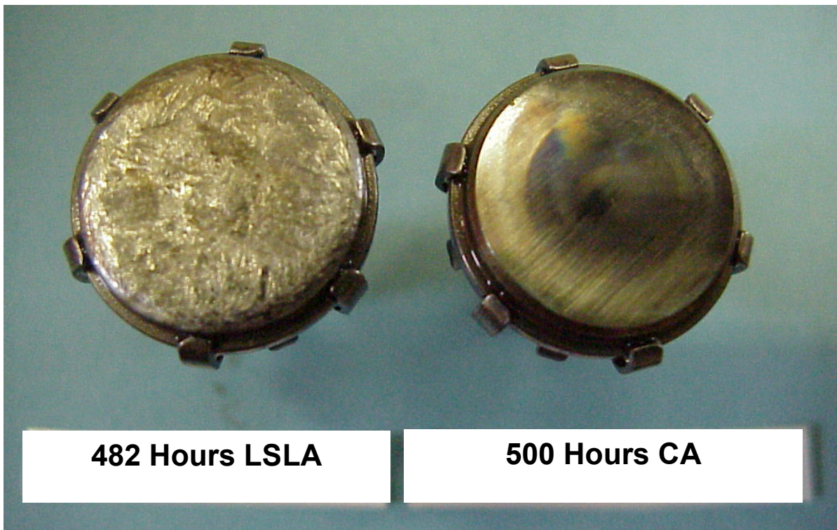
Figure 1-19. Rail Pump Plunger Follower Wear for LSLA (Test 1) and CA (Test 2) Fuels.
