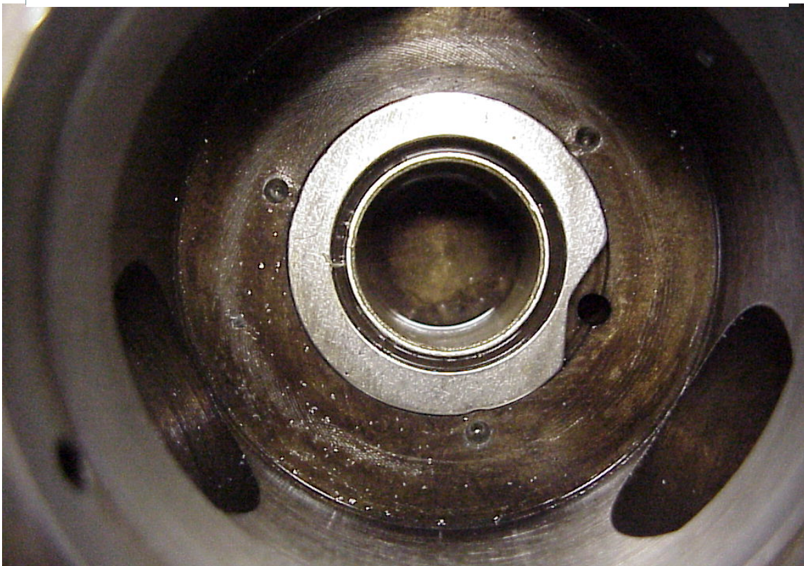
Figure 1-25. Bosch Test 4 with DMM15, Pump Housing Wear Debris.
