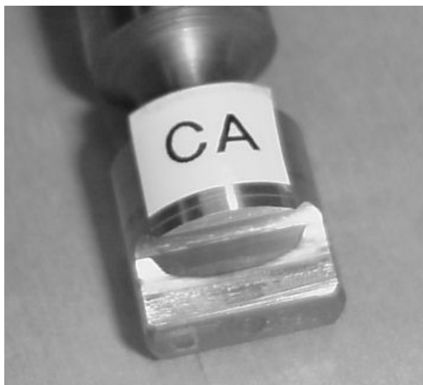
Figure 1-12. Drive Tang from CA Pump SN:8897760
