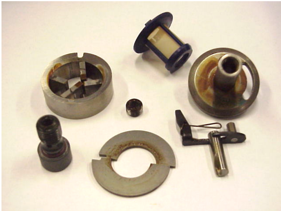
Figure 1-3. Heavy Deposits from CA Fuel from a Stanadyne Pump
