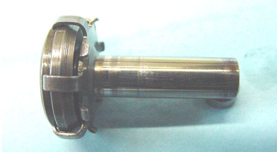
Figure 1-41. LSLA (Test 7) Pump Plunger with Light Polish, Scratches, and Deposition
