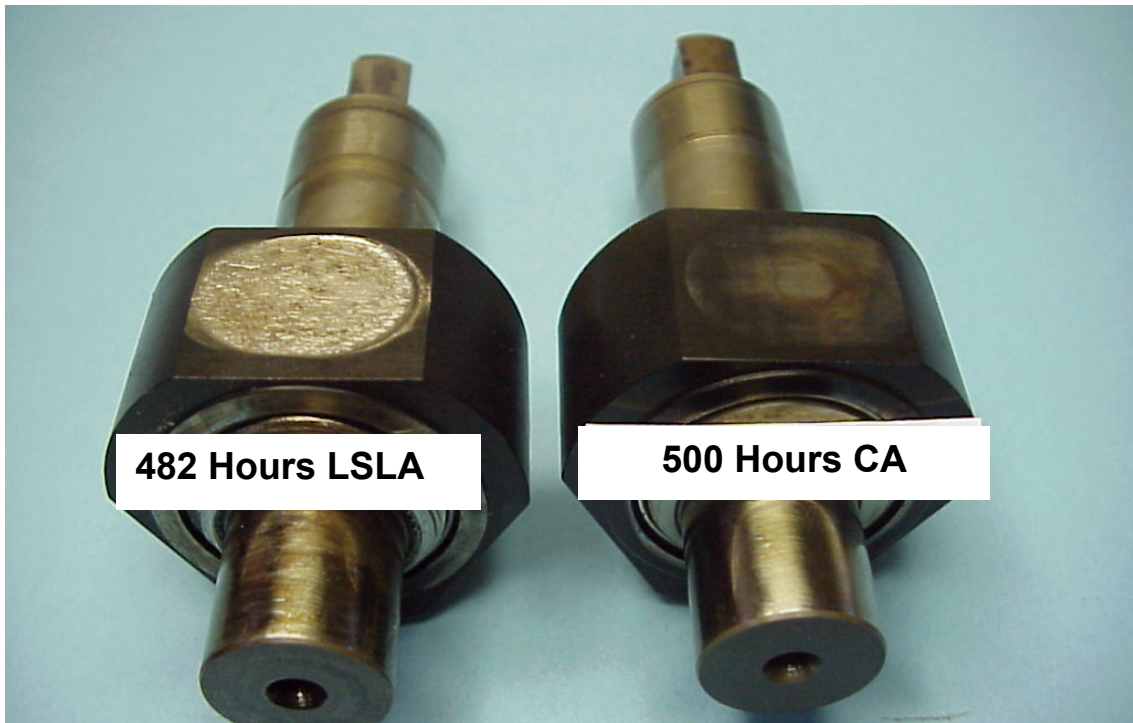
Figure 1-18. Common Rail Pump Eccentric Follower Wear for LSLA (Test 1) and CA (Test 2) Fuels.
