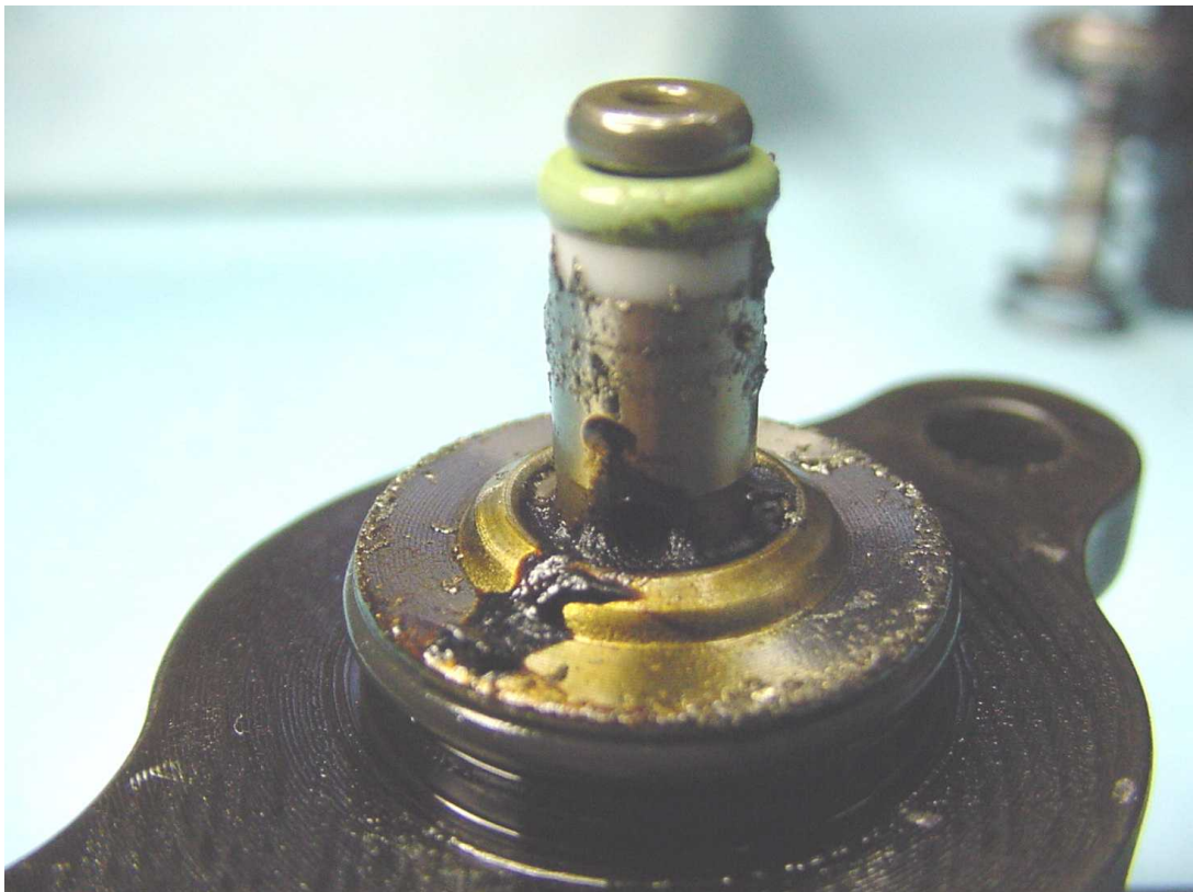
Figure 1-29. FT100 (Test 5) Rail Pressure Regulator with Deposits
