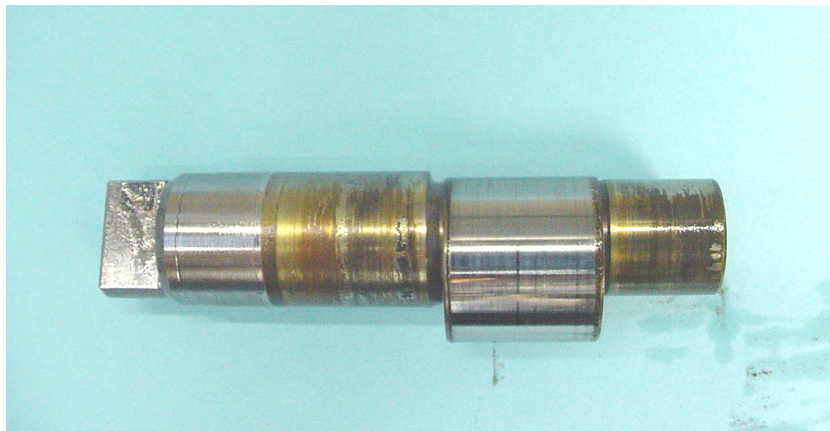
Figure 1-43. LSLA (Test 7) Common Rail Pump Shaft with Deposits.
