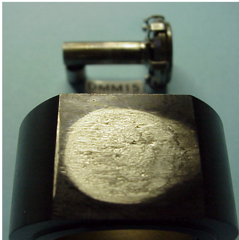
Figure 1-23. Wear Scar on DMM15 (Test 4) Cam Follower.
