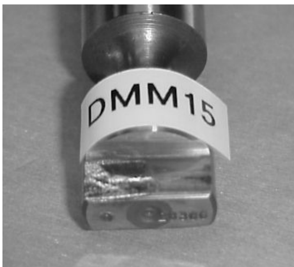
Figure 1-13. Drive Tang from DMM15 Pump SN:8897772
