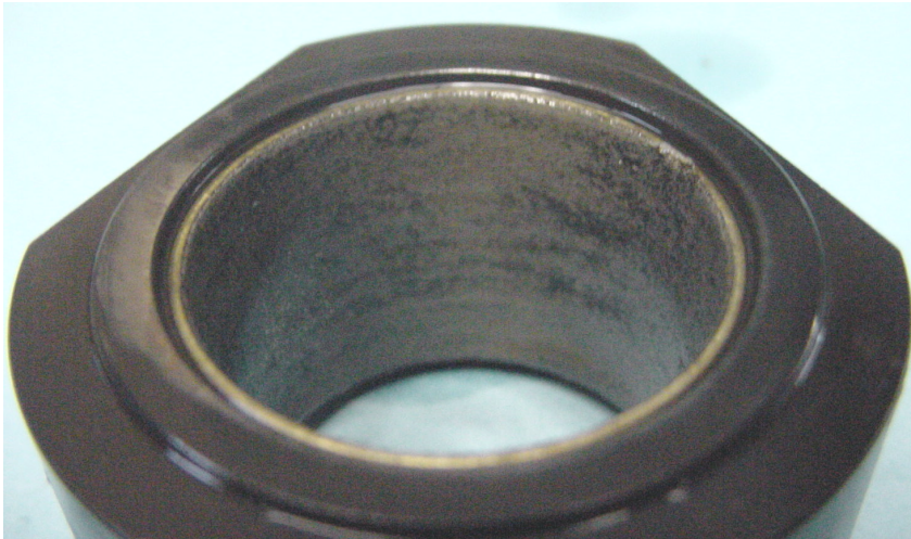
Figure 1-42. LSLA (Test 7) Cam Follower with Bearing Pitting.
