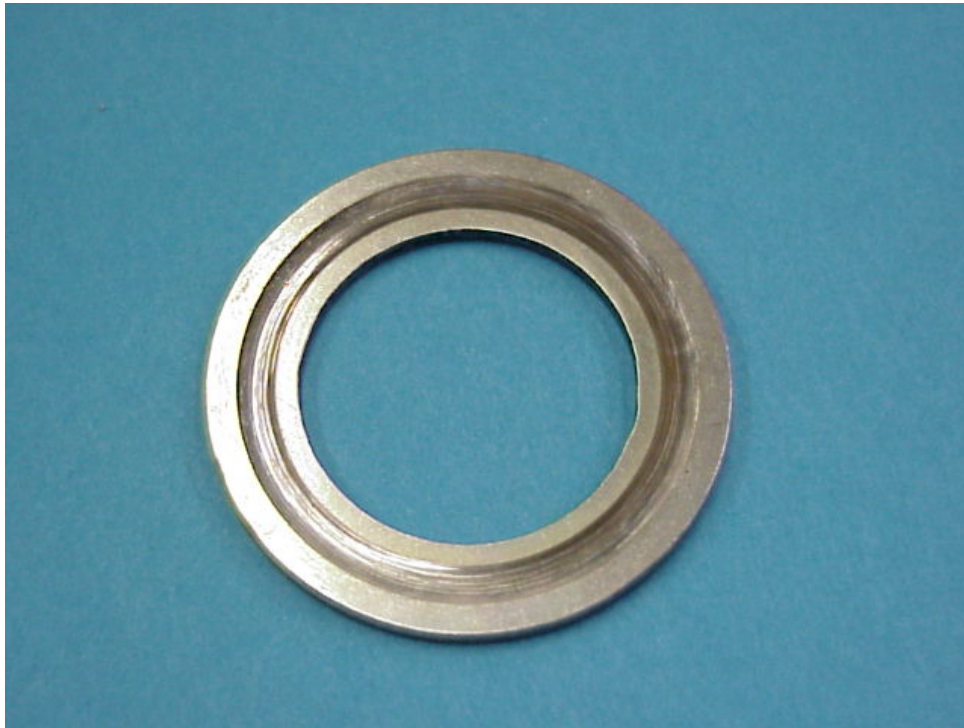
Figure 1-2. Governor Thrust Washer Wear Groove with CA Fuel
