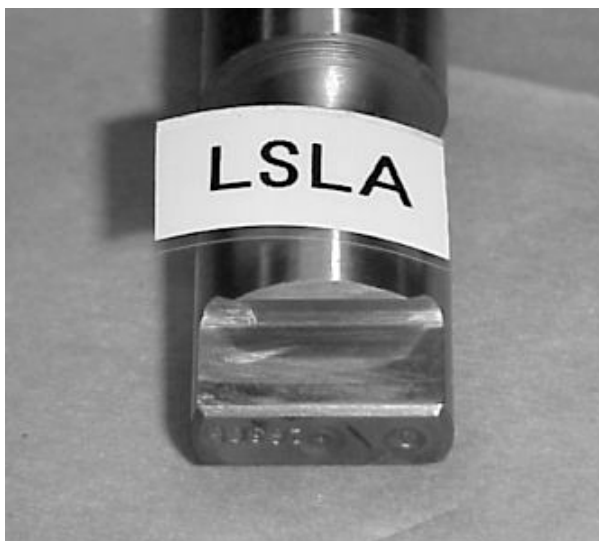
Figure 1-11. Drive Tang from LSLA Pump SN:8897758
