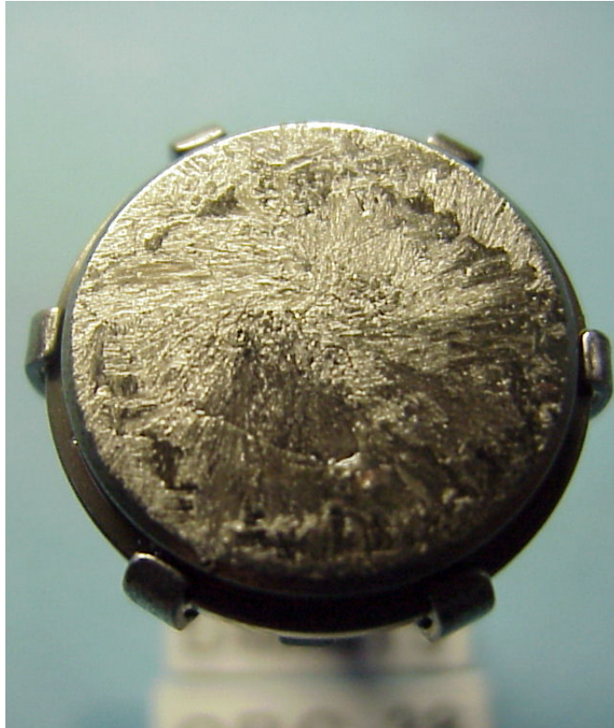
Figure 1-22. Wear Scar on DMM15 (Test 4) Plunger Follower.
