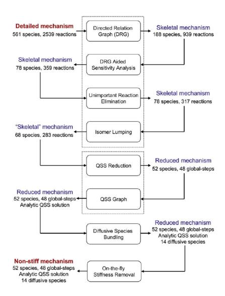
Figure 7. Flow chart of the integrated reduction procedure for an n-heptane mechanism [105].
