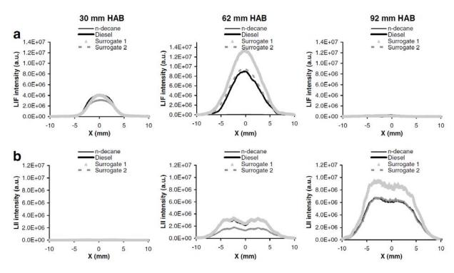
Figure 5. Radial profiles of (a) laser-induced fluorescence of PAH and (b) laser-induced incandescence (LII) of soot particles obtained at different heights above the burner (HAB) in each flame. Surrogate 1 is original IDEA fuel of 30% 1-MN/70% n-decane. Surrogate 2 is new proposed surrogate of 20% 1-MN/80% n-decane. N-decane signals are very weak indicating near zero soot on this plot. The triangles and dashed line sometimes appear as solid lines [83].
