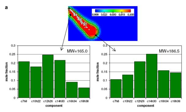
Figure 9. Computed concentration of vaporized hydrocarbons in a surrogate diesel spray from a multi-component vaporization model at 0.5 ms after start of injection [122].
