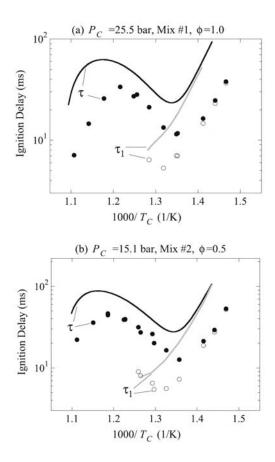
Figure 4. Comparison of experimental (symbols) and computed (lines) ignition delays of methylcyclohexane for (a) compressed gas pressure,  $P_C$  =25.5 bar, Mix #1 ( $O_2/N_2/Ar$ =10.5/12.25/71.75,  $\phi$  = 1.0) and (b)  $P_C$  = 15.1 bar, Mix #2 ( $O_2/N_2/Ar$ =7.16/16.35/71.75,  $\phi$  = 0.5) [50].
