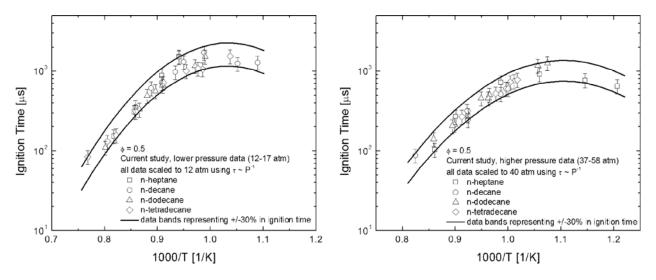
Figure 3. Experimentally measured ignition delay times for C7, C10, C12 and C14 n-alkanes at an equivalence ratio of 0.5 [12]. Reprinted ("Adapted" or "in part") with permission from [12]. Copyright 2009 American Chemical Society.
