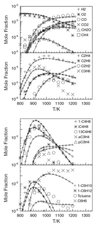
Figure 6. Comparison of a surrogate diesel model and synthetic diesel fuel experiments in a jet stirred reactor at 10 atm and  $\phi$ = 2 (diesel, 0.05%; O<sub>2</sub>, 0.345%; N<sub>2</sub>, 99.6%; residence time = 0.5 s) [91].
