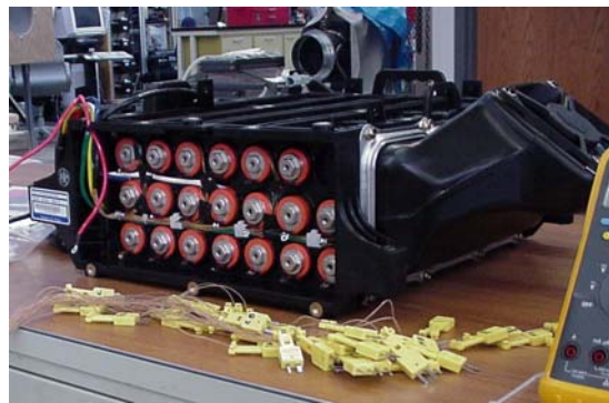
Figure 1, Honda Insight Battery Pack
