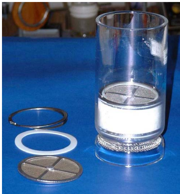
FIGURE 4. XAD-2 GLASS CARTRIDGE FOR SAMPLING SEMI-VOLATILE HYDROCARBONS
