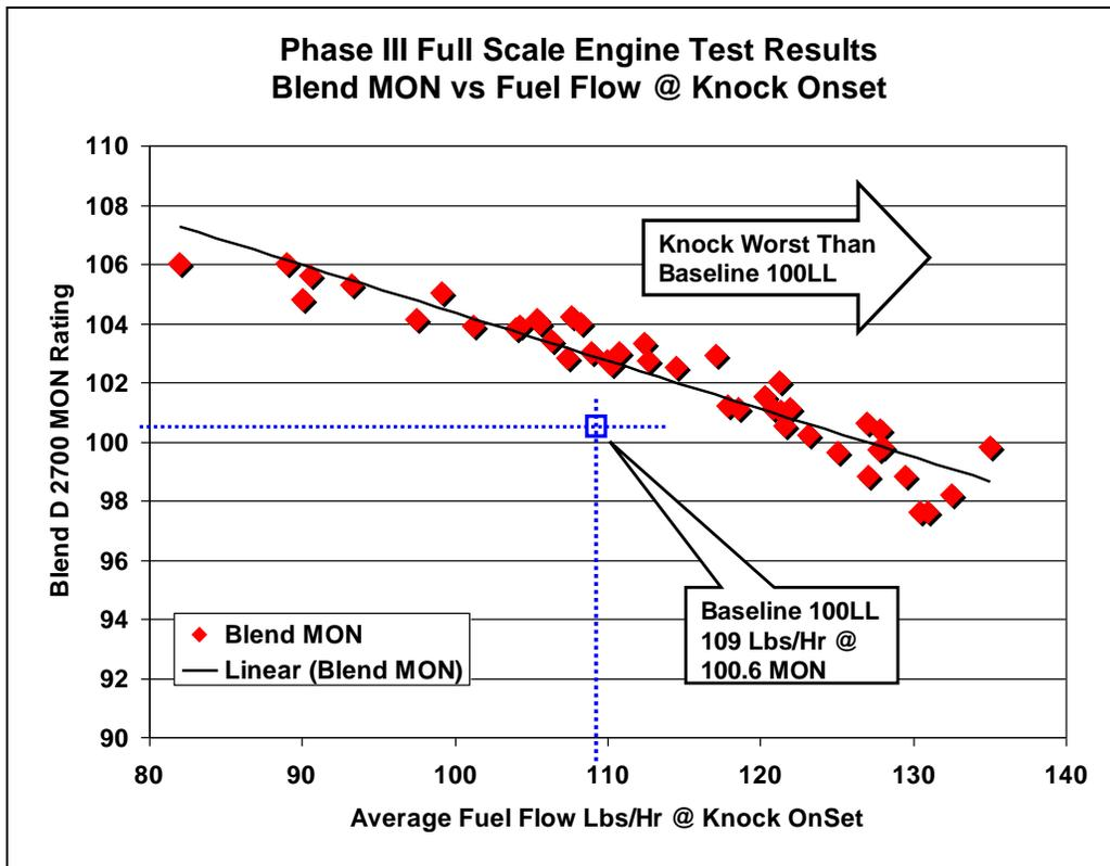
Figure 61.0 – Phase III Blend MON vs Knock Onset Average Fuel Flow <sup>(15)</sup>
