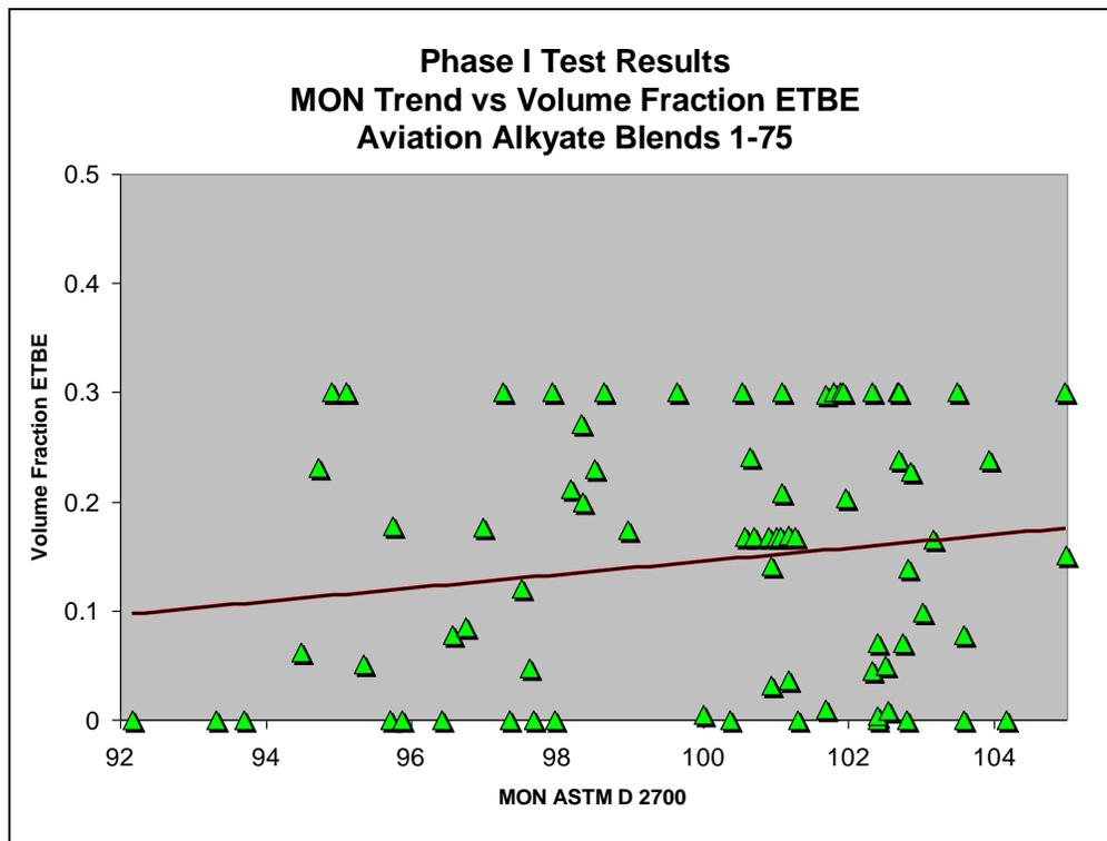
Figure 20.0 - Phase I, MON Trend vs ETBE Volume Fraction
