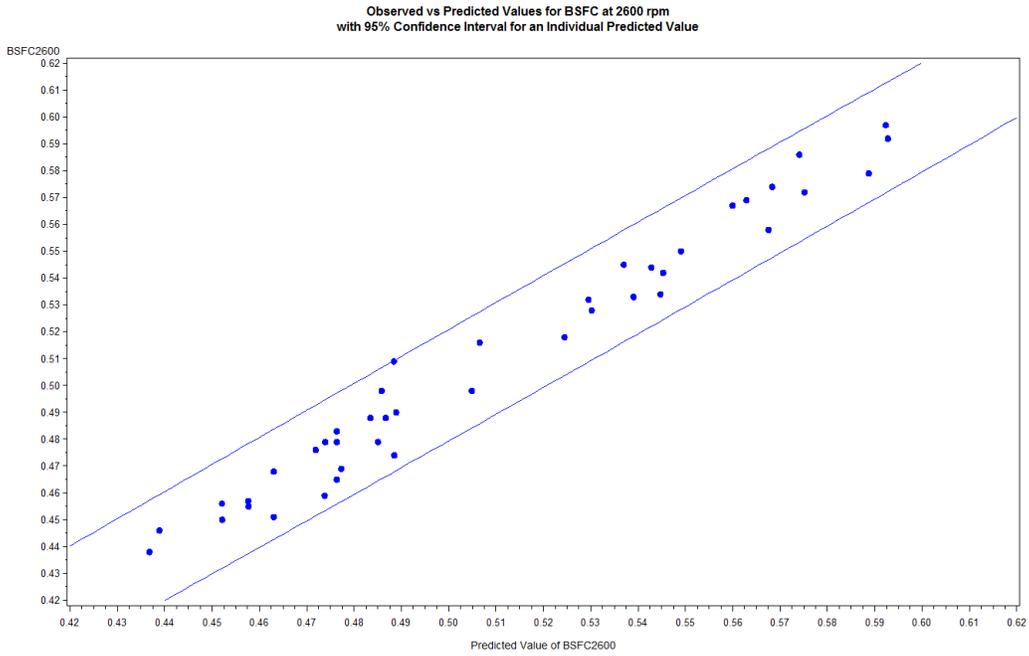
Figure 43 Observed versus Predicted Values for BSFC at 2600 rpm with 95% Confidence Interval for an Individual Predicted Value
