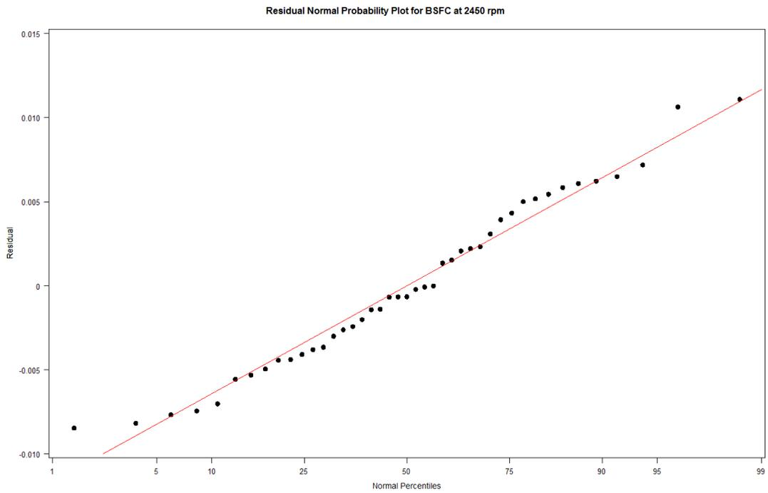
Figure 42 Normal Probability Plot of BSFC at 2450 rpm Residuals
