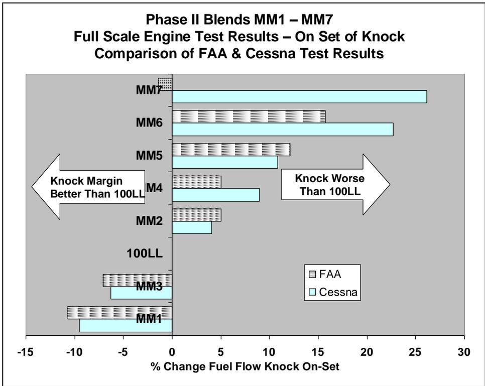
Figure 53.0 – Comparison FAA & Cessna Results MM1-MM7
