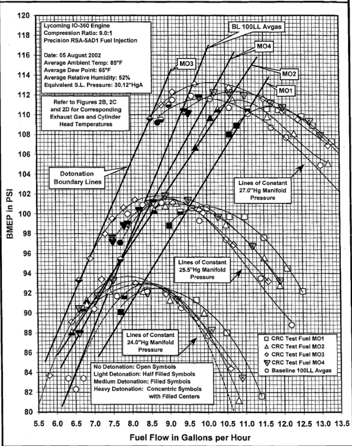
Figure 42.0 – Cessna Knock Test, Mixture Lean Out, Blends MO1-MO4 <sup>(13)</sup>
