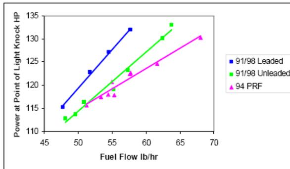
Figure 10: A Comparison of Detonation Limited Power Output versus Fuel Flow for 94 PRF, Leaded and Unleaded AVGAS at 2600 RPM
