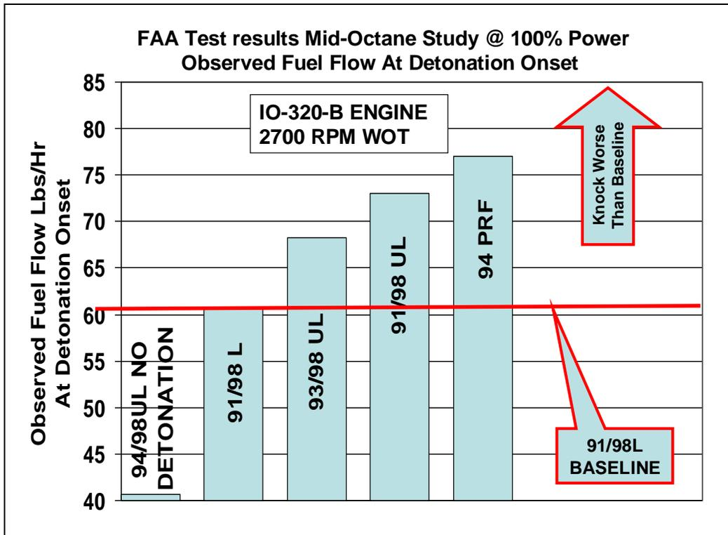
Figure 76.0 – Effect of Mid-Octane Fuels – “Fuel Flow at Detonation On-Set”
