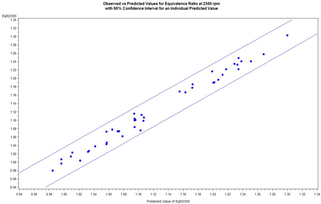
Figure 22 Observed versus Predicted Values for Equivalence Ratio at 2350 rpm with 95% Confidence Interval for an Individual Predicted Value
