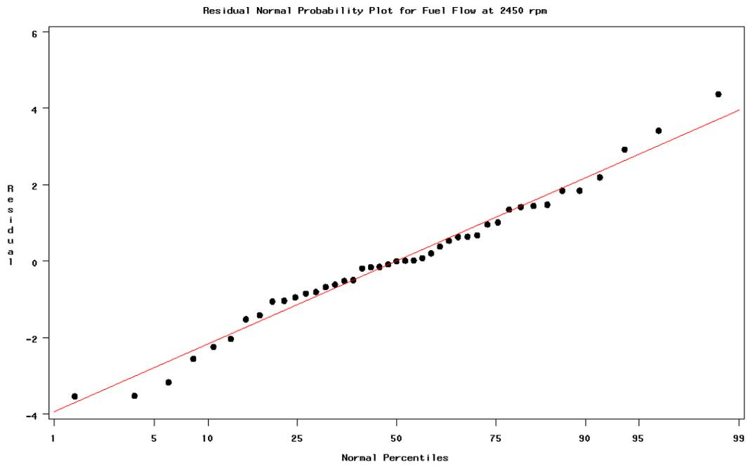
Figure 12 Normal Probability Plot of Fuel Flow at 2450 rpm Residuals
