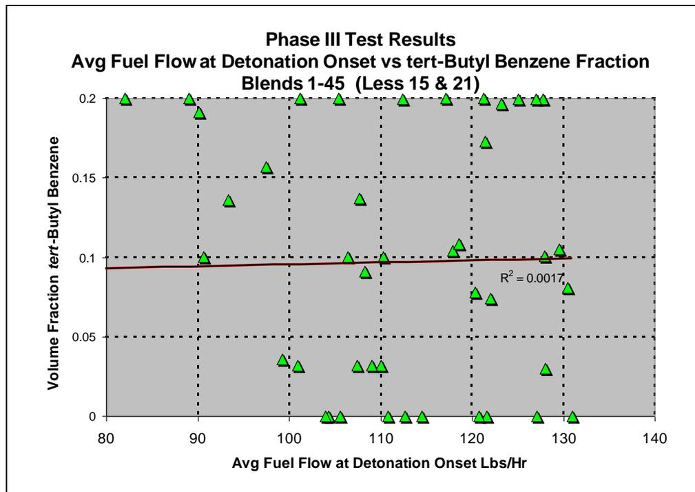
Figure 66.0 – Effect of *tert*-Butyl Benzene on Knock Onset Average Fuel Flow
