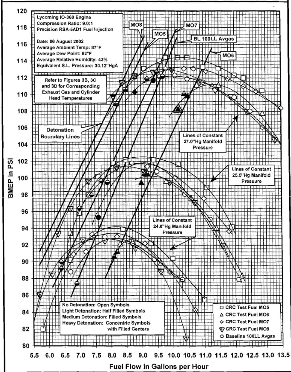
Figure 43.0 – Cessna Knock Test, Mixture Lean Out, Blends MO5-MO8 <sup>(13)</sup>
