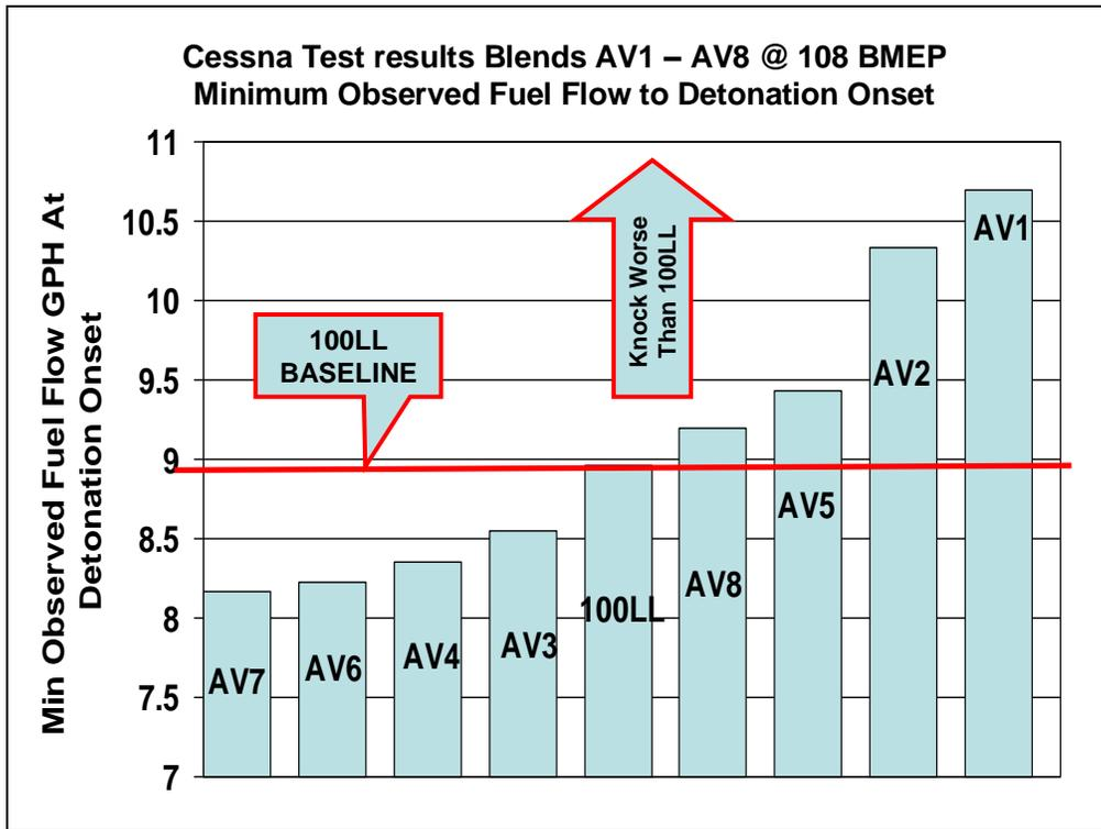
Figure 46.0 – Relative Ranking Blends AV1 – AV8, Cessna Test
