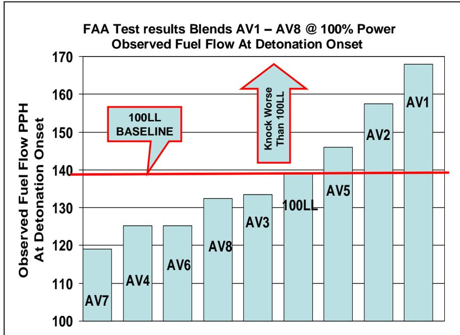
Figure 34.0 – Relative Ranking Blends AV1 – AV8, FAA Test
