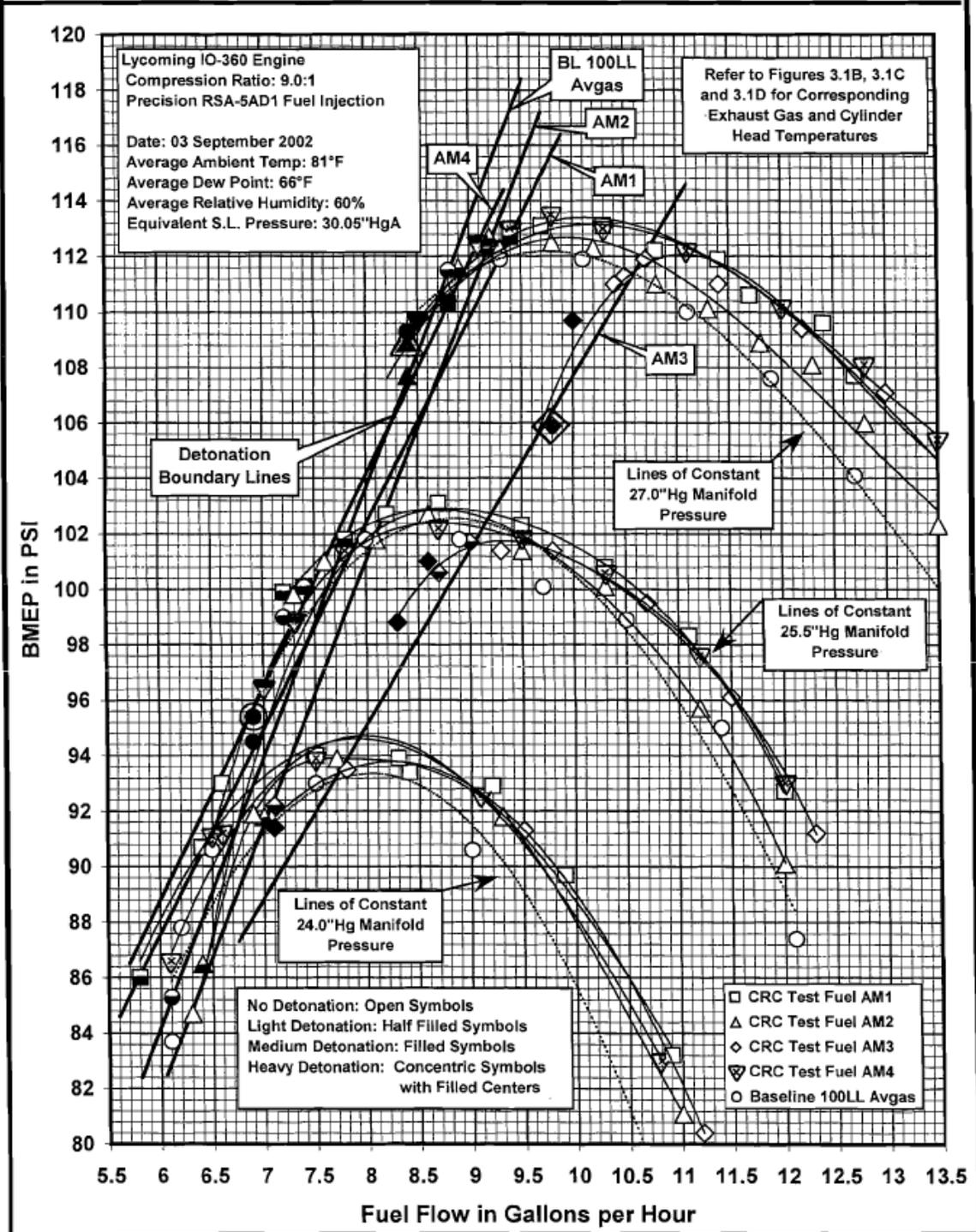
Figure 40.0 – Cessna Knock Test, Mixture Lean Out, Blends AM1-AM4 <sup>(13)</sup>
