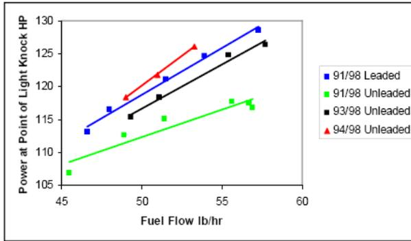
Figure 4: A Comparison of Detonation Limited Power Output versus Fuel Flow for Leaded and Unleaded AVGAS at 2450 RPM
