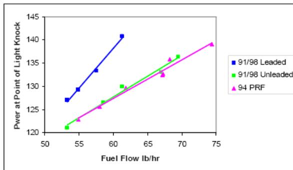
Figure 11: A Comparison of Detonation Limited Power Output versus Fuel Flow for 94 PRF, Leaded and Unleaded AVGAS at 2700 RPM
