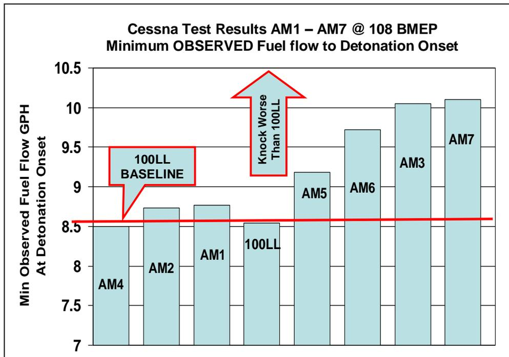
Figure 47.0 – Relative Ranking Blends AM1 – AM7, Cessna Test
