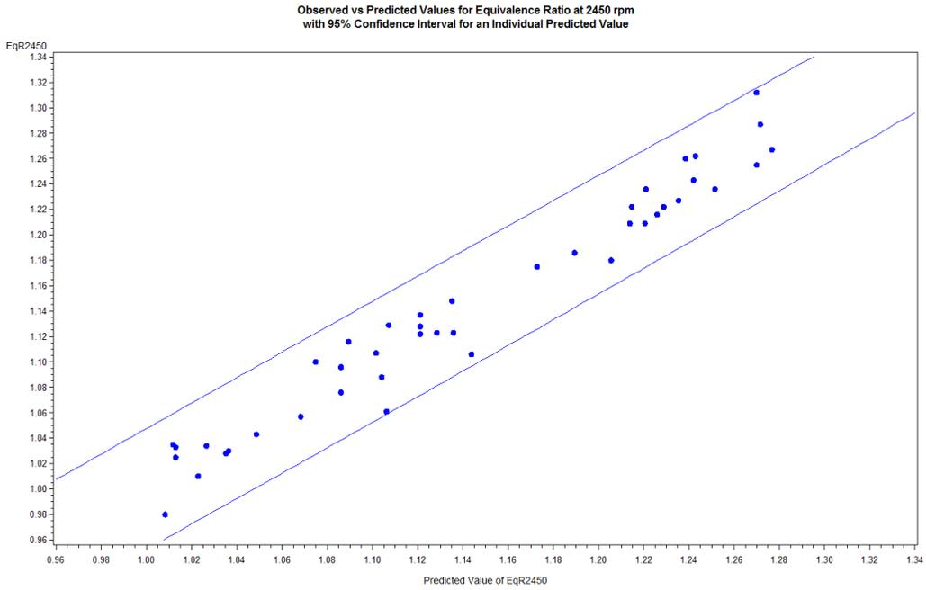
Figure 25 Observed versus Predicted Values for Equivalence Ratio at 2450 rpm with 95% Confidence Interval for an Individual Predicted Value
