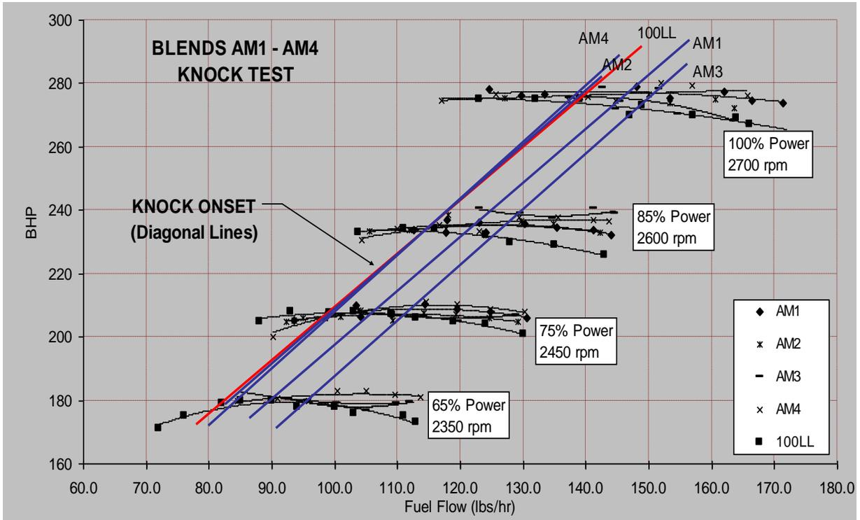
Figure 28.0 – FAA Knock Test, Blends AM1 – AM4 <sup>(12)</sup>
