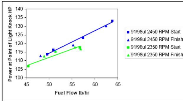
Figure 2: Detonation Limited Power/Fuel Flow Measurements for the 94 Primary Reference Fuel Prior and Post Leaded 91/98 AVGAS Testing
