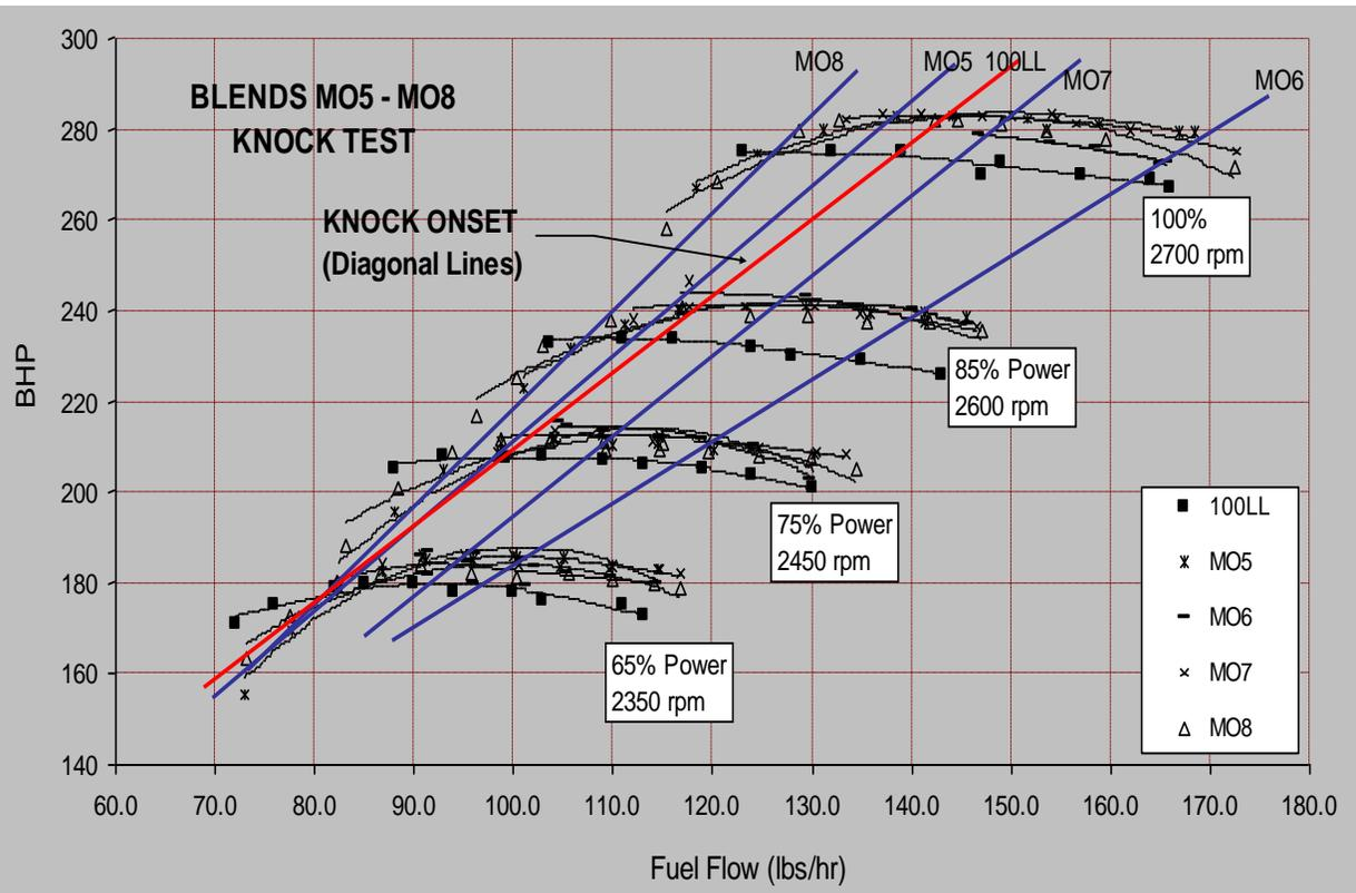
Figure 31.0 – FAA Knock Test, Blends MO5 – MO8 <sup>(12)</sup>
