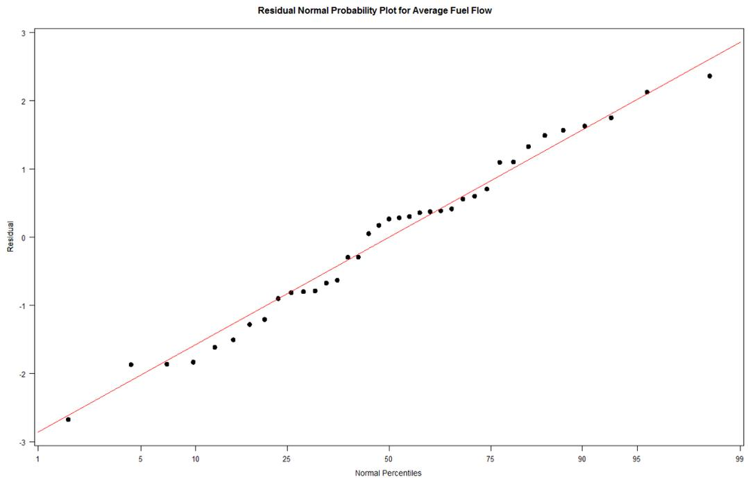
Figure 6 Normal Probability Plot of Average Fuel Flow Residuals
