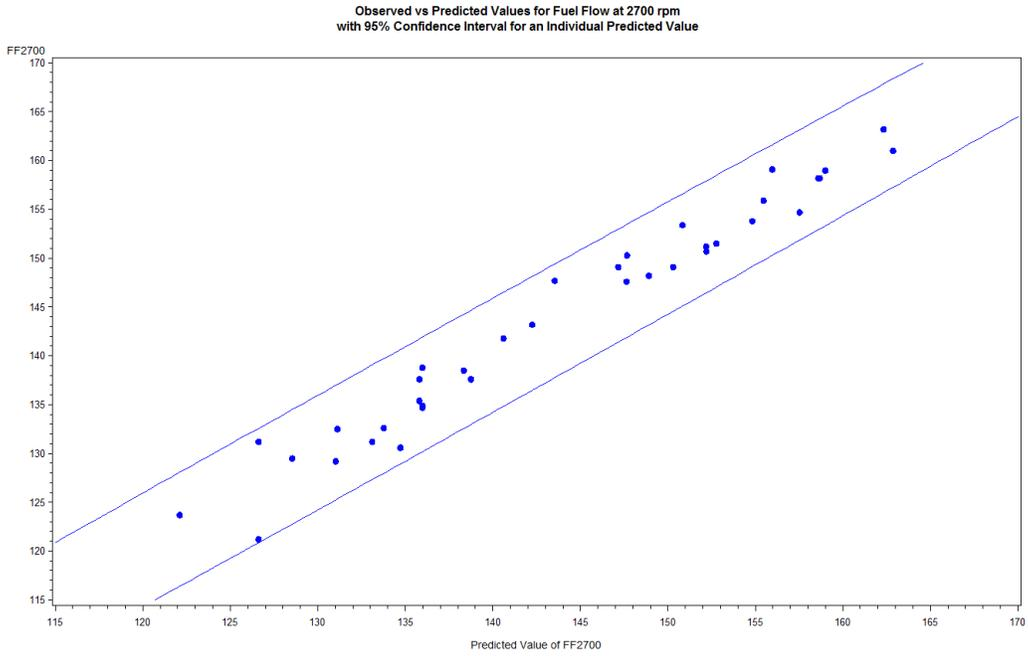
Figure 16 Observed versus Predicted Values for Fuel Flow at 2700 rpm with 95% Confidence Interval for an Individual Predicted Value
