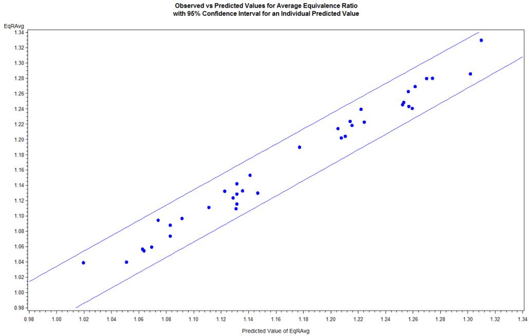
Figure 19 Observed versus Predicted Values for Average Equivalence Ratio with 95% Confidence Interval for an Individual Predicted Value
