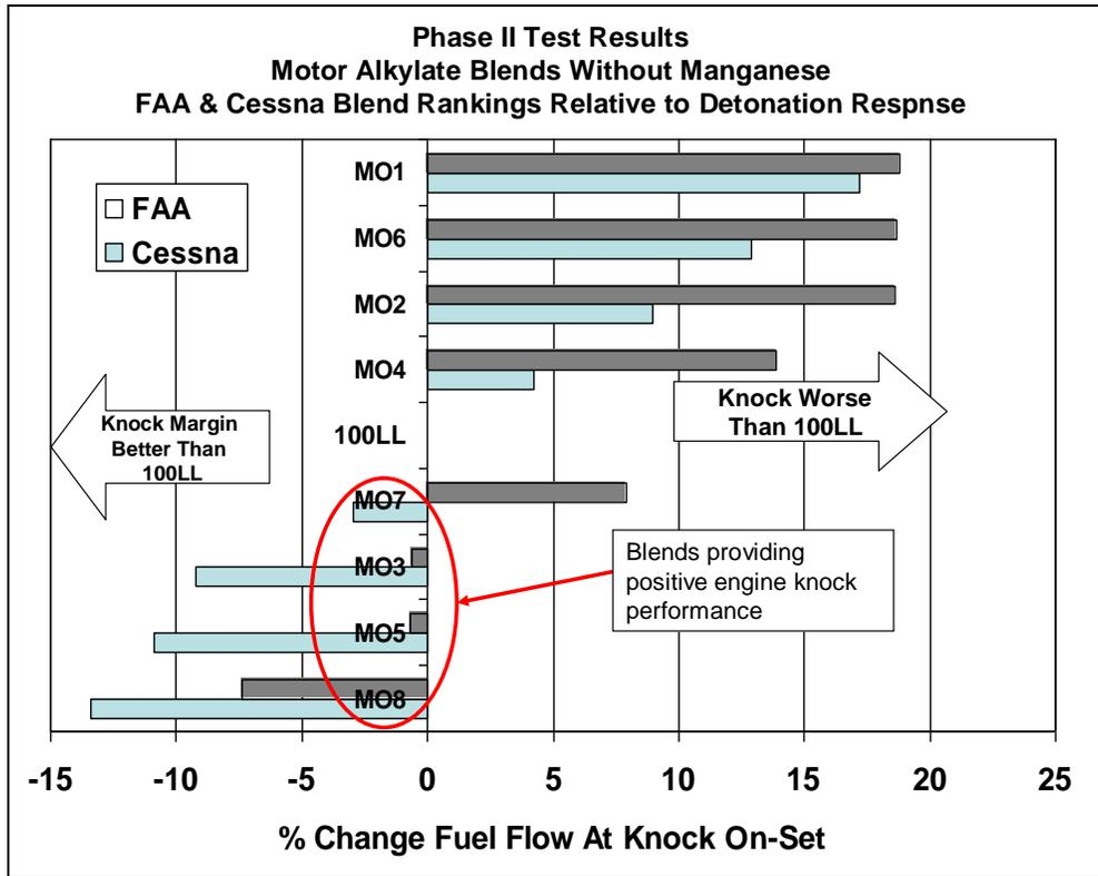
Figure 57.0 – Detonation Ranking of Motor Alkylate Blends W/O MMT
