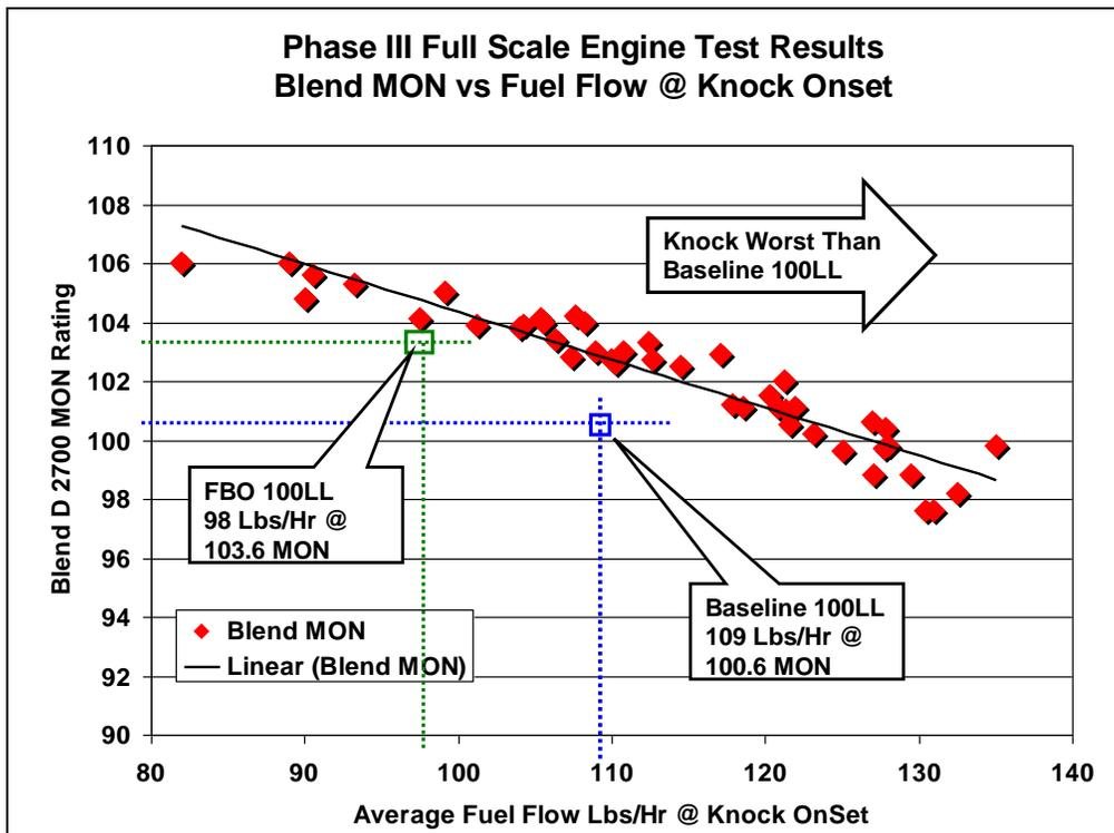
Figure 69.0 – Detonation Performance of Min Spec 100LL & FBO 100LL D 2700 MON Rating vs Avg Fuel Flow At Knock On-Set
