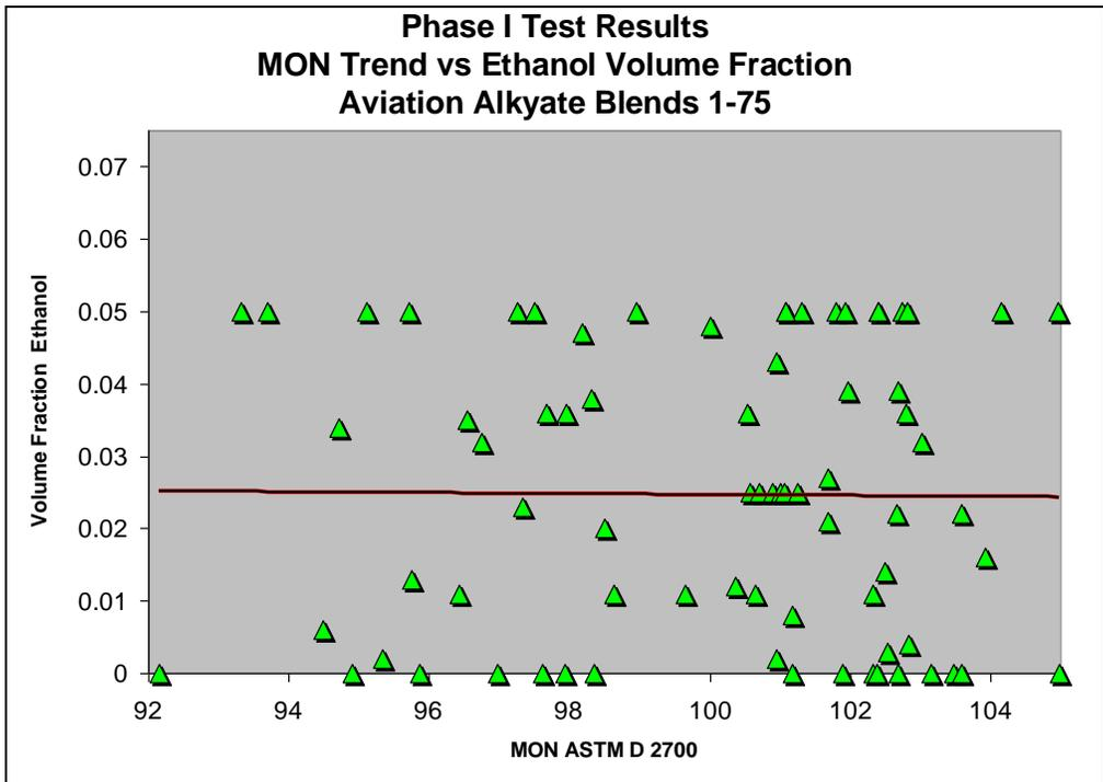
Figure 22.0 - Phase I, MON Trend vs Ethanol Volume Fraction
