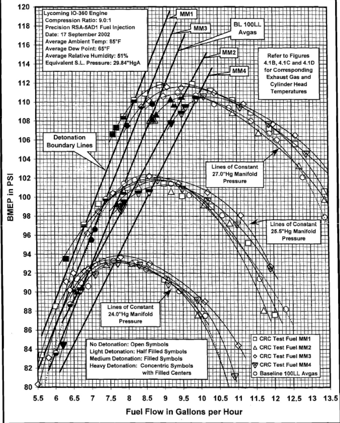
Figure 44.0 – Cessna Knock Test, Mixture Lean Out, Blends MM1-MM4 <sup>(13)</sup>
