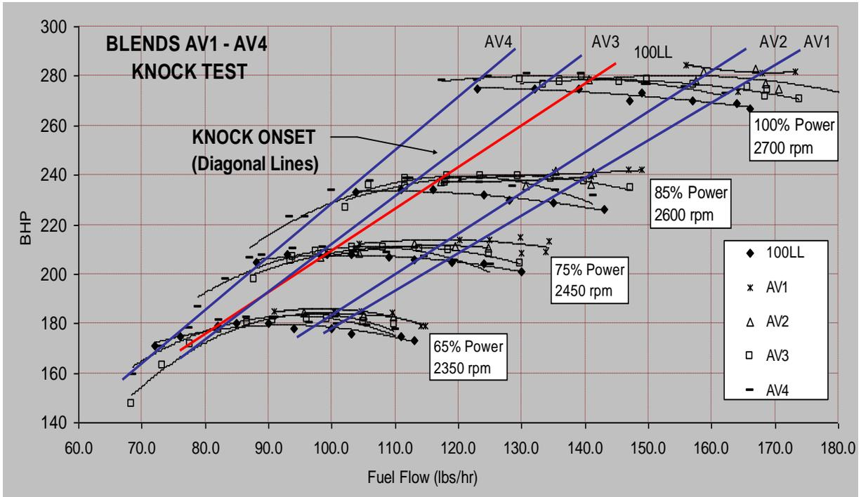
Figure 26.0 – FAA Knock Test, Mixture Lean Out, Blends AV1-AV4 <sup>(12)</sup>
