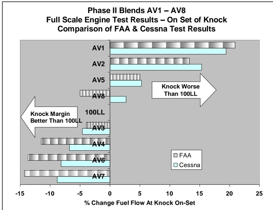
Figure 50.0 – Comparison FAA & Cessna Results AV1-AV8
