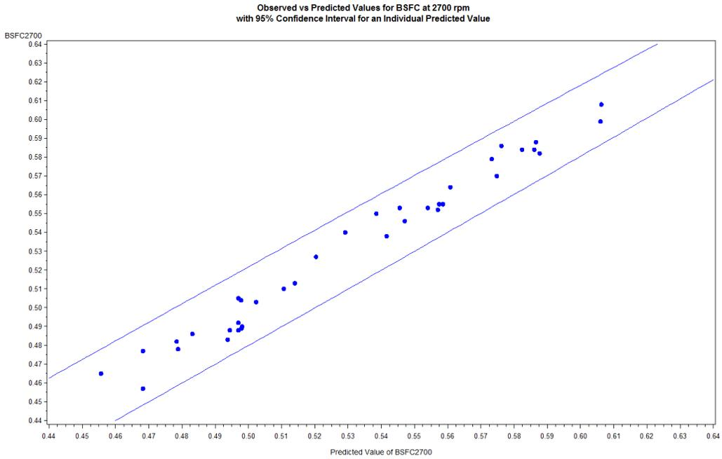
Figure 46 Observed versus Predicted Values for BSFC at 2700 rpm with 95% Confidence Interval for an Individual Predicted Value
