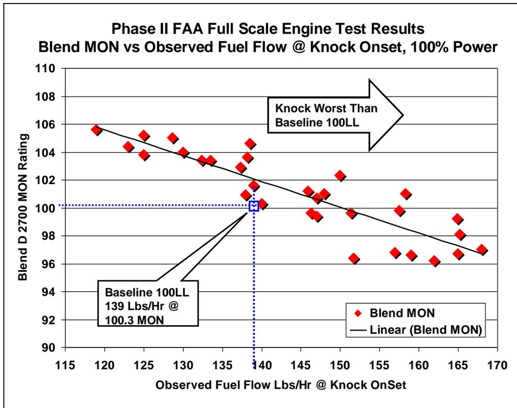
Figure 54.0 – Phase II Blend MON vs FAA Knock Onset Fuel Flow <sup>(12)</sup>
