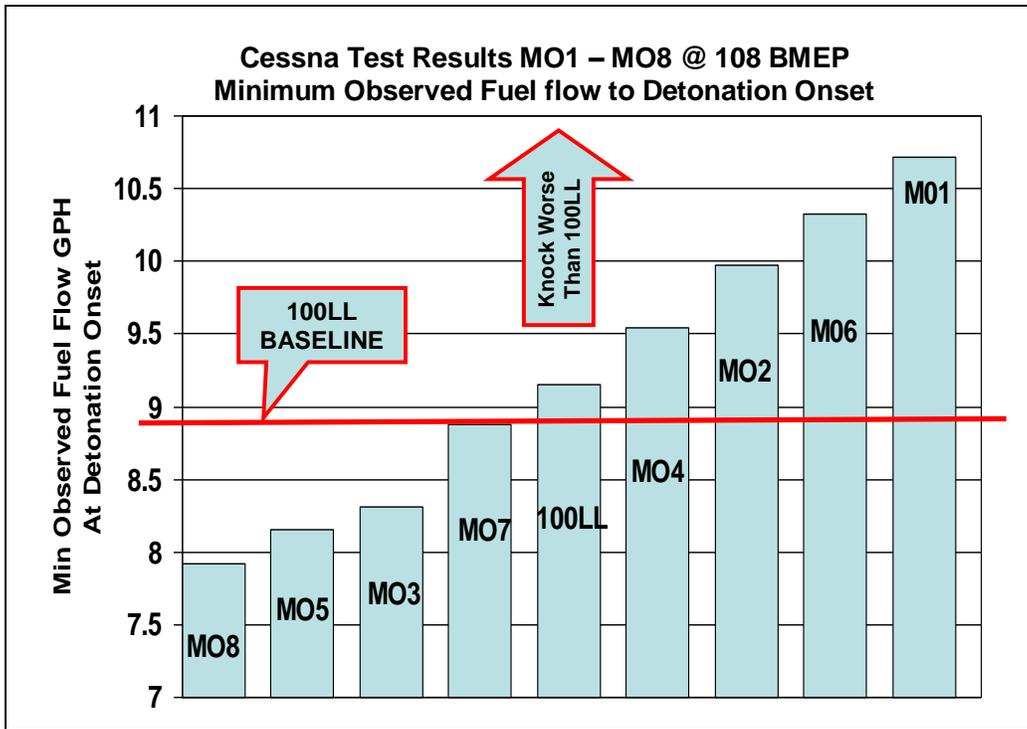
Figure 48.0 – Relative Ranking Blends MO1 – MO8, Cessna Test
