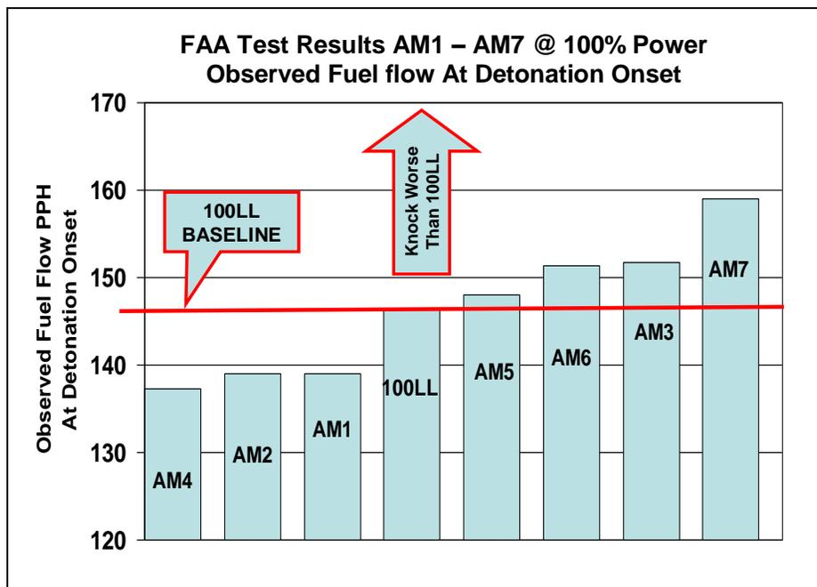
Figure 35.0 – Relative Ranking Blends AM1 – AM7, FAA Test
