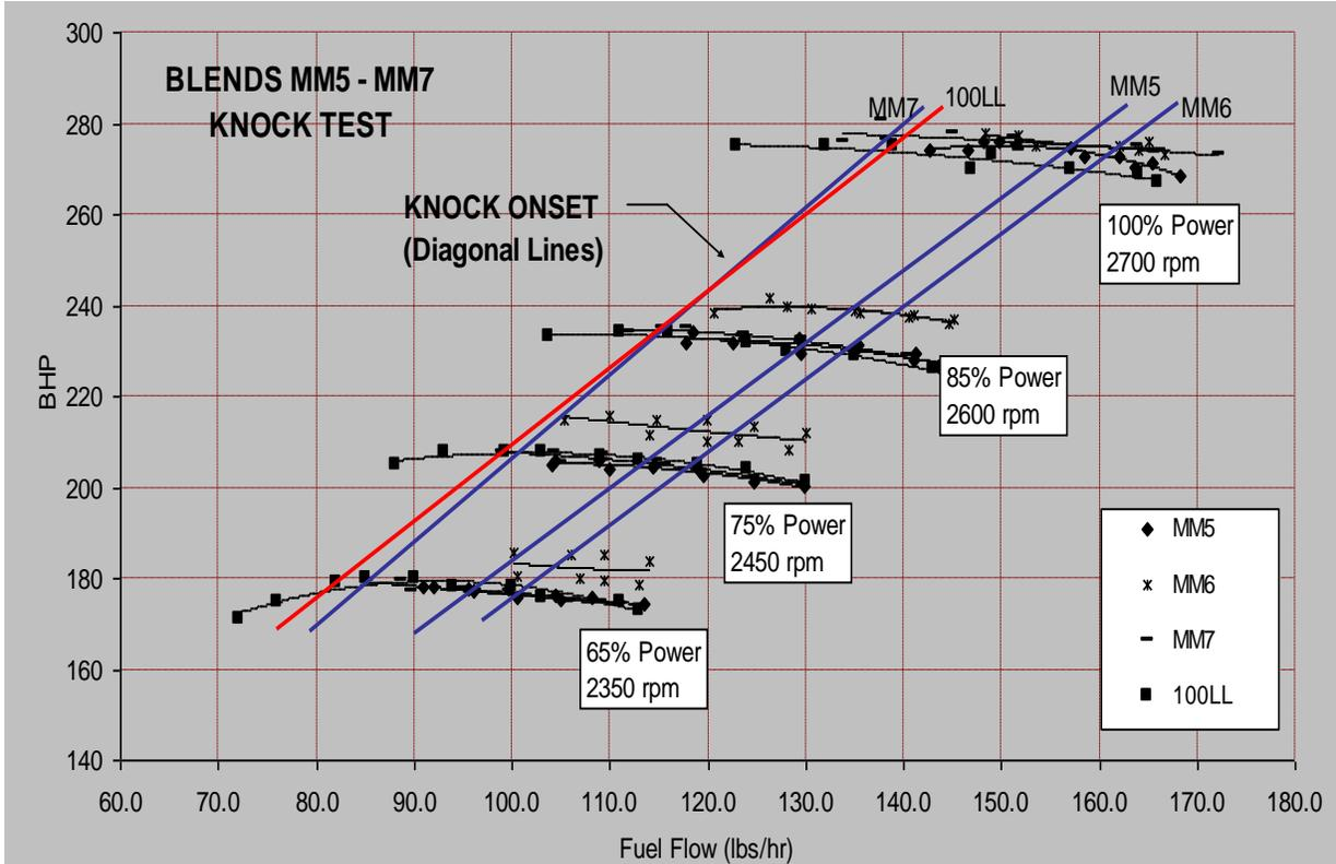
Figure 33.0 – FAA Knock Test, Blends MM5 – MM7 <sup>(12)</sup>
