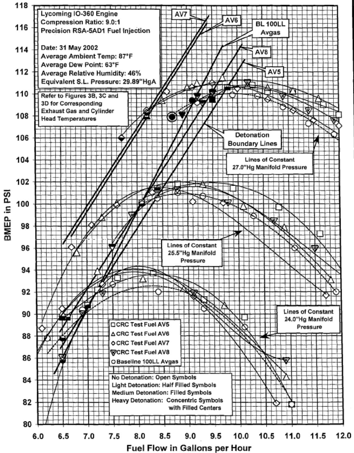
Figure 39.0 – Cessna Knock Test, Mixture Lean Out, Blends AV5-AV8 <sup>(13)</sup>
