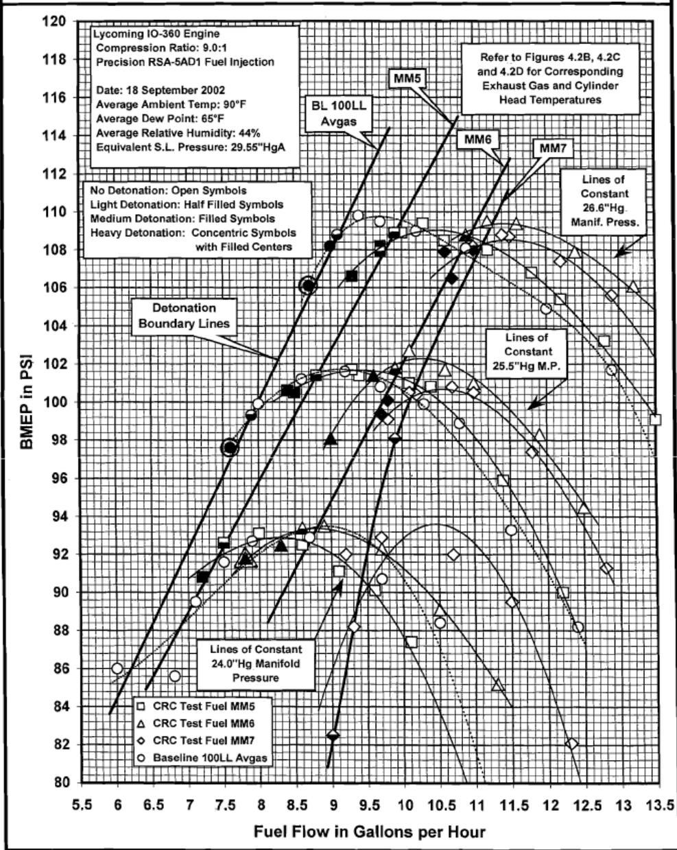
Figure 45.0 – Cessna Knock Test, Mixture Lean Out, Blends MM5-MM7 <sup>(13)</sup>
