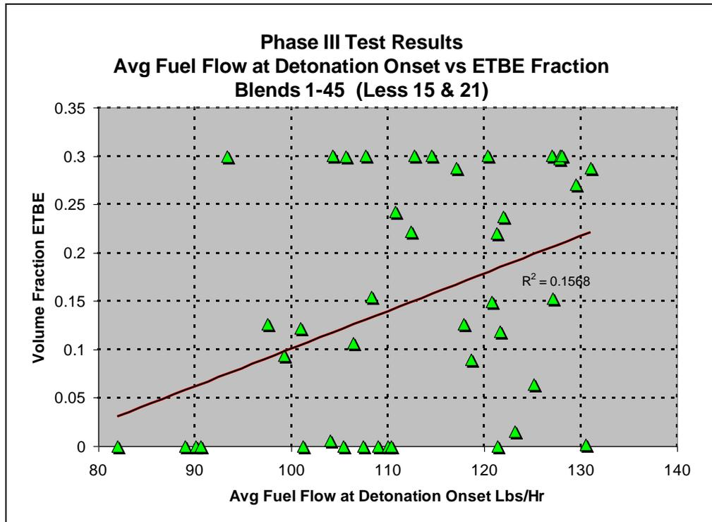
Figure 67.0 – Effect of ETBE on Knock Onset Avg Fuel Flow
