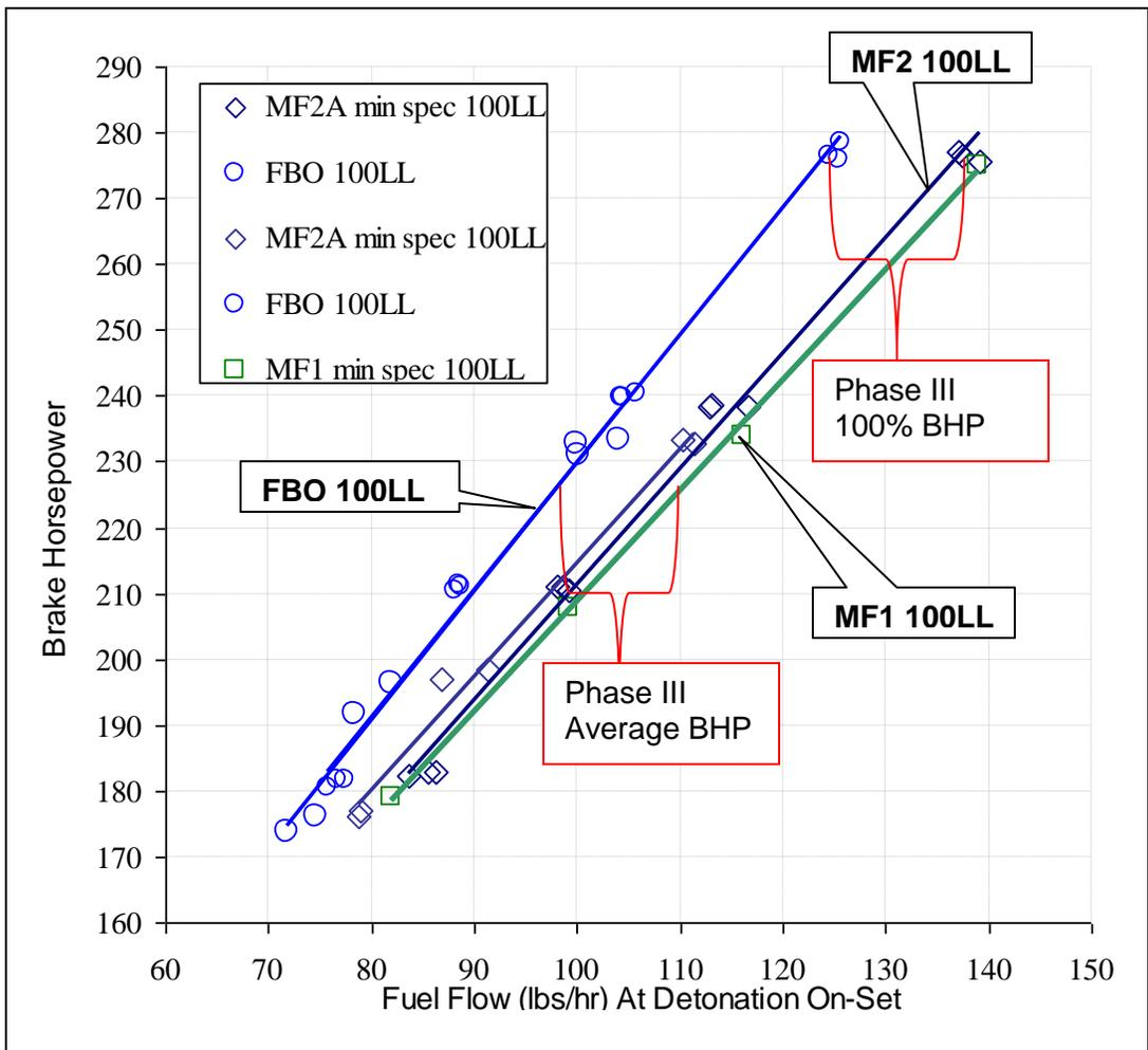
Figure 68.0 – Detonation Performance of Min Spec 100LL & FBO 100LL<sup>(15)</sup>
