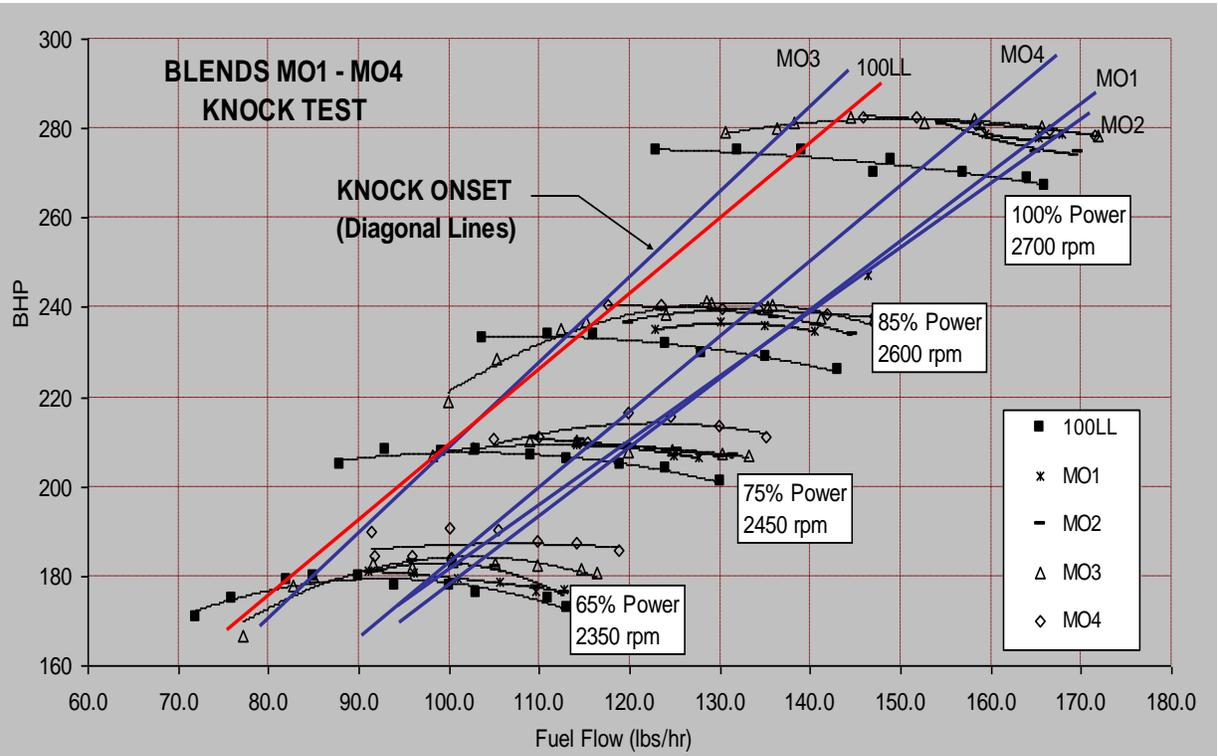
Figure 30.0 – FAA Knock Test, Blends MO1 – MO4 <sup>(12)</sup>
