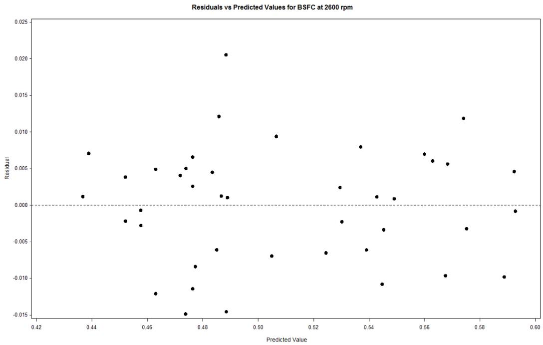
Figure 44 Residual versus Predicted Values for BSFC at 2600 rpm
