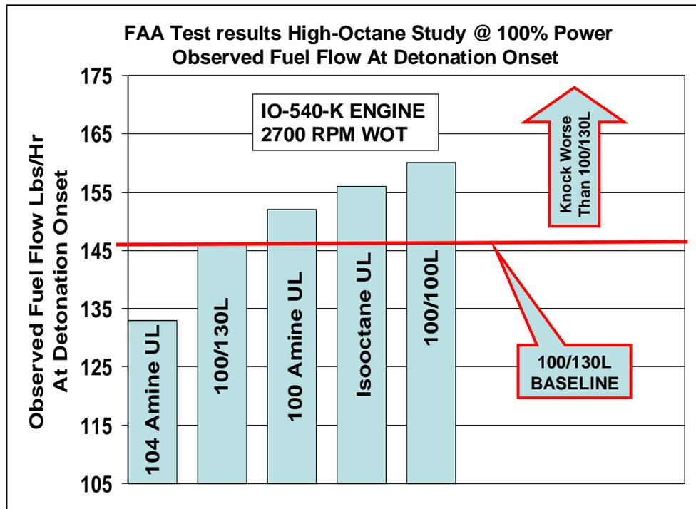
Figure 73.0 – Effect of High-Octane Fuels – “Fuel Flow at Detonation Onset”
