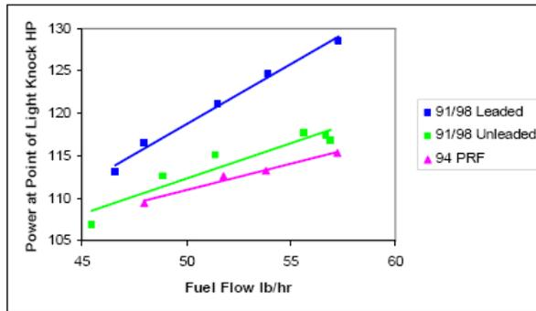
Figure 9: A Comparison of Detonation Limited Power Output versus Fuel Flow for 94 PRF, Leaded and Unleaded AVGAS at 2450 RPM
