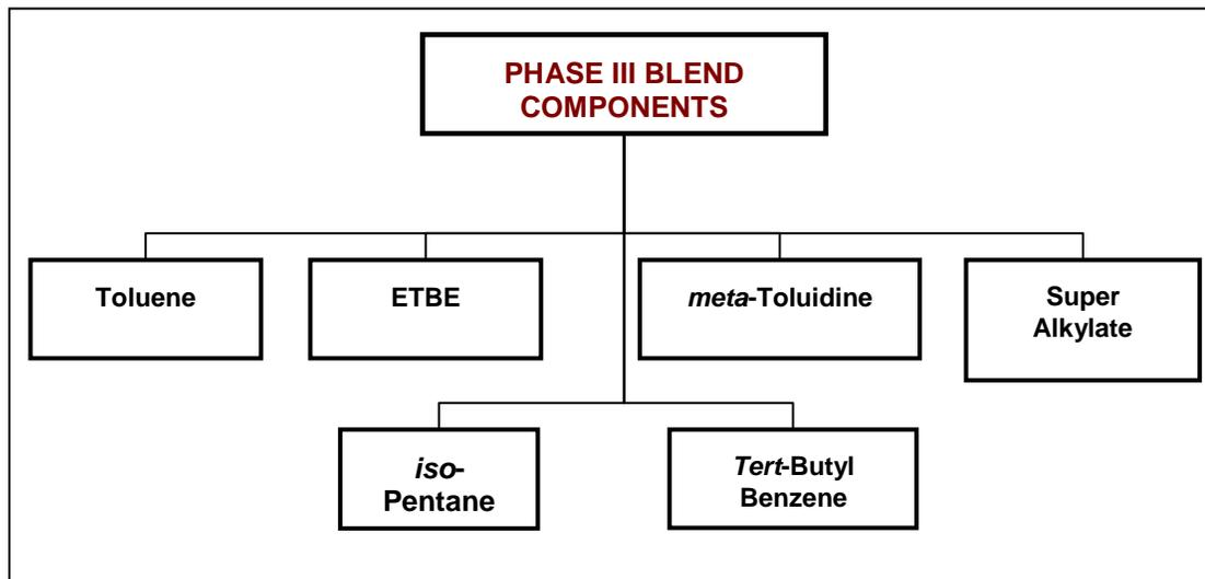
Figure 58.0 – Phase III Blend Components
