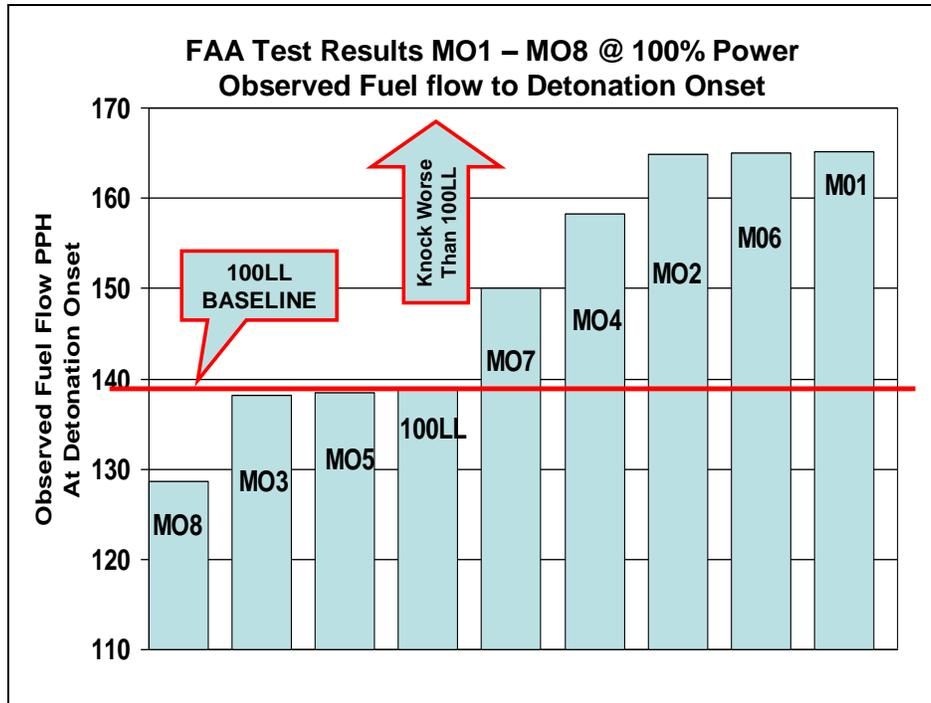
Figure 36.0 – Relative Ranking Blends MO1 – MO8, FAA Test
