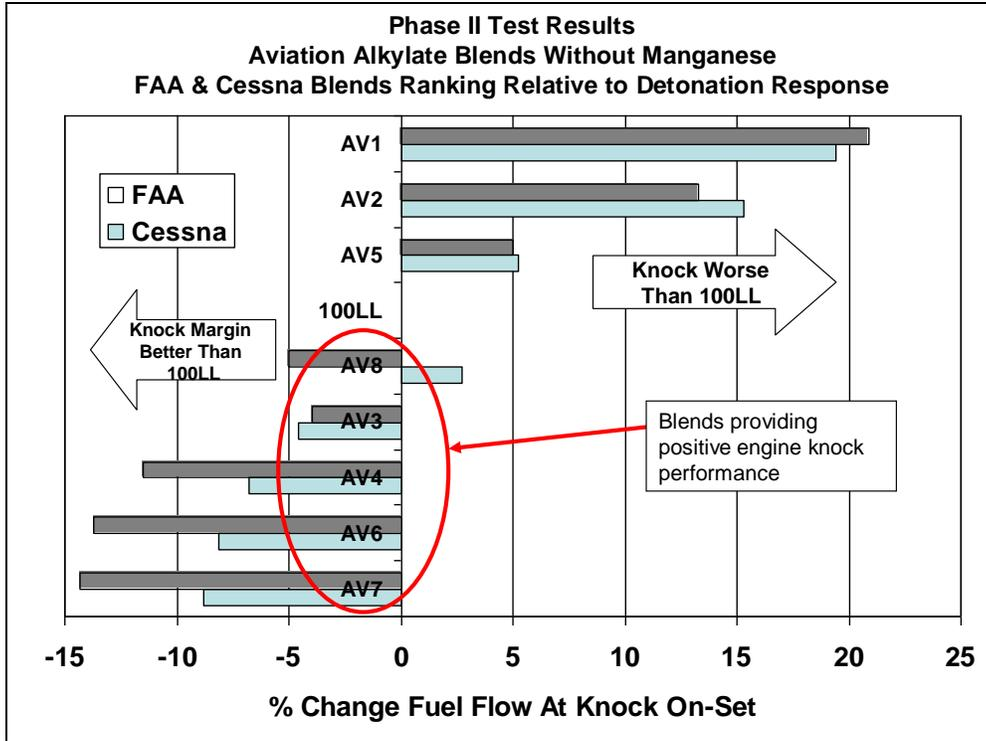
Figure 55.0 – Detonation Ranking of Av Alkylate Blends W/O MMT
