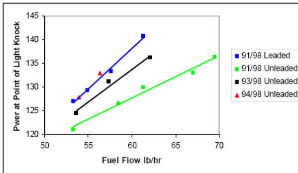
Figure 6: A Comparison of Detonation Limited Power Output versus Fuel Flow for Leaded and Unleaded AVGAS at 2700 RPM
