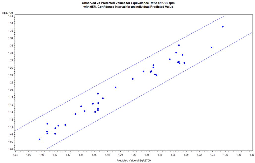
Figure 31 Observed versus Predicted Values for Equivalence Ratio at 2700 rpm with 95% Confidence Interval for an Individual Predicted Value
