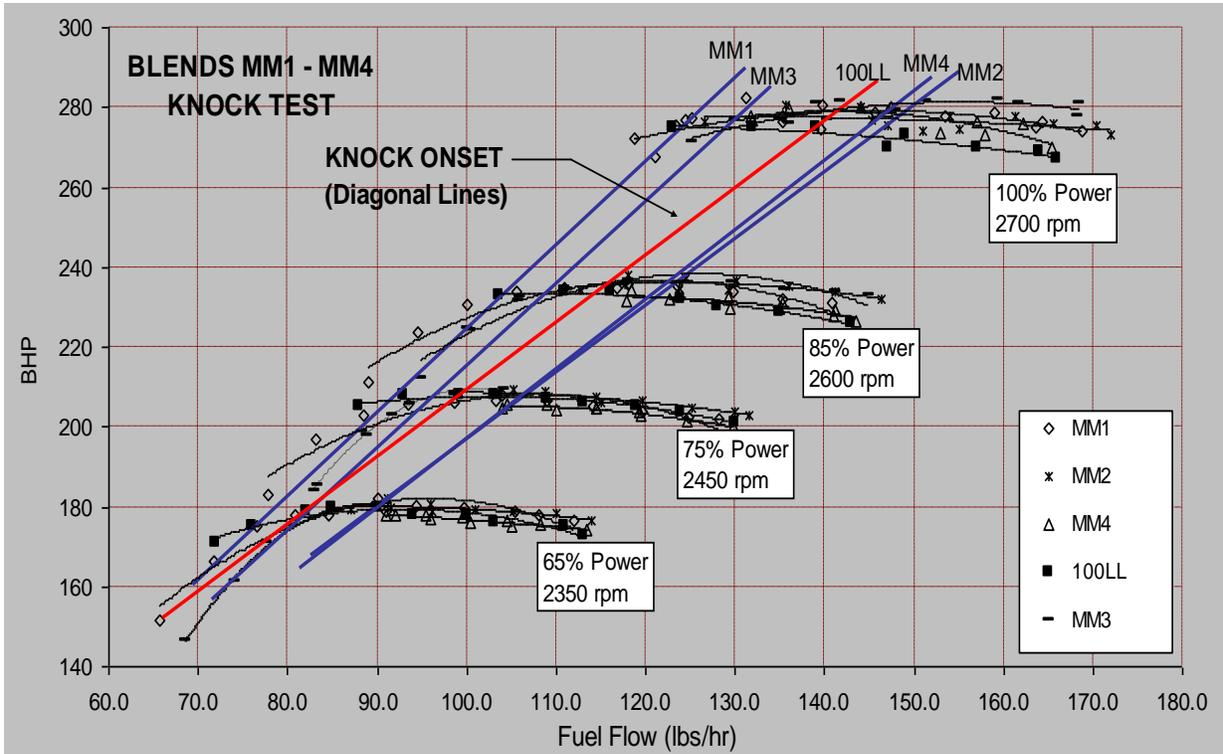
Figure 32.0 – FAA Knock Test, Blends MM1 – MM4 <sup>(12)</sup>
