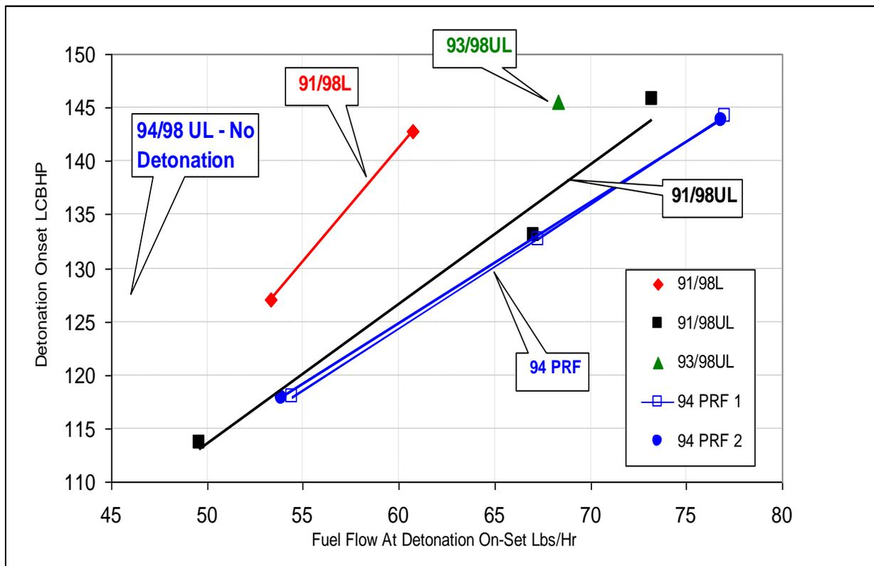
Figure 74.0 – Mid-Octane Study, “Fuel Flow at Detonation Onset”<sup>(14)</sup>
