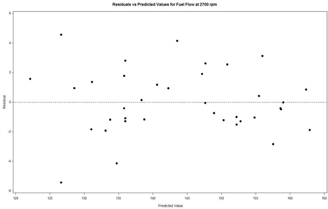
Figure 17 Residual versus Predicted Values for Fuel Flow at 2700 rpm
