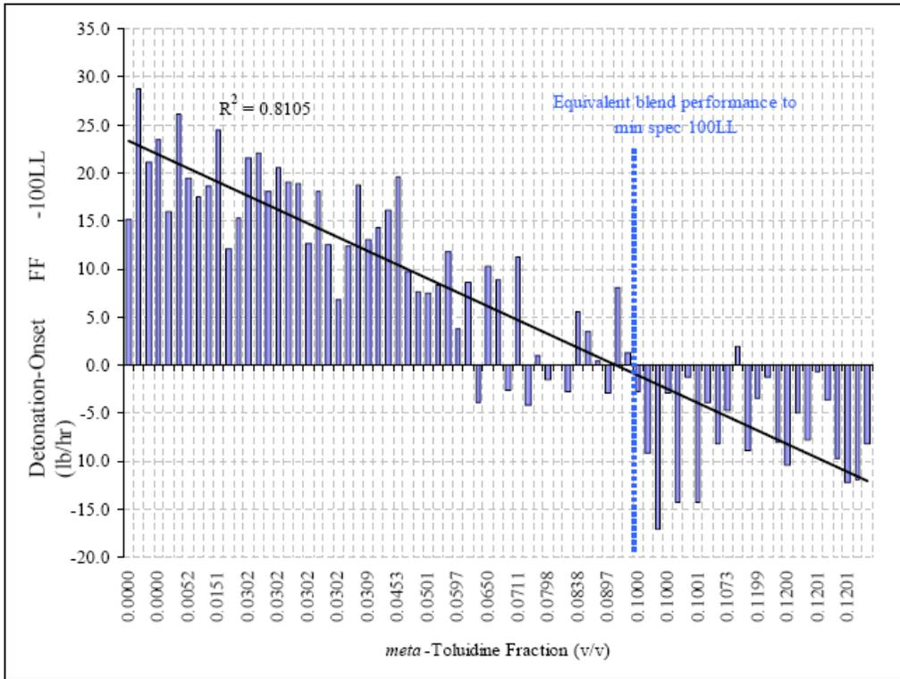
Figure 63.0 – Effect of meta-Toluidine on Blend Detonation Onset Fuel Flow For all 77 Phase II & Phase III Blends<sup>(15)</sup>
