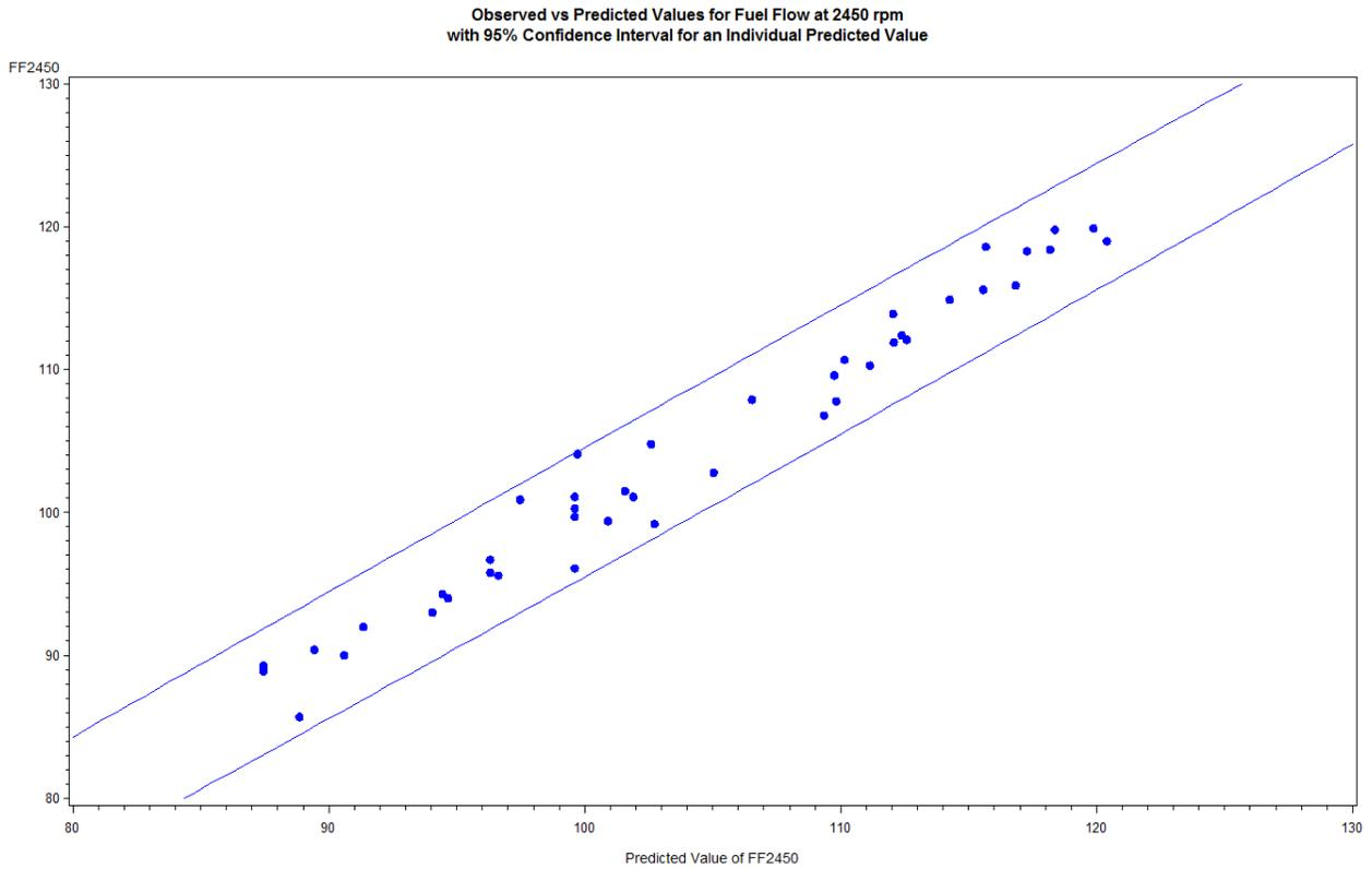
Figure 10 Observed versus Predicted Values for Fuel Flow at 2450 rpm with 95% Confidence Interval for an Individual Predicted Value
