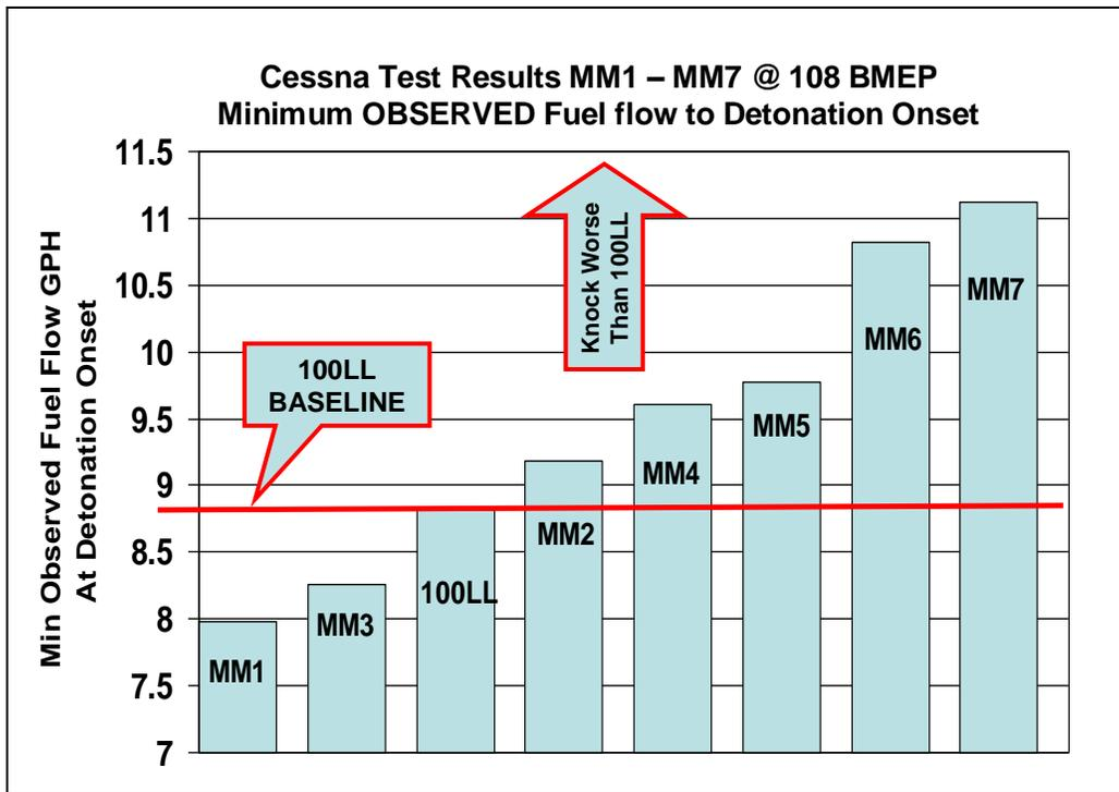
Figure 49.0 – Relative Ranking Blends MM1 – MM7, Cessna Test
