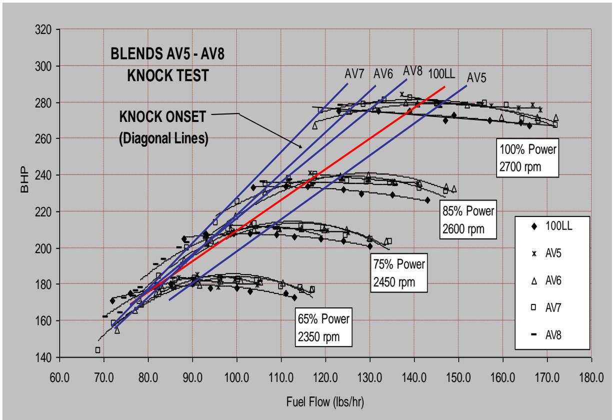
Figure 27.0 – FAA Knock Test, Mixture Lean Out, Blends AV5-AV8 <sup>(12)</sup>
