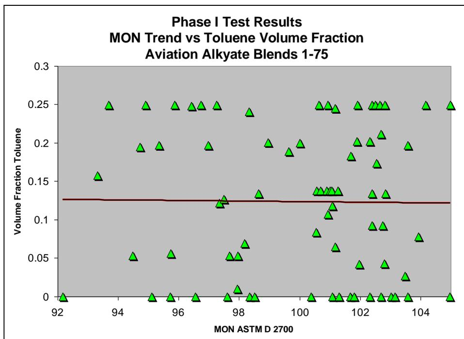
Figure 23.0 - Phase I, MON Trend vs Toluene Volume Fraction
