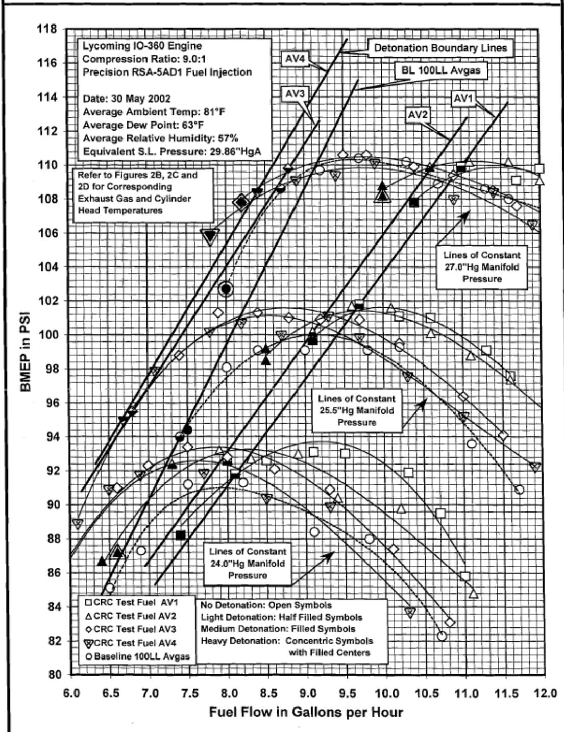
Figure 38.0 – Cessna Knock Test, Mixture Lean Out, Blends AV1-AV4 <sup>(13)</sup>
