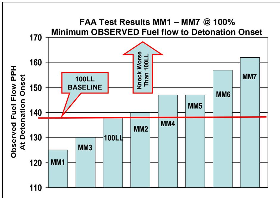
Figure 37.0 – Relative Ranking Blends MM1 – MM7, FAA Test
