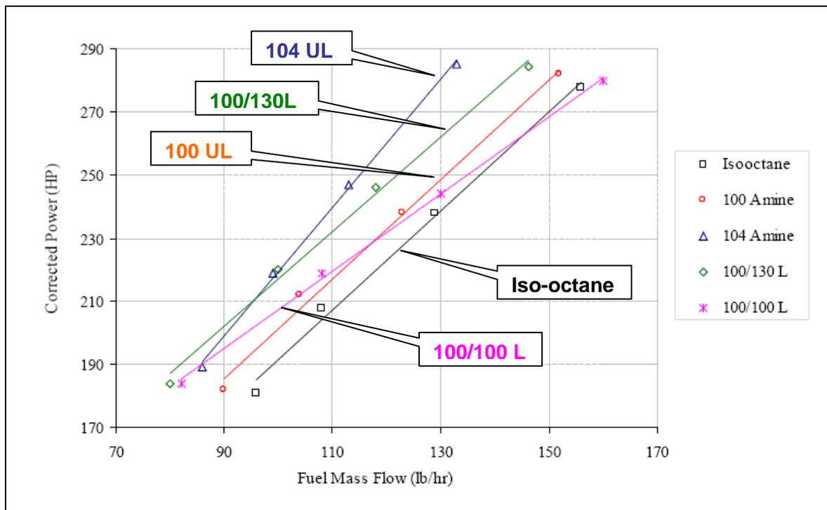
Figure 72.0 – High-Octane Study, “Fuel Flow at Detonation Onset”<sup>(14)</sup>
