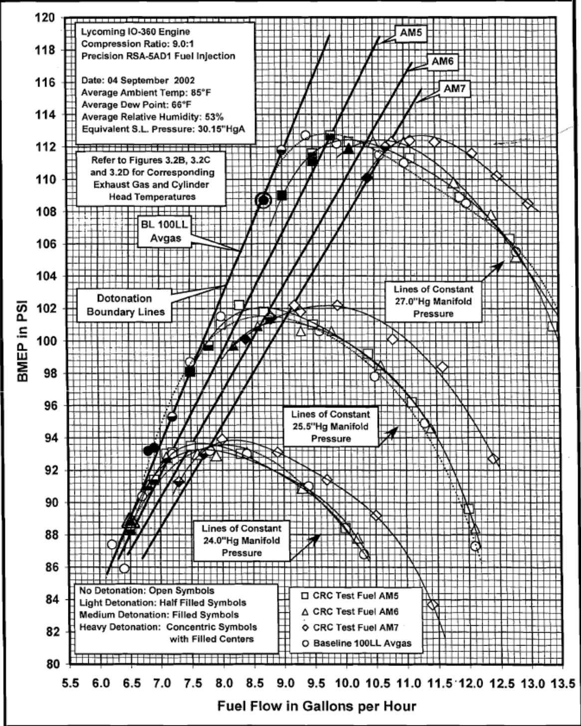
Figure 41.0 – Cessna Knock Test, Mixture Lean Out, Blends AM5-AM7 <sup>(13)</sup>
