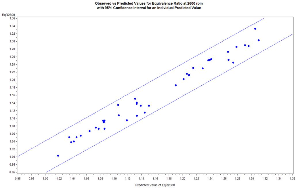
Figure 28 Observed versus Predicted Values for Equivalence Ratio at 2600 rpm with 95% Confidence Interval for an Individual Predicted Value
