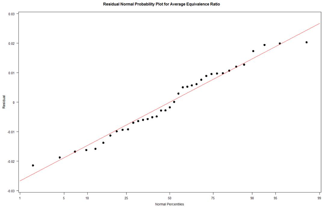
Figure 21 Normal Probability Plot of Average Equivalence Ratio Residuals
