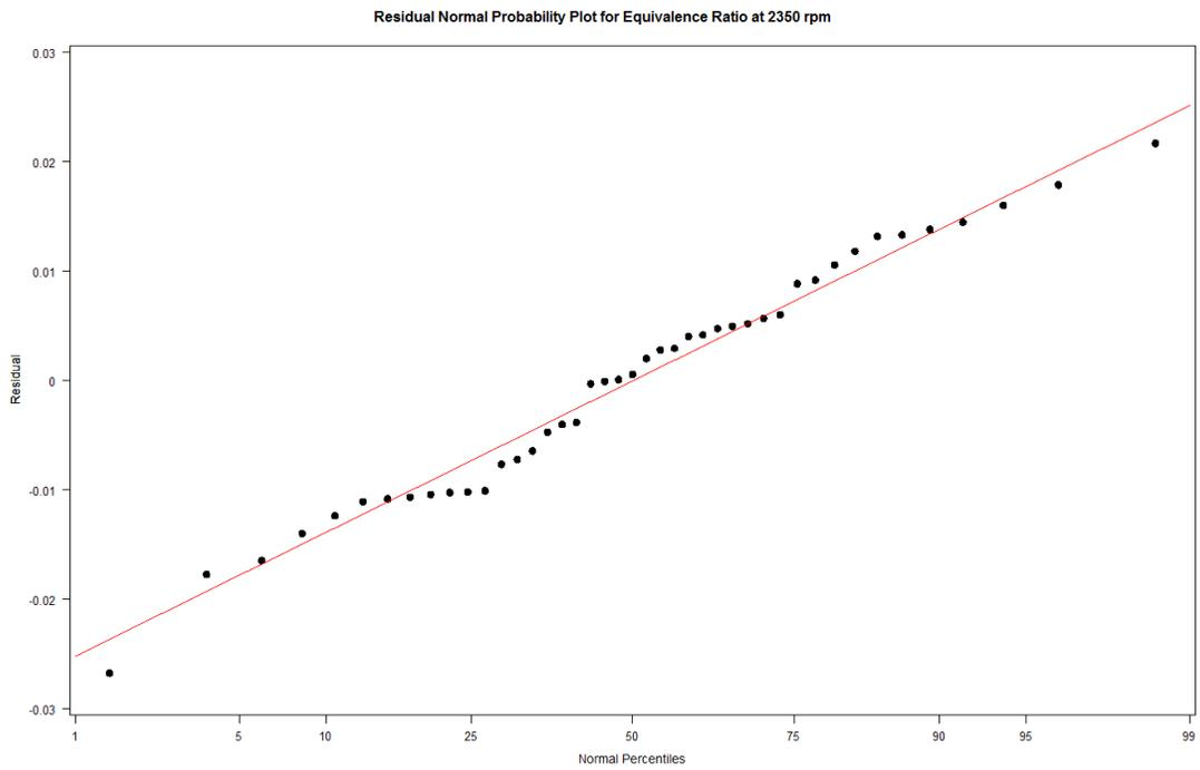
Figure 24 Normal Probability Plot of Equivalence Ratio at 2350 rpm Residuals
