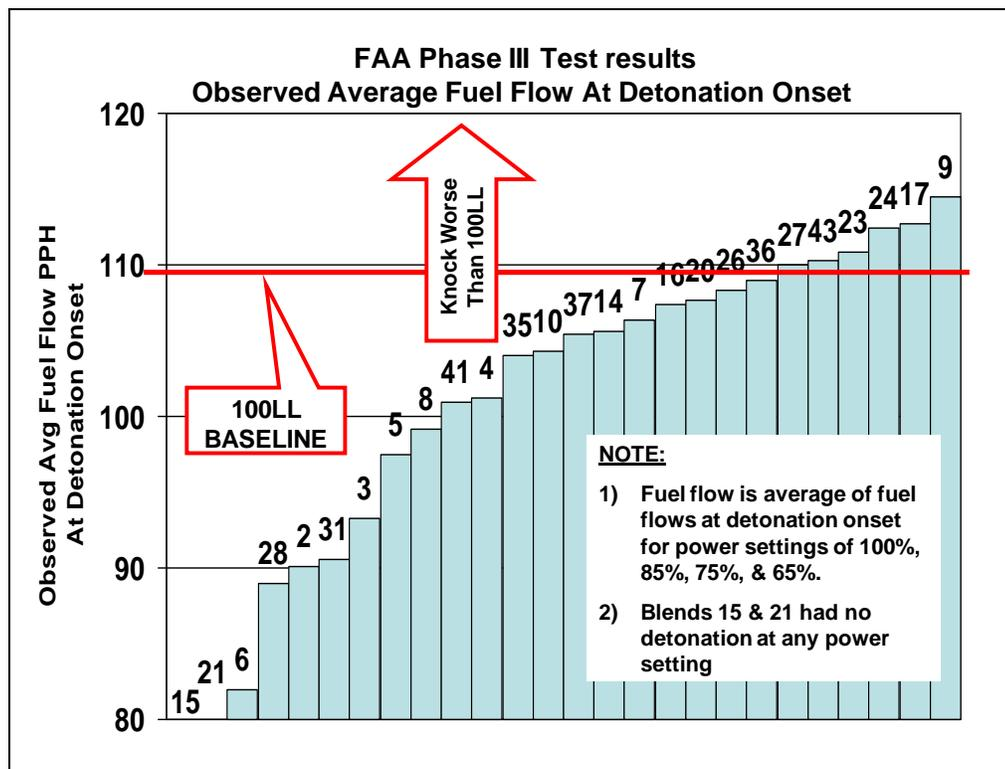
Figure 59.0 – Detonation Ranking of Phase III Blends <sup>(15)</sup>
