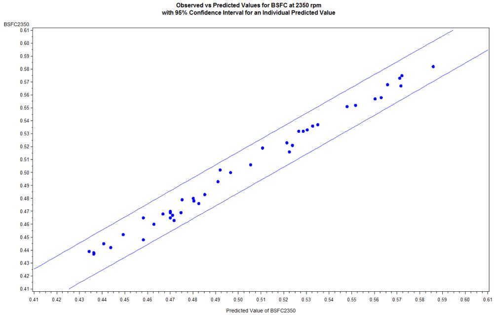
Figure 37 Observed versus Predicted Values for BSFC at 2350 rpm with 95% Confidence Interval for an Individual Predicted Value
