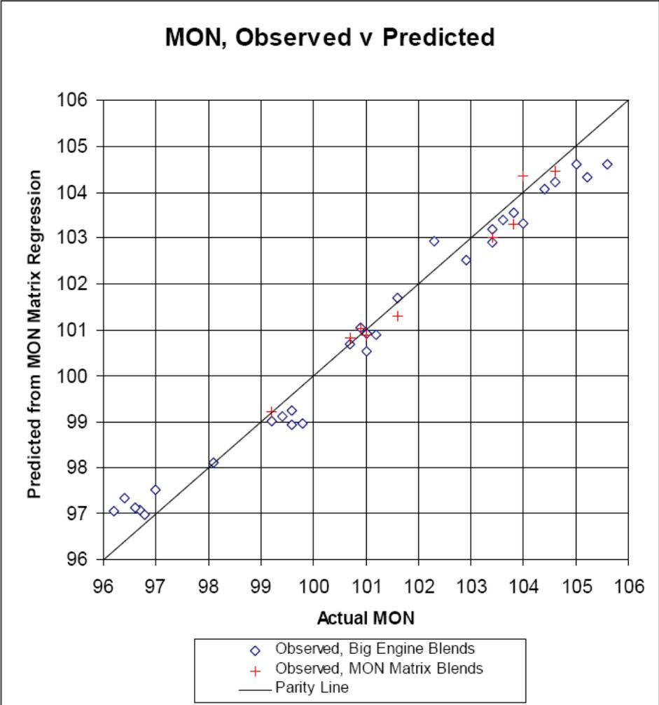
Figure 25.0 – D 2700 MON Observed Test Results vs Predicted MON <sup>(10)</sup>
