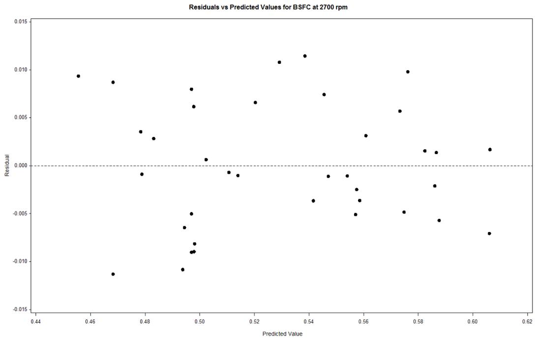
Figure 47 Residual versus Predicted Values for BSFC at 2700 rpm
