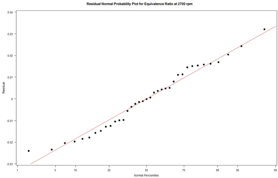
Figure 33 Normal Probability Plot of Equivalence Ratio at 2700 rpm Residuals
