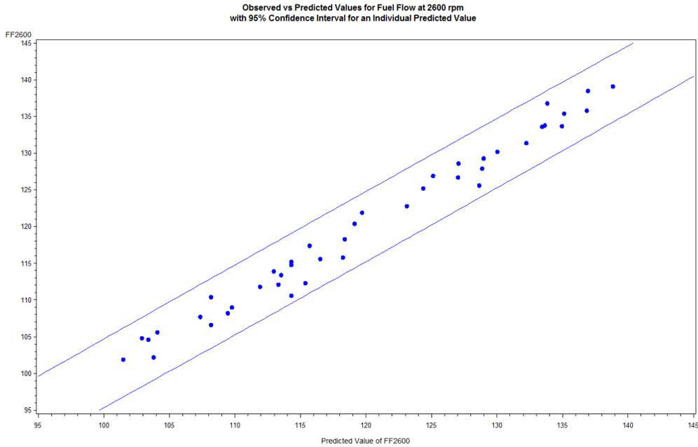
Figure 13 Observed versus Predicted Values for Fuel Flow at 2600 rpm with 95% Confidence Interval for an Individual Predicted Value
