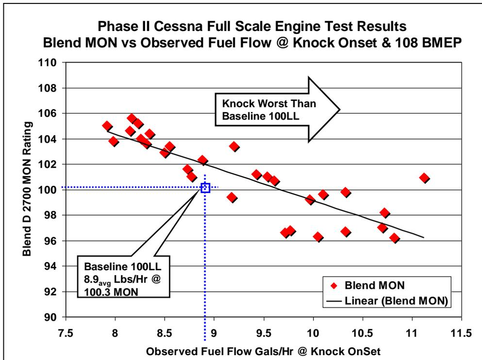
Figure 56.0 – Phase II Blend MON vs Cessna Knock Onset Fuel Flow <sup>(13)</sup>
