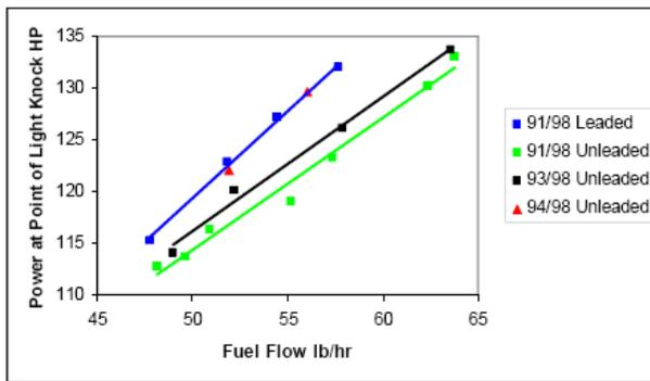
Figure 5: A Comparison of Detonation Limited Power Output versus Fuel Flow for Leaded and Unleaded AVGAS at 2600 RPM
