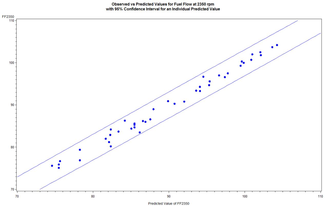
Figure 7 Observed versus Predicted Values for Fuel Flow at 2350 rpm with 95% Confidence Interval for an Individual Predicted Value
