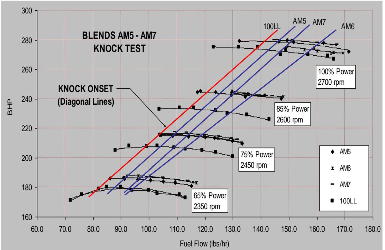
Figure 29.0 – FAA Knock Test, Blends AM5 – AM7 <sup>(12)</sup>
