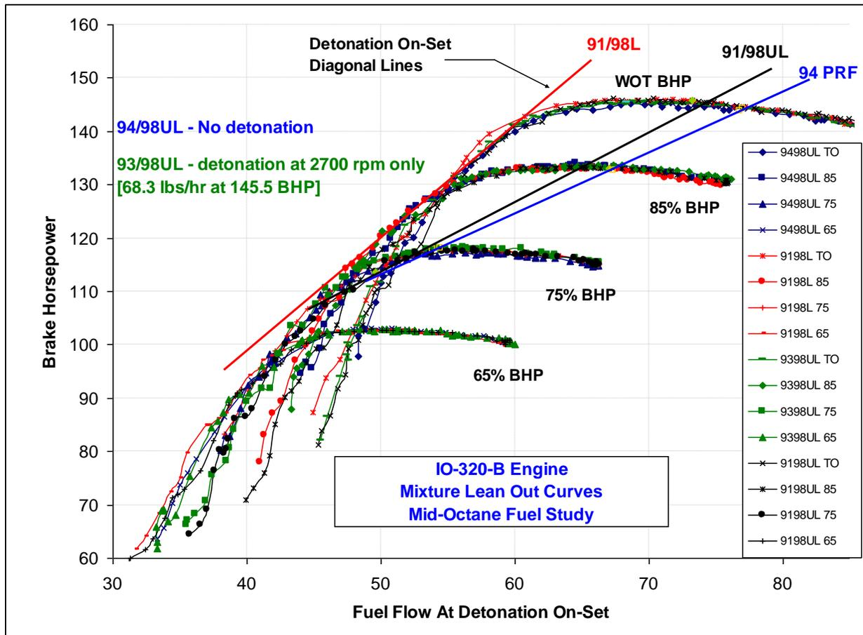
Figure 75.0 – Mid-Octane Fuel Study, Mixture Lean Out Curves <sup>(14)</sup>
