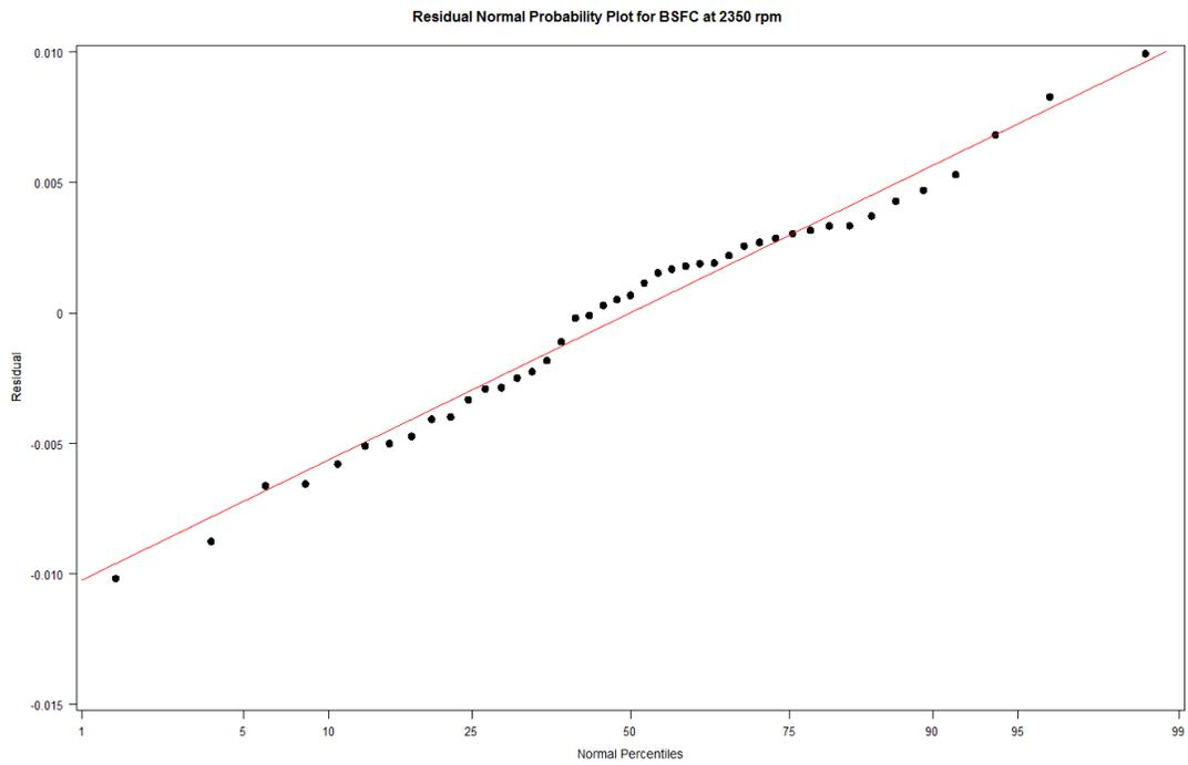
Figure 39 Normal Probability Plot of BSFC at 2350 rpm Residuals
