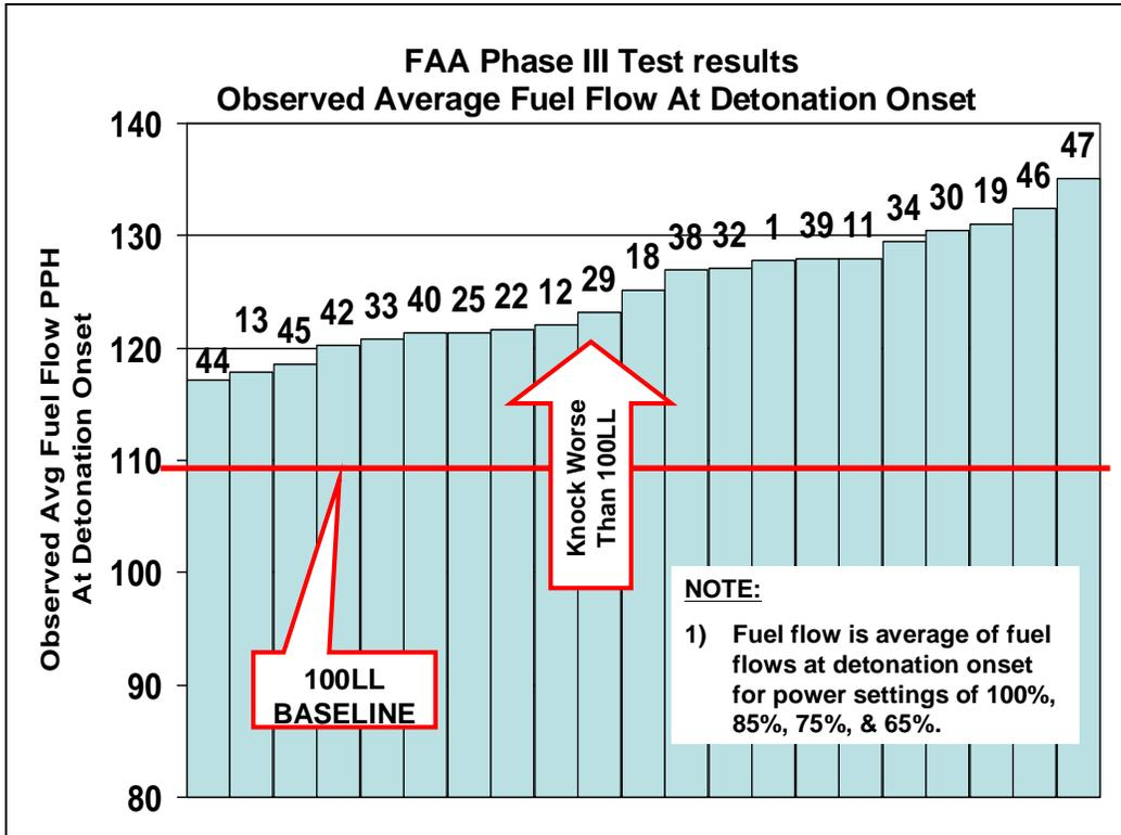
Figure 60.0 – Detonation Ranking of Phase III Blends <sup>(15)</sup>
