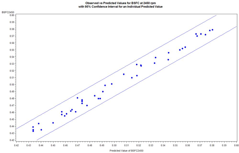
Figure 40 Observed versus Predicted Values for BSFC at 2450 rpm with 95% Confidence Interval for an Individual Predicted Value
