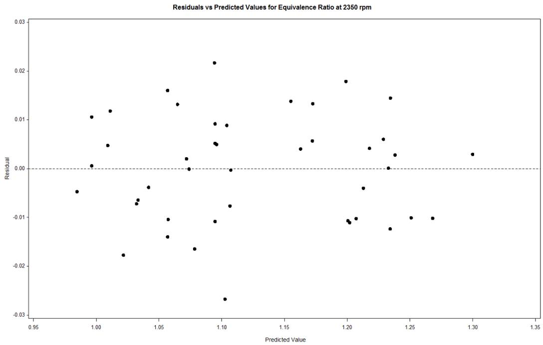
Figure 23 Residual versus Predicted Values for Equivalence Ratio at 2350 rpm
