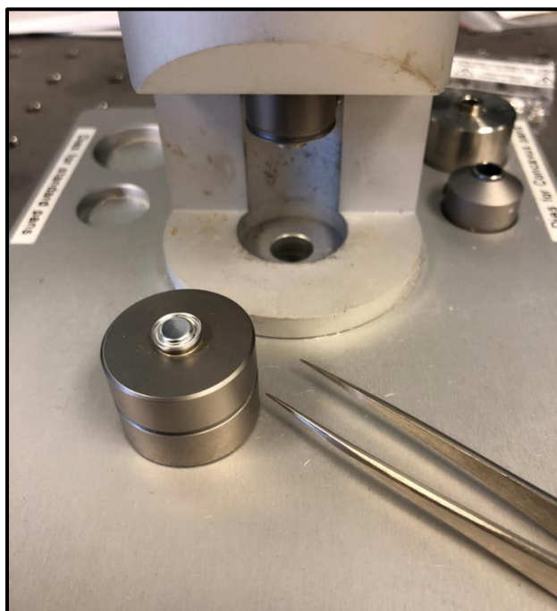
Figure C6: Laser-drilled lid placed on DSC pan.
