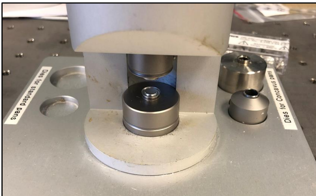
Figure C8: DSC pan/lid after crimping
