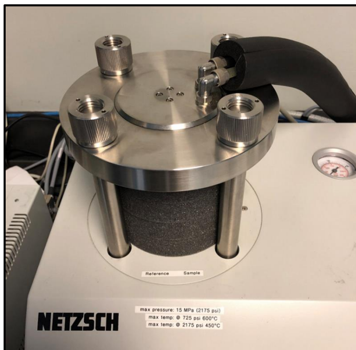
Figure C14: The HPDSC cell, with the SS lid installed and retaining nuts tightened.
