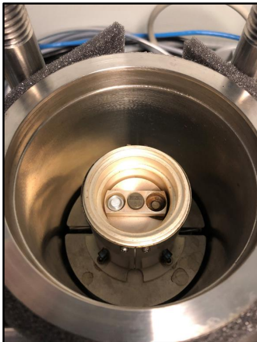
Figure C9: Inside of the HPDSC cell, with an empty pan/lid on the reference side of the HPDSC cell.
