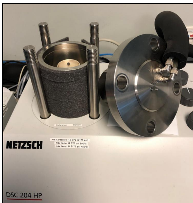
Figure C13: The HPDSC cell, with the water-cooled SS lid.
