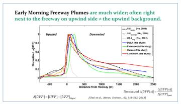
experimental study in which an instrumented mobile platform was used to measure a suite of pollutants while driving on various roadways in northern and southern California. A sophisticated data processing approach was followed to ensure that proper weighting of individual sections of each test run was done and reliable data were obtained. It was determined that about 20 repeat runs conducted under similar meteorological conditions and time of day were required to obtain reasonable averages.
