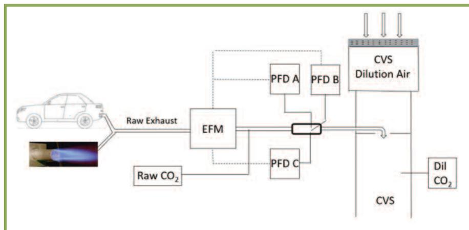
**Figure 2.** Laboratory setup for comparing three PDF systems with the CVS system.
