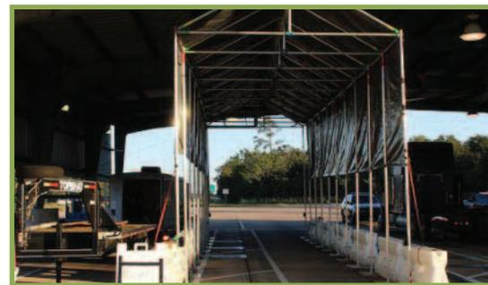
**Figure 3.** The OHMS system samples truck exhaust as trucks start from a stopped position and pass through a test setup.
