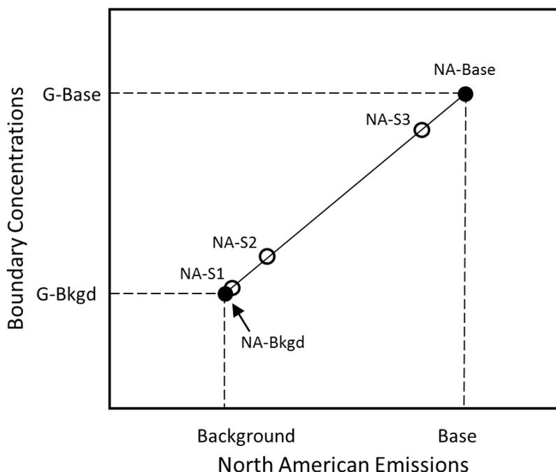
**Figure ES-1.** Schematic representation of the simulations with CAMx for the North American domain. The sensitivities are integrated numerically from the background case to the base case using values of the sensitivities at the points NA-S1, NA-S2, NA-S3 along the path. At these points, the boundary concentrations from GEOS-Chem and the anthropogenic emissions are reduced from those in the base case.
