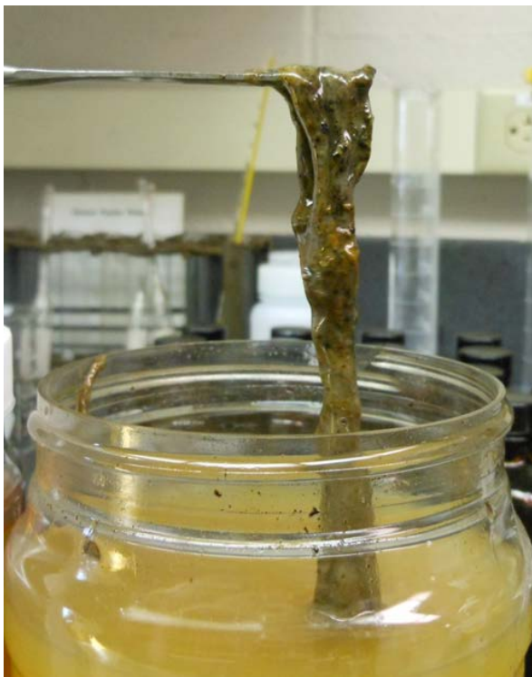
Figure 4: Fuel "rag" layer from diesel bulk storage tank bottom sample 8
