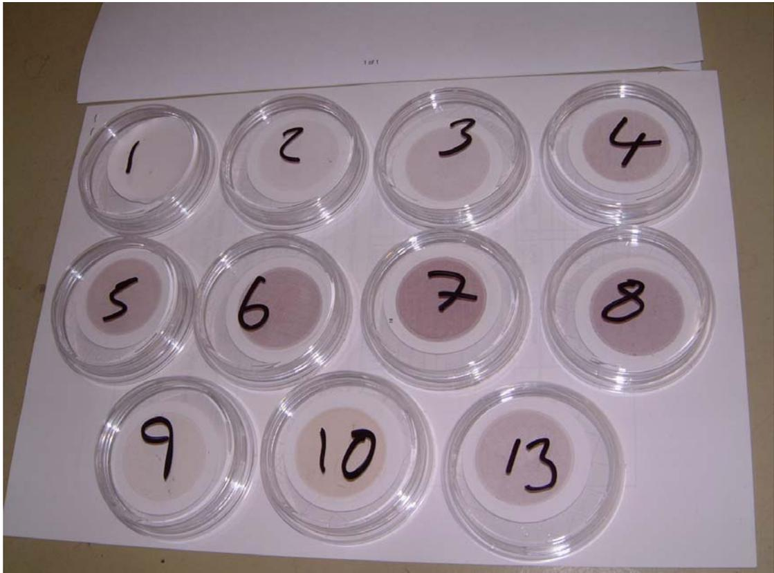
Photograph of the gravimetric pads used in the above particulate assay showing the colorimetric correlation with expected loading.
