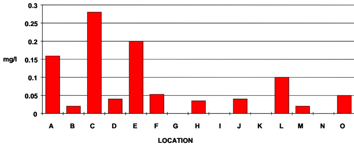
**API/IP Study 1996: Into-plane gravimetric dirt loadings per ASTM D2276
