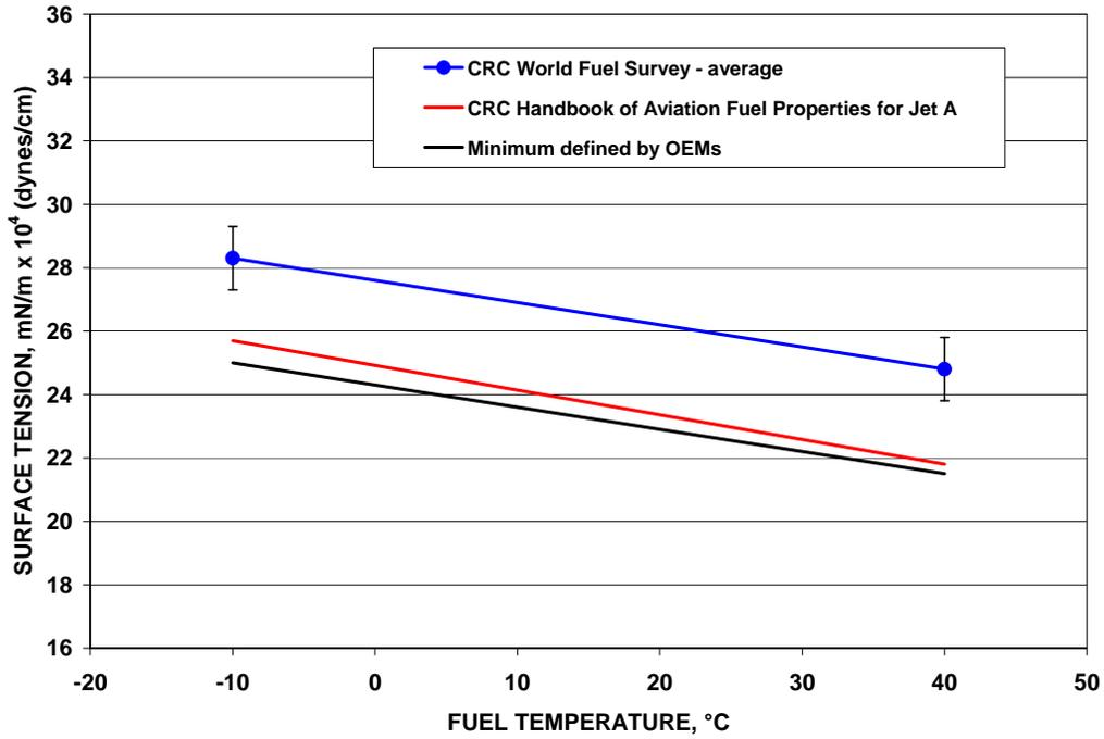
Figure 6. Typical Surface Tension Characteristics of Jet Fuel
