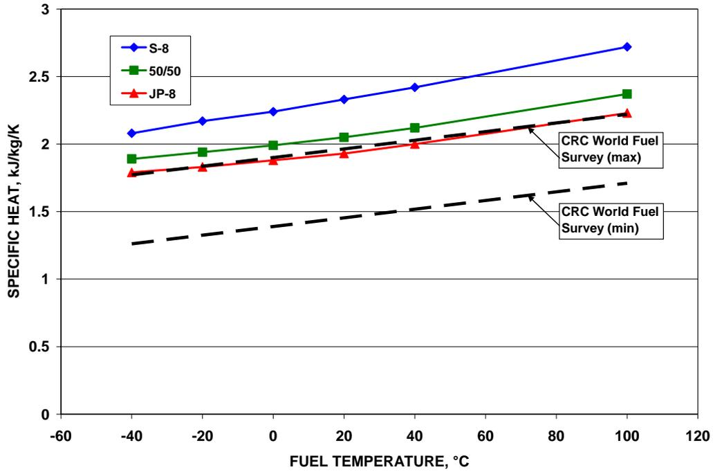
Figure 15. Comparison of Specific Heat
