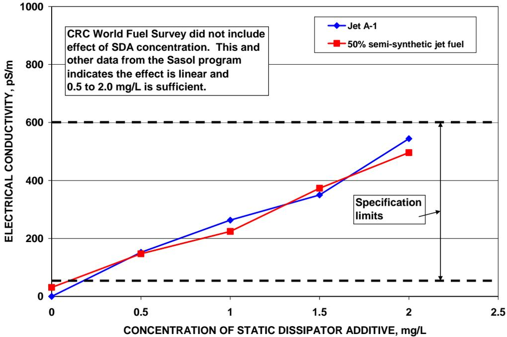
Figure 10. Typical Response to Static Dissipater Additive
