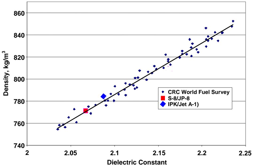
Figure 19. Comparison of Dielectric-Density Characteristics of 50/50 Blends with CRC World Fuel Survey
