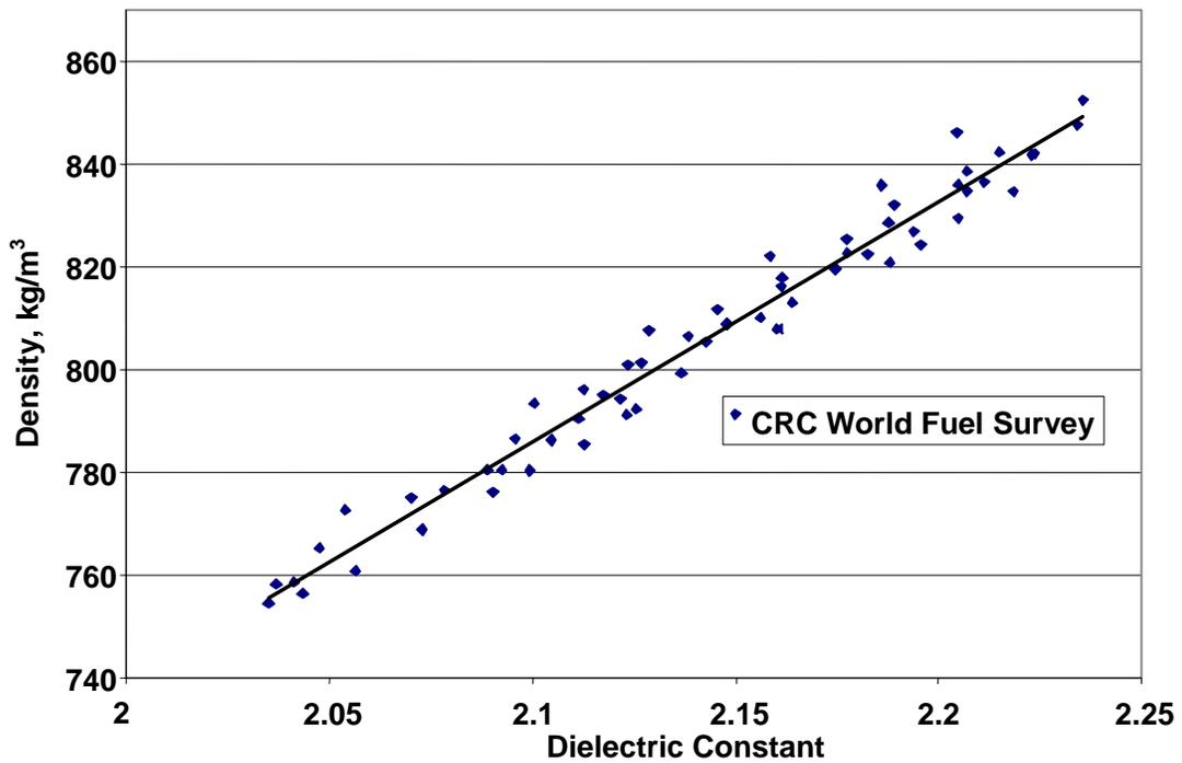
Figure 9. Typical Dielectric-Density Characteristics for Jet Fuel
