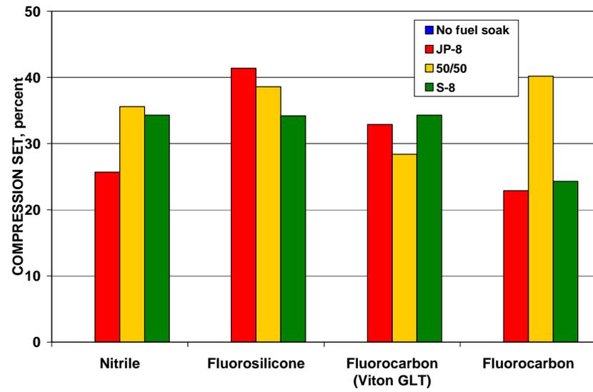
Figure 22. Effect of S-8 on O-Ring Material Properties
