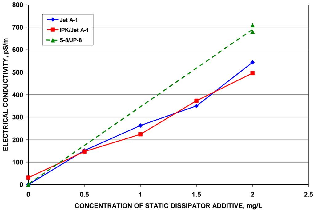
**Figure 21. Effectiveness of Static Dissipator Additive**
