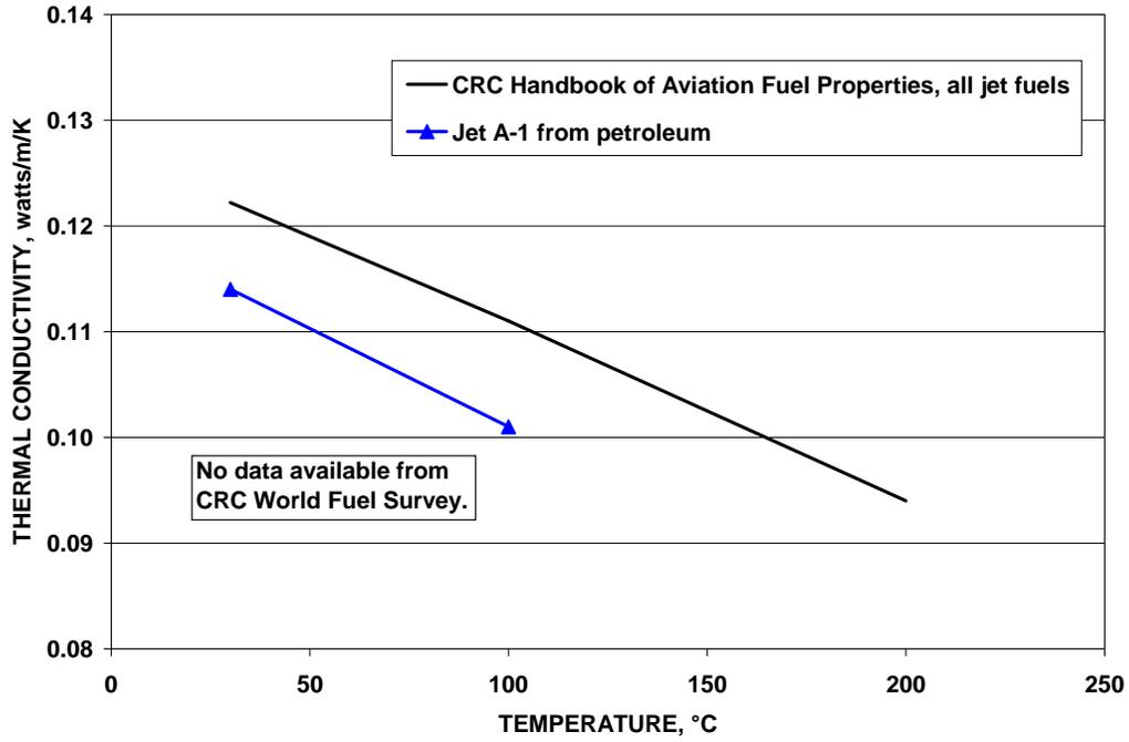
Figure 8. Typical Thermal Conductivity Characteristics of Jet Fuel
