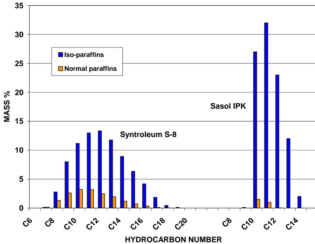
Figure 11. Hydrocarbon Composition of S-8 and IPK
