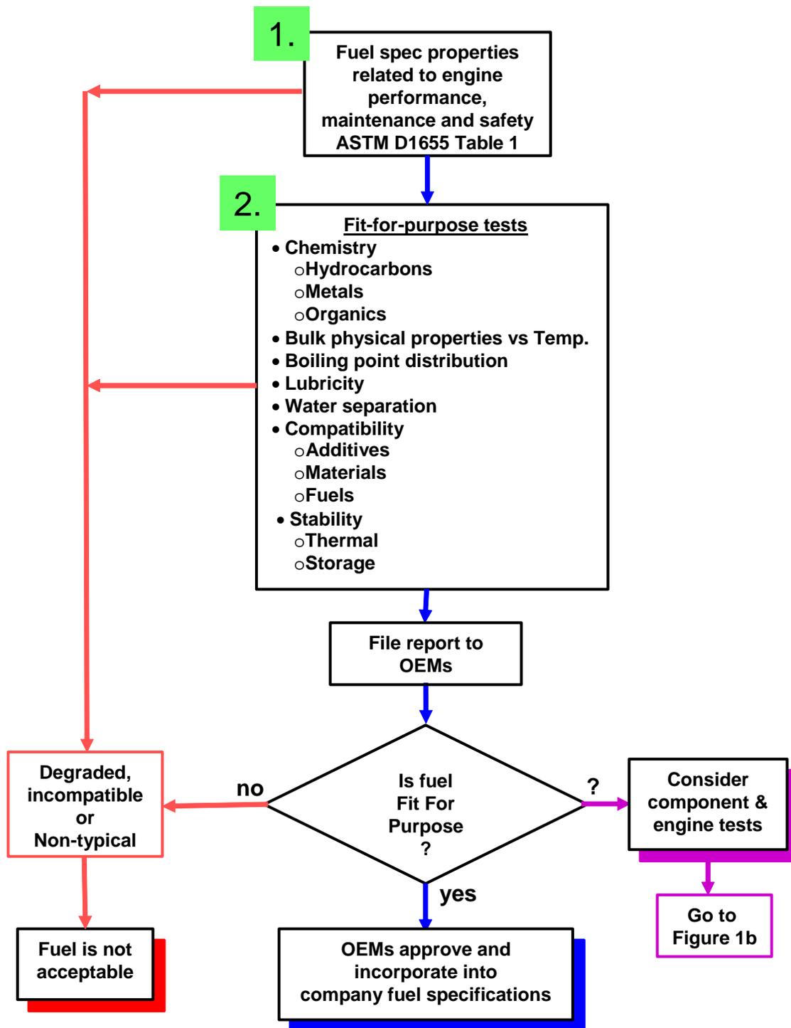
Figure 1a. Approval Process for F-T Kerosenes as Jet Fuel
