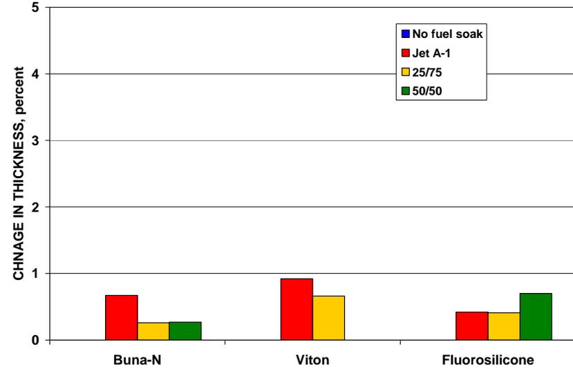
Figure 23. Effect of Sasol IPK on O-Ring Material Properties
