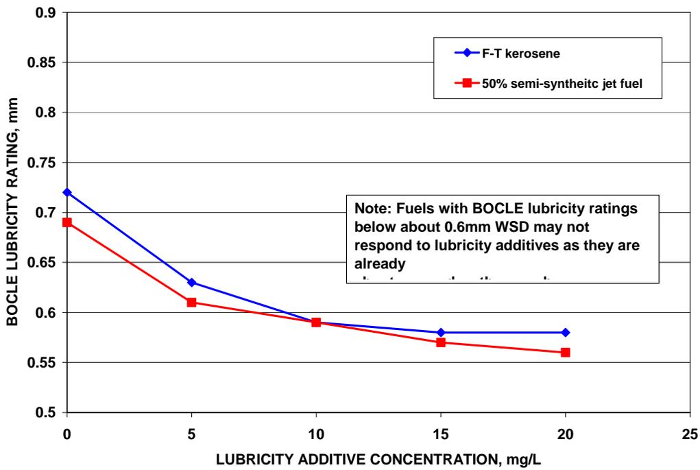
Figure 3. Typical Response to Corrosion Inhibitor/Lubricity Improver (CI/LI) Additive
