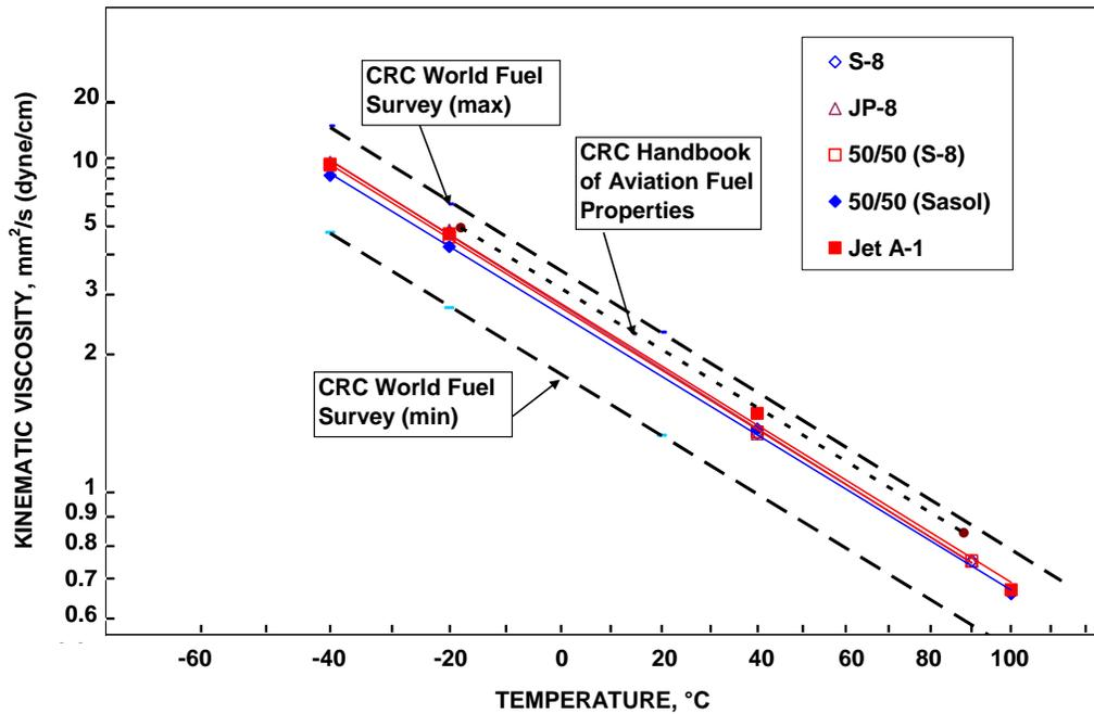
**Figure 12. Comparison of Viscosity**
