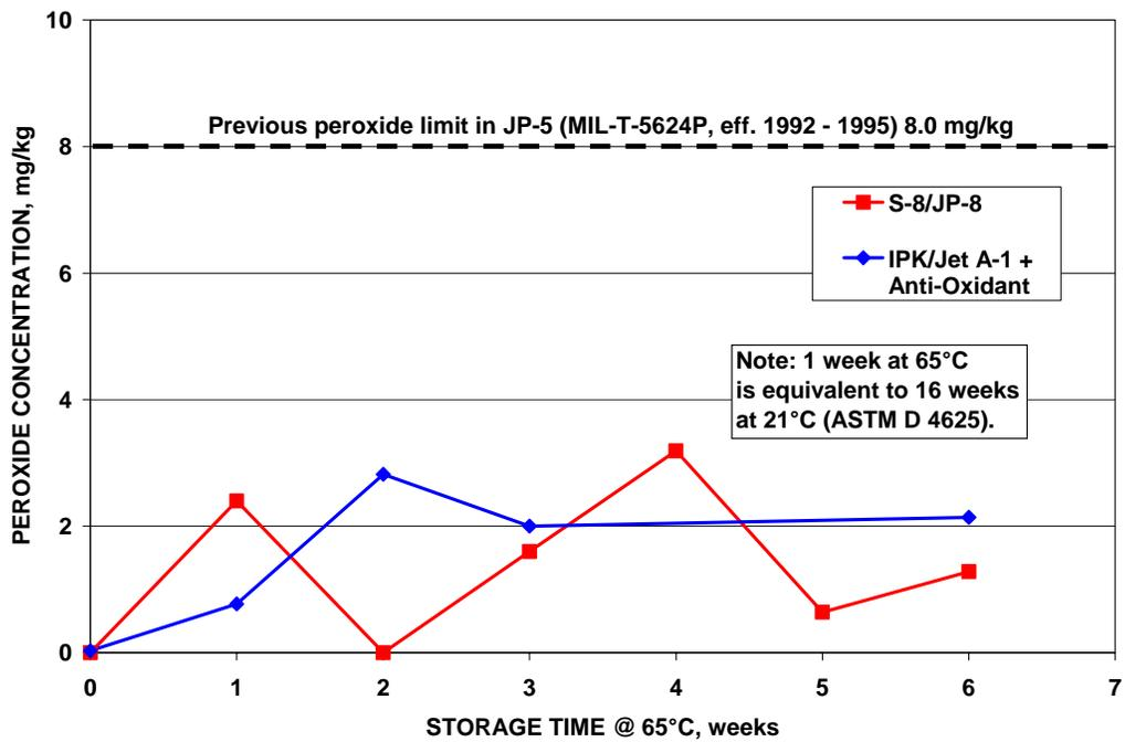
Figure 20. Peroxide Formation During Accelerated Storage (ASTM D 3703)
