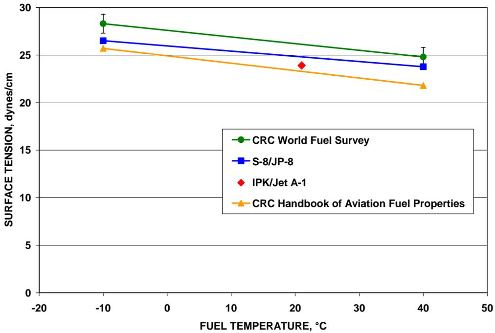
Figure 16. Comparison of Surface Tension
