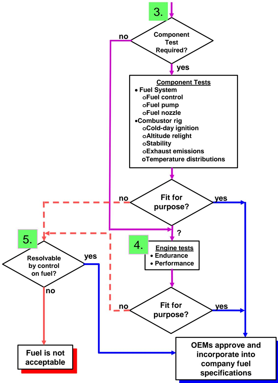
Figure 1b. Approval Process for F-T Kerosenes as Jet Fuel
