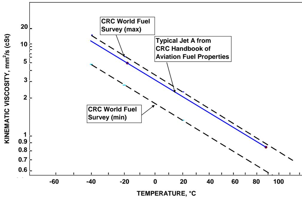
Figure 2. Typical Viscosity Characteristics of Jet Fuel
