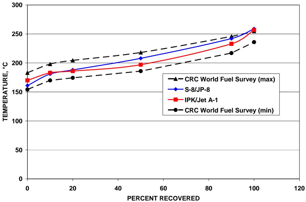
Figure 18. Comparison of Boiling Point Distribution (ASTM D 86)
