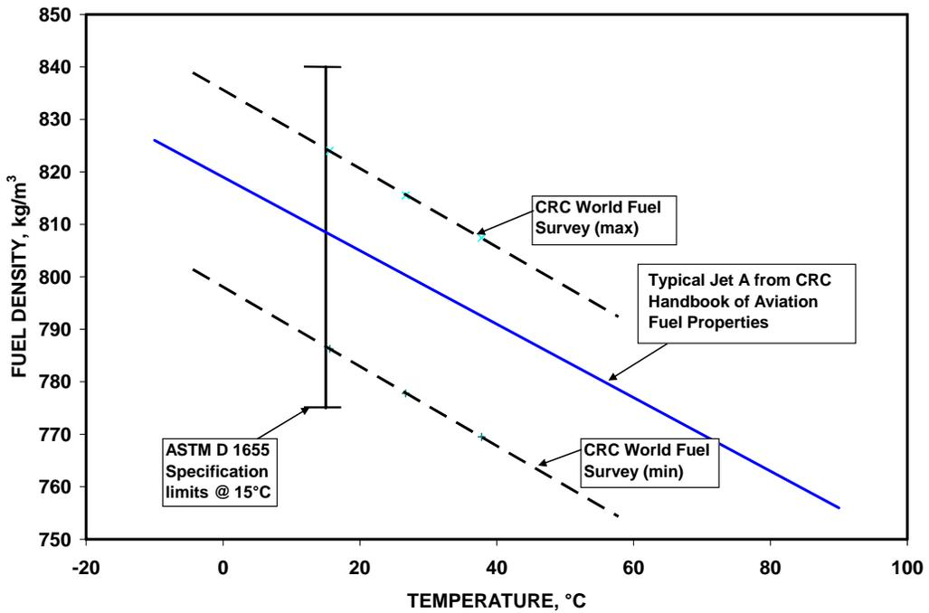
Figure 5. Typical Density Characteristics of Jet Fuel
