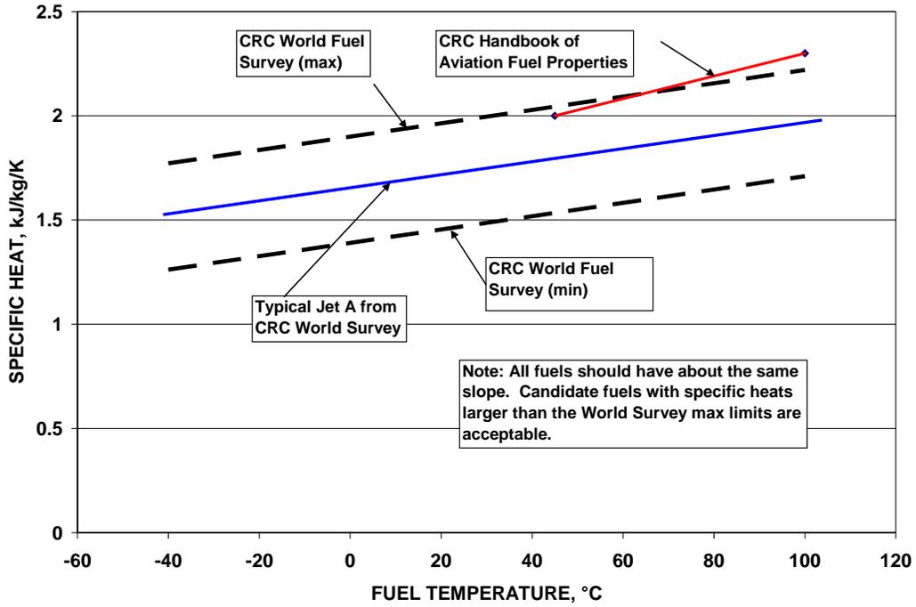
Figure 4. Typical Specific Heat Characteristics of Jet Fuel
