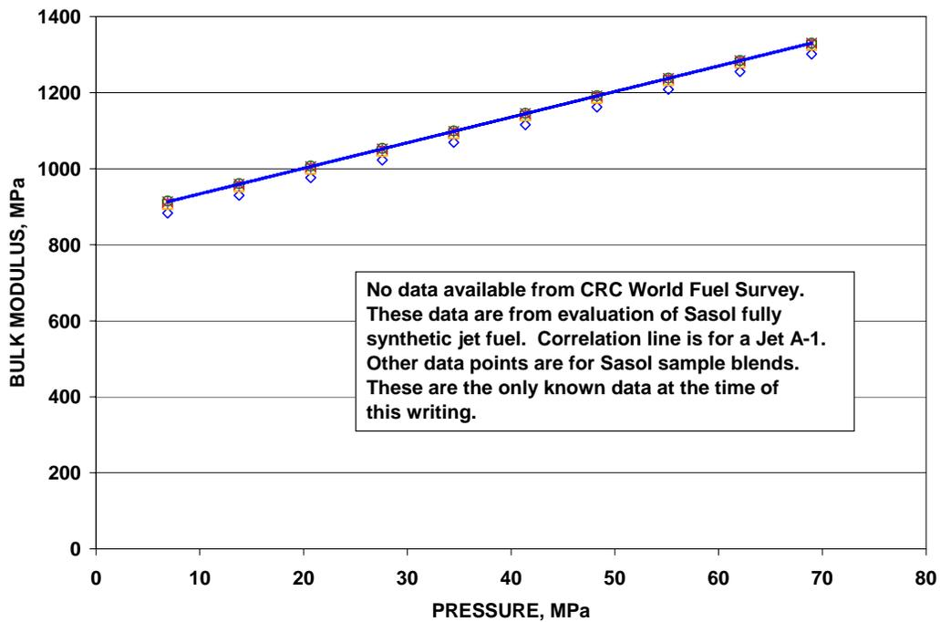
Figure 7. Bulk Modulus Characteristics
