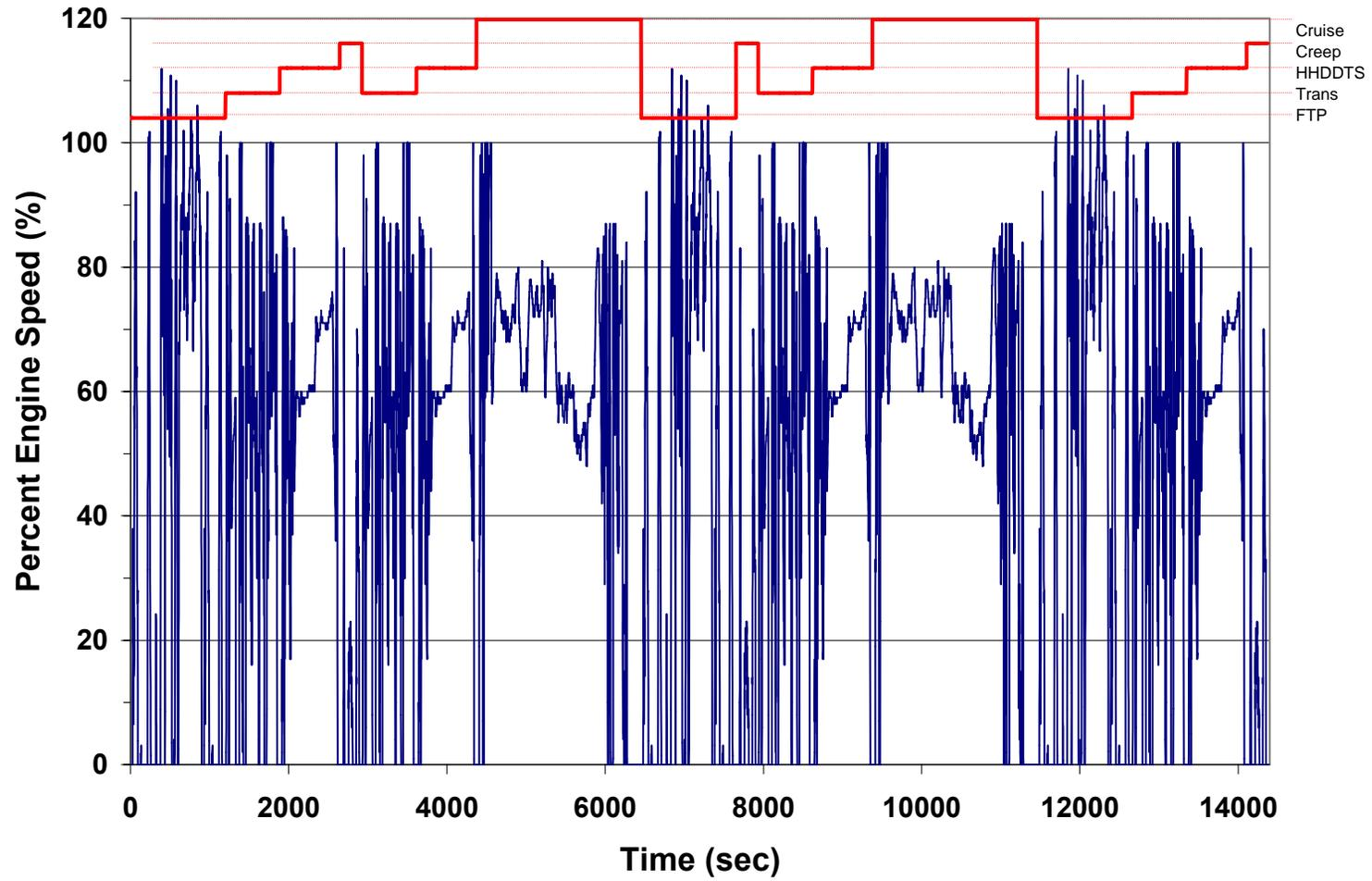
Figure 2: Engine Speed for 4-hour Sub-Cycle
