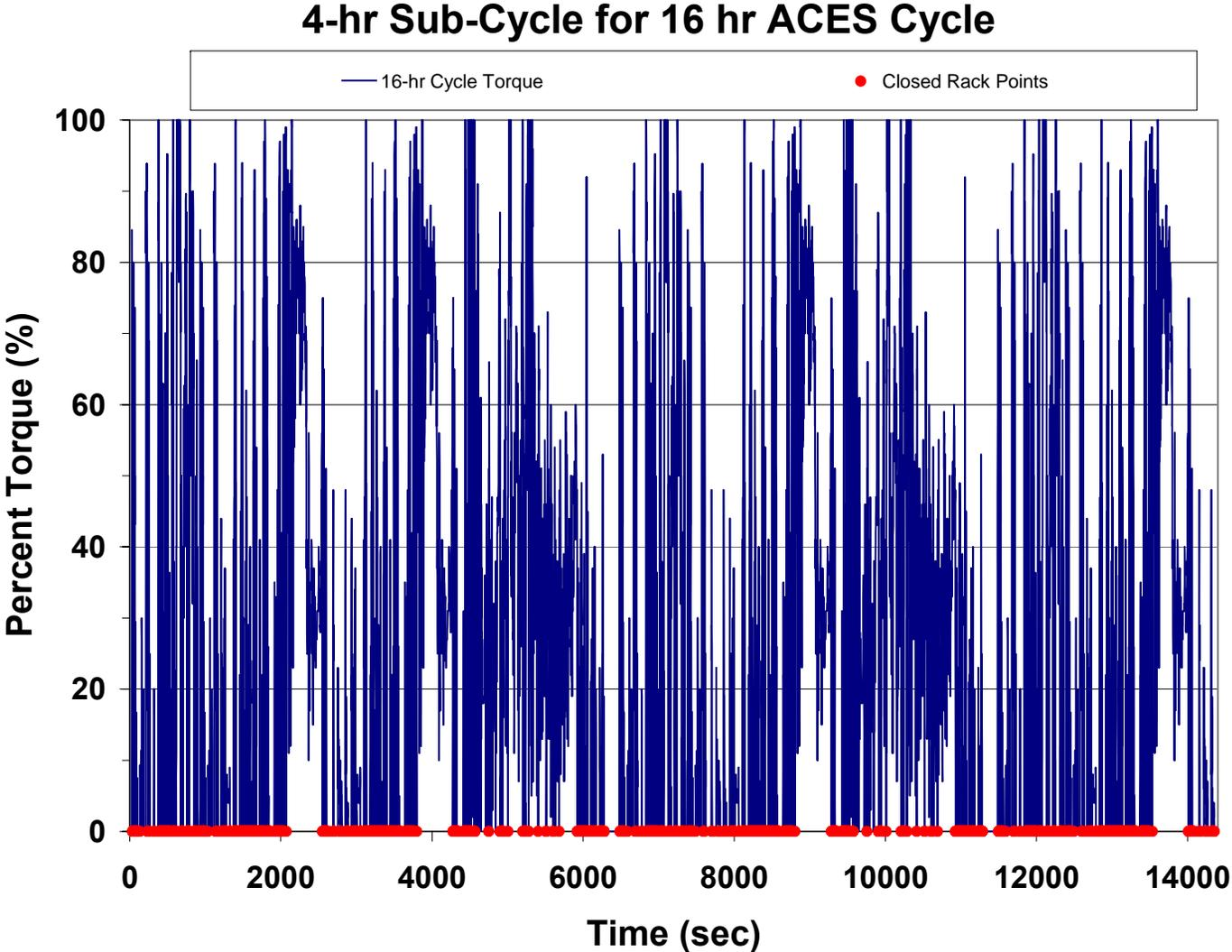
Figure 3: Engine Torque for 4-hour Sub-Cycle
