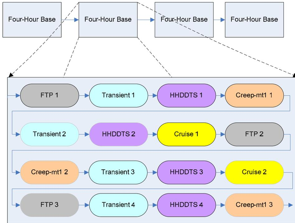
**Figure 1: 16-hour Test Sequence**
