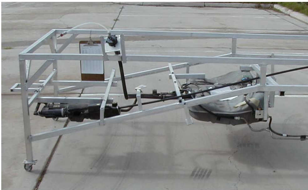
Figure 5 - Rig 11 Fuel Tank and Canister
