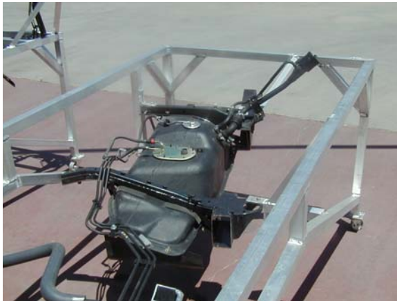
Figure 3 - Rig 1 Fuel Tank
