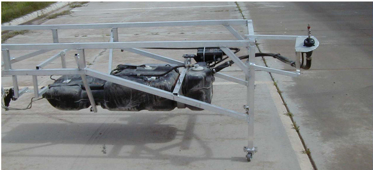
Figure 8 - Rig 14 Fuel Tank and Canister
