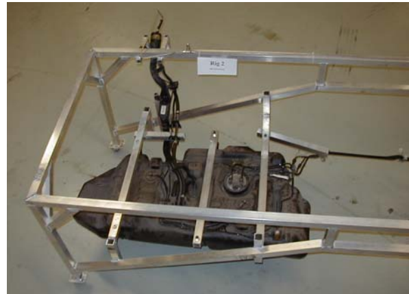
Figure 4 - Rig 2 Fuel Tank
