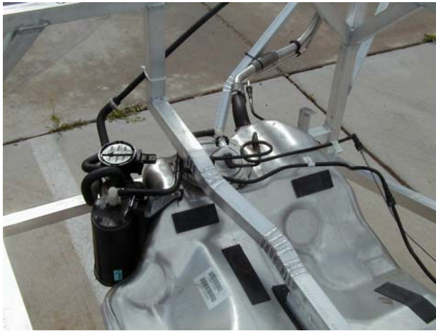
Figure 7 - Rig 12 Fuel Tank and Canister
