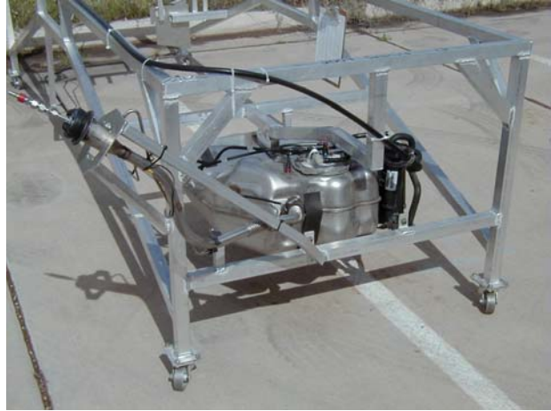
Figure 6 - Rig 12 Fuel Tank
