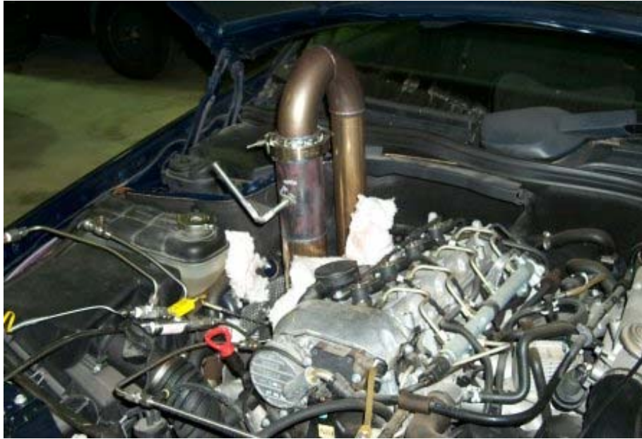
FIGURE 1. SPOOL PIECE INSTALLED ON VEHICLE
