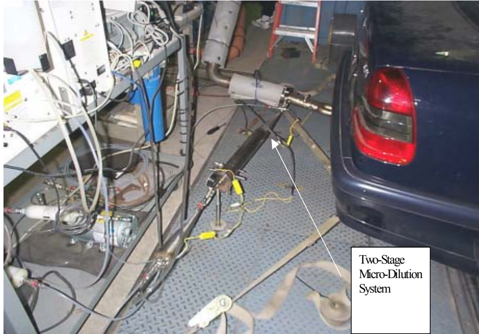
FIGURE 2. PARTICLE SIZE MEASUREMENT SETUP AT THE TAILPIPE
