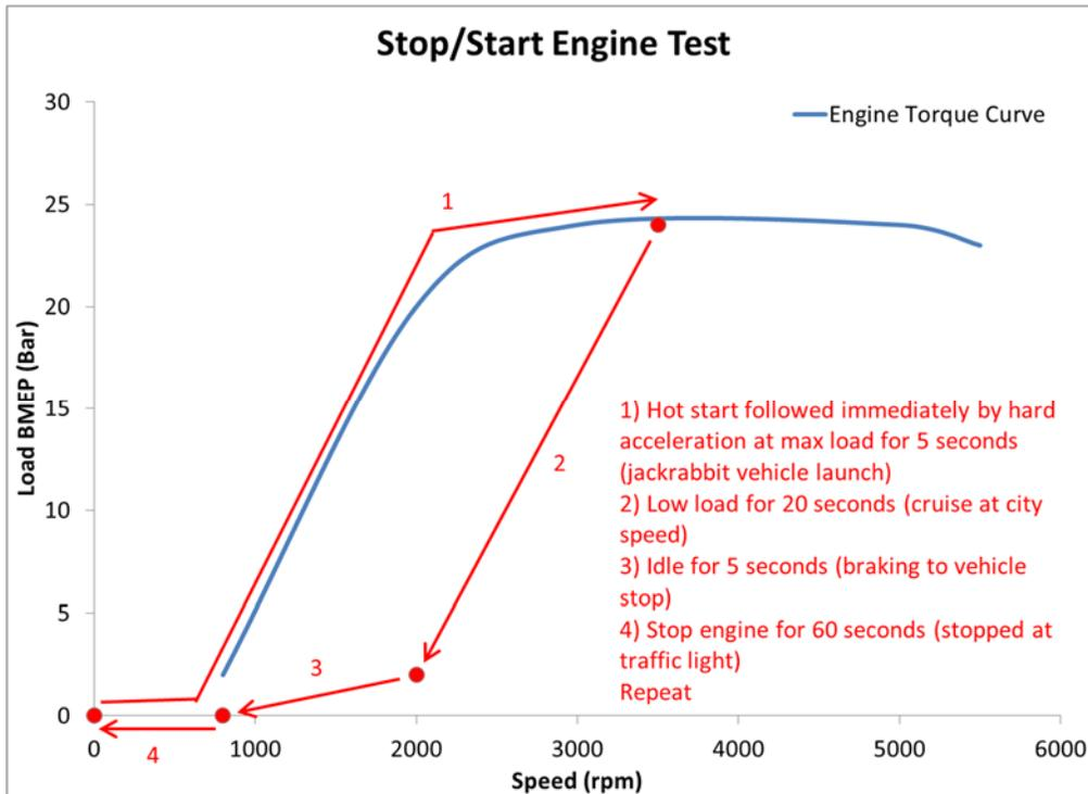
Figure 5. Start/Stop Engine Test
