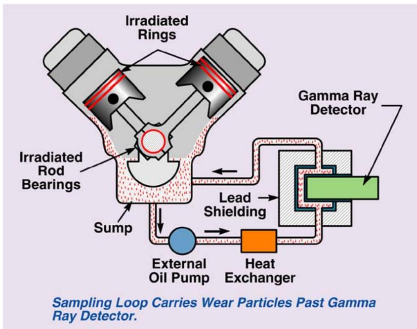
Figure 6. Typical Arrangement for RNT Engine Wear Testing (Figure courtesy of Southwest Research Institute, (3,4))
