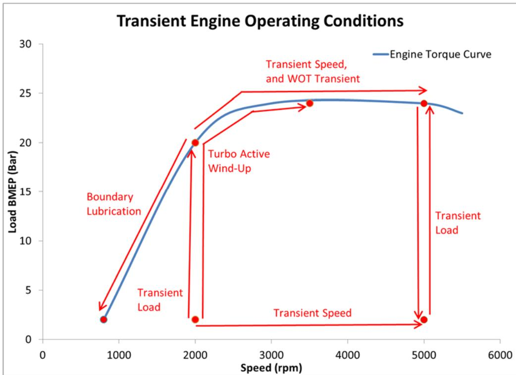
Figure 2. Transient Engine Operating Conditions
