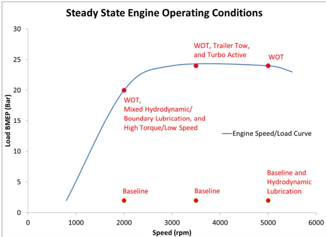
Figure 1. Steady State Engine Operating Conditions
