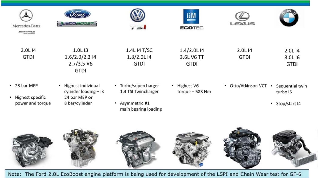
Figure A-1. Candidate Engines and their Characteristics (Courtesy of Bill Woebkenberg, Aramco Services)
