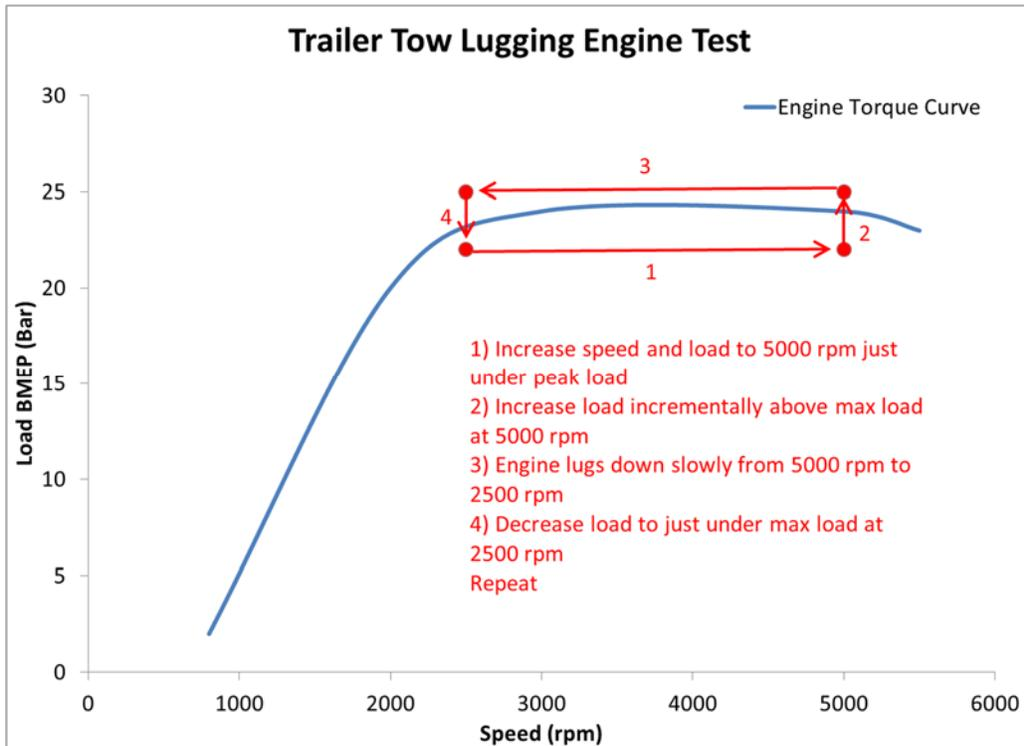
Figure 3. Trailer Tow Lugging Engine Test
