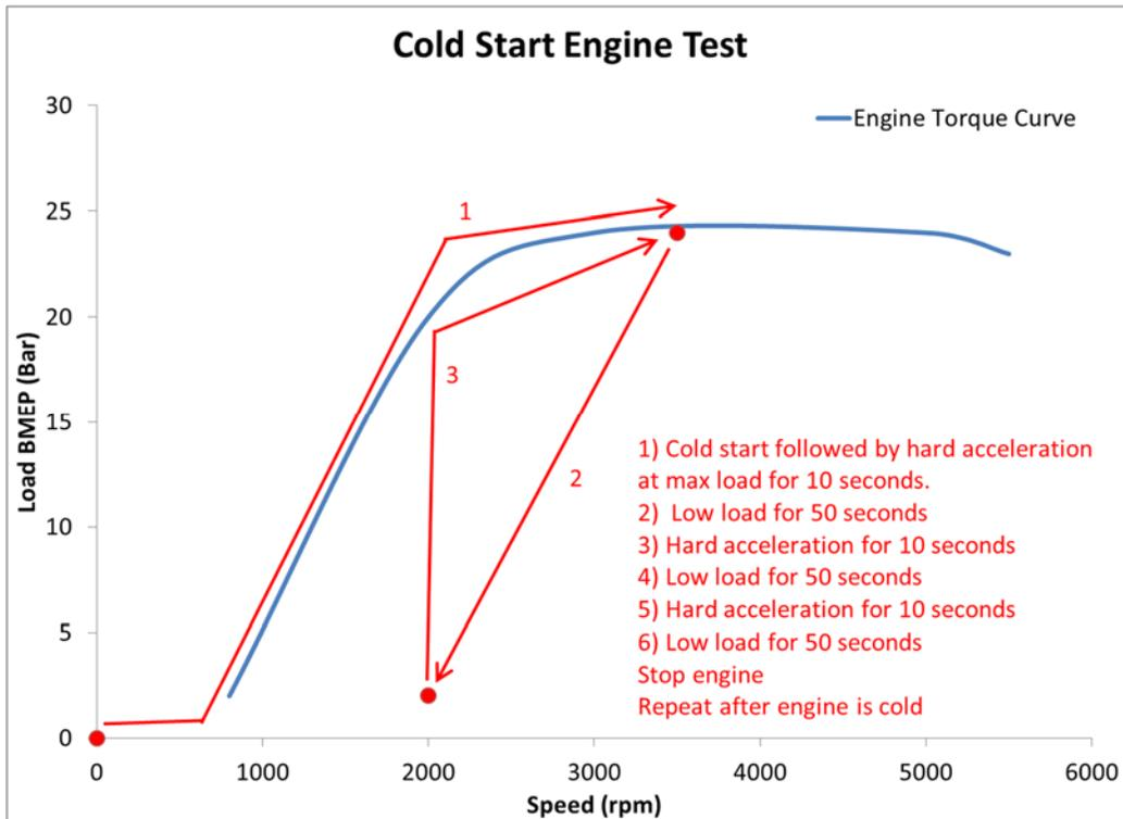
Figure 4. Cold Start Engine Test
