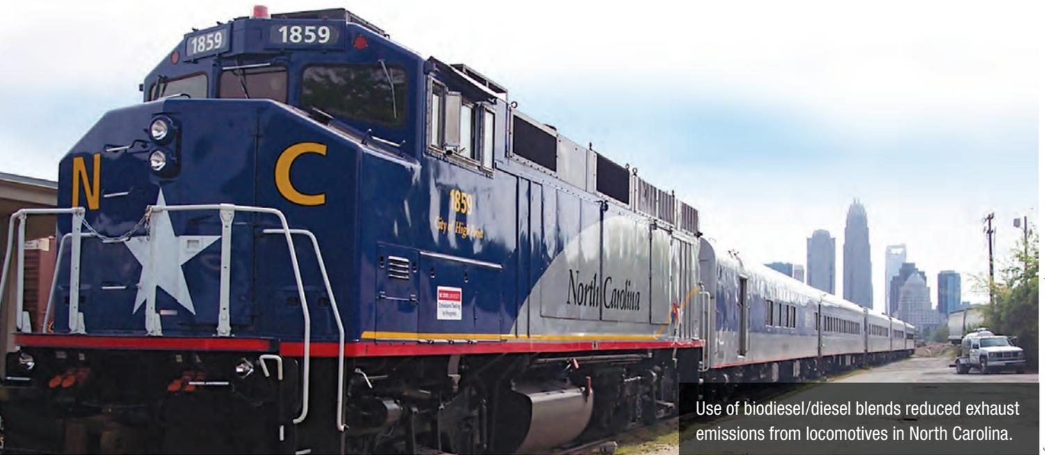
Use of biodiesel/diesel blends reduced exhaust emissions from locomotives in North Carolina.
