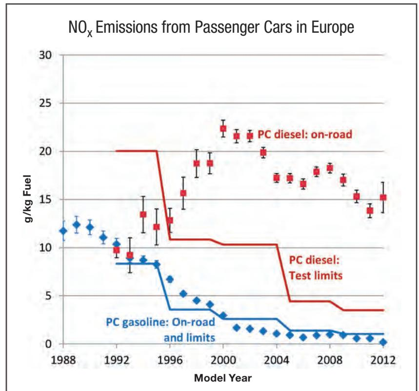
Figure 1.  $\text{NO}_x$  emissions measurements from European gasoline (blue) and diesel (red) cars.
