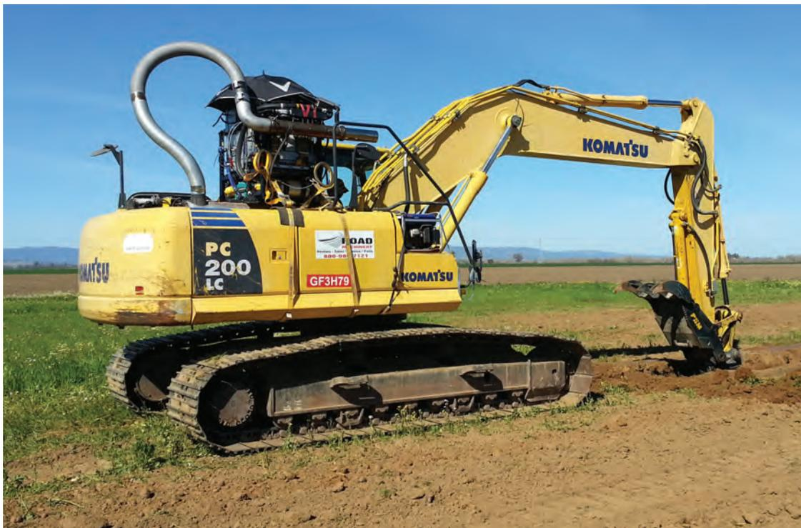
Figure 4. A track excavator outfitted for emissions measurement.
