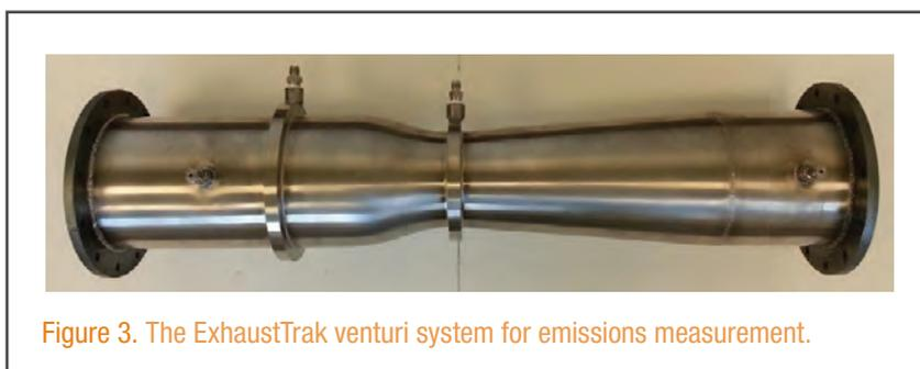
Figure 3. The ExhaustTrak venturi system for emissions measurement.
