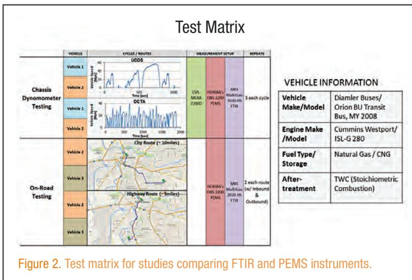
Figure 2. Test matrix for studies comparing FTIR and PEMS instruments.
