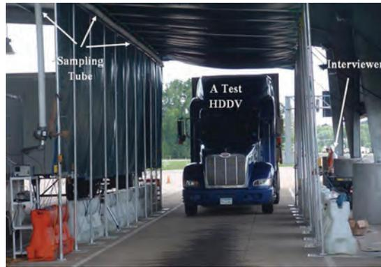
Figure 5. (top) Method for real-time testing of heavy-duty diesel trucks.
