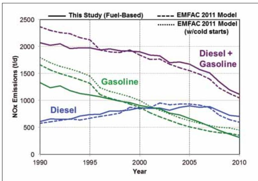
Figure 1. On-road vehicle NO<sub>x</sub> emission trends compared to the EMFAC2011 model for diesel and gasoline.
