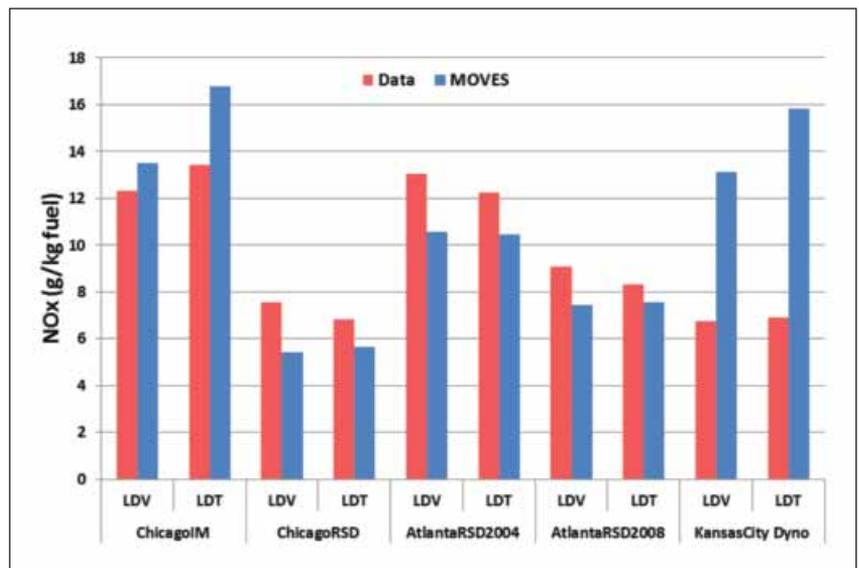
Figure 2. Fleet average NO<sub>x</sub> emission rates for MOVES model vs. emissions data collected from light-duty vehicles in Chicago, Atlanta, and Kansas City.
