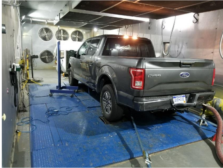
Figure 7. Ford F-150 setup inside climate controlled chassis dynamometer chamber rear view
