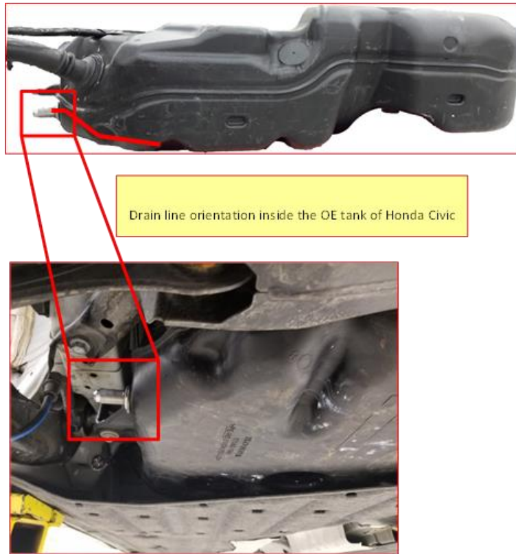
Figure 8. Fuel Tank Drain installation
