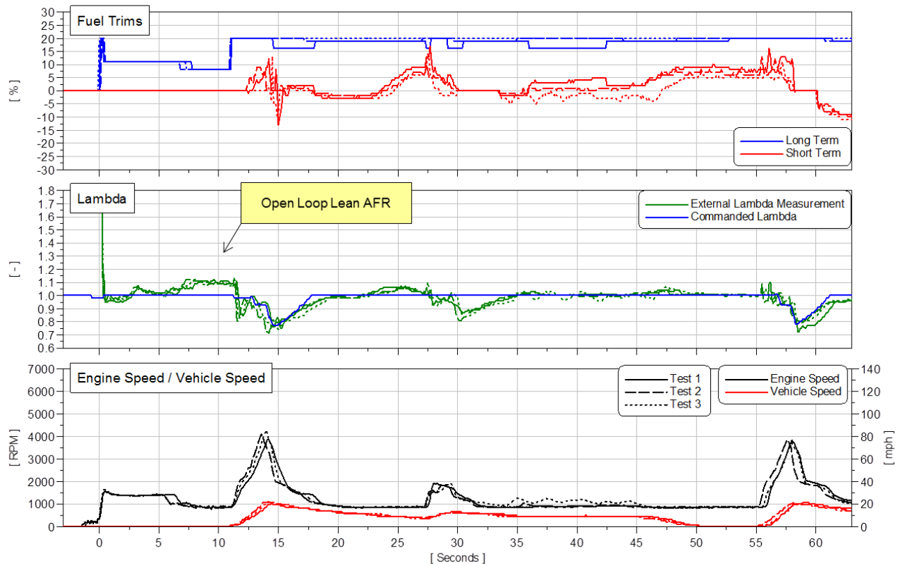
Figure 62. Mazda CX-9 CE30 TR2340A All Tests Open Loop AFR Consistently Lean
